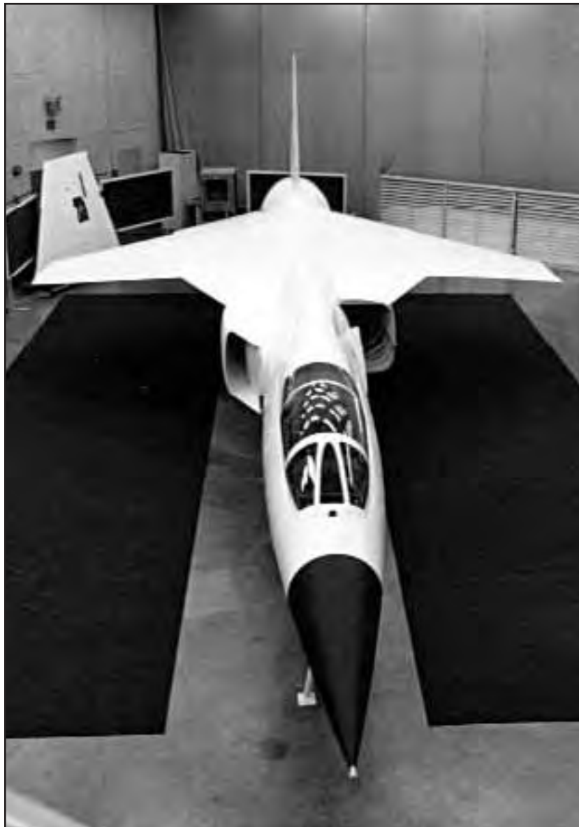
The X-27 was a major modification of the Lockheed F-104 Starfighter designed as an advanced lightweight fighter for foreign sales. The project did not progress beyond the mockup stage when the U.S. Air Force declined to purchase a version of the aircraft. (Lockheed via the Jay Miller Collection)
