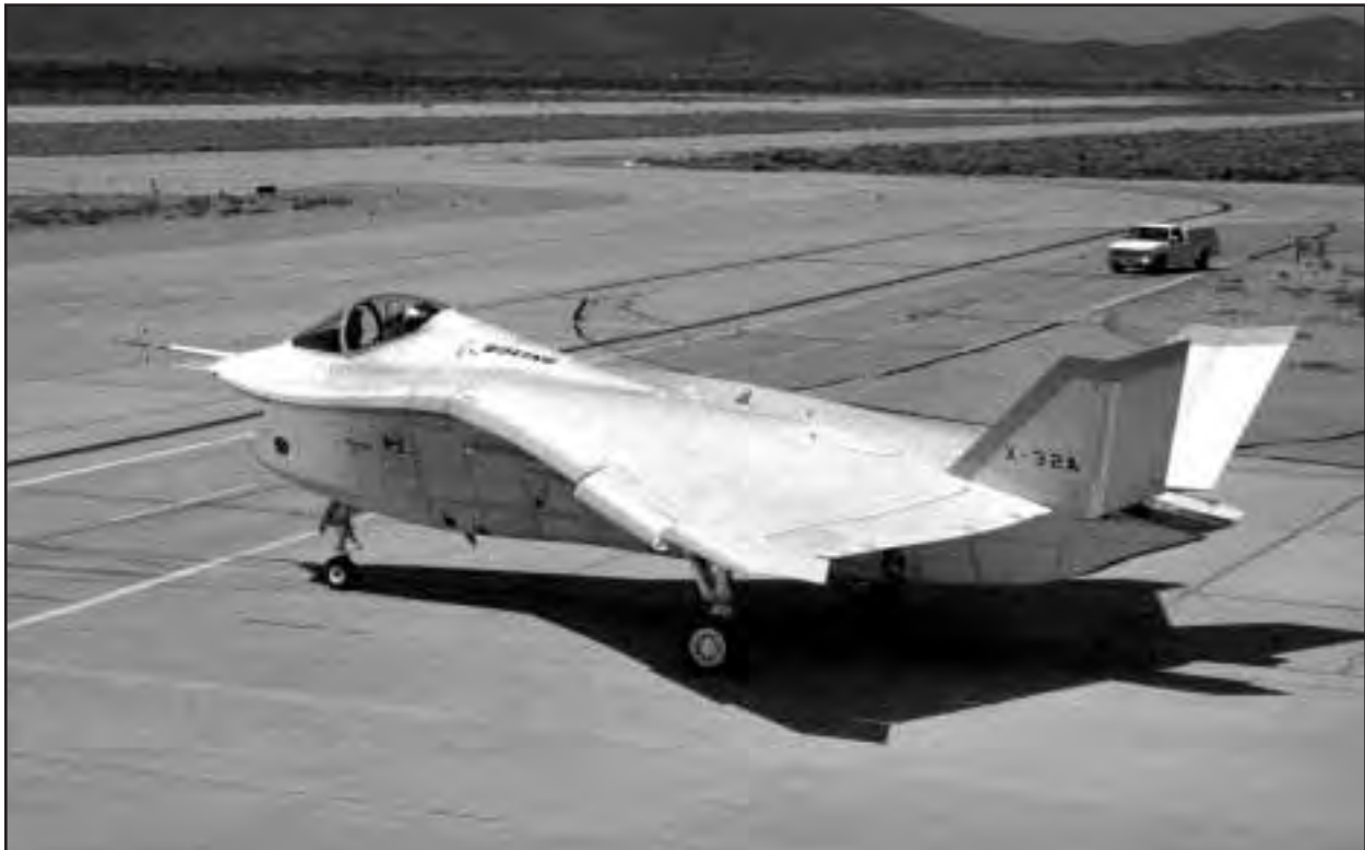
The X-32A completed low- and high-speed taxi tests at Palmdale on 23 May 2000 in preparation for its first flight. (Boeing via the Dennis R. Jenkins Collection)
