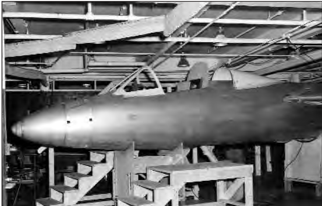
The X-16 was designed as a high-altitude reconnaissance aircraft, but was ultimately cancelled in favor of the Lockheed U-2. A full-scale mockup was completed, but no aircraft were actually built. (Bell Aerospace via the Jay Miller Collection)
