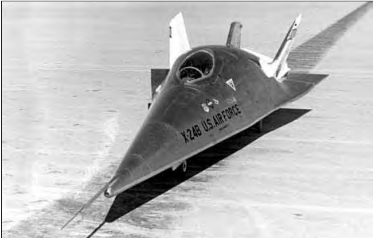
Underneath the sleek skin of the X-24B lurked the original X-24A. The streamlined shape was designed by the Air Force Flight Dynamics Laboratory as the FDL-7/FDL-8. (Martin Marietta via the Jay Miller Collection)
