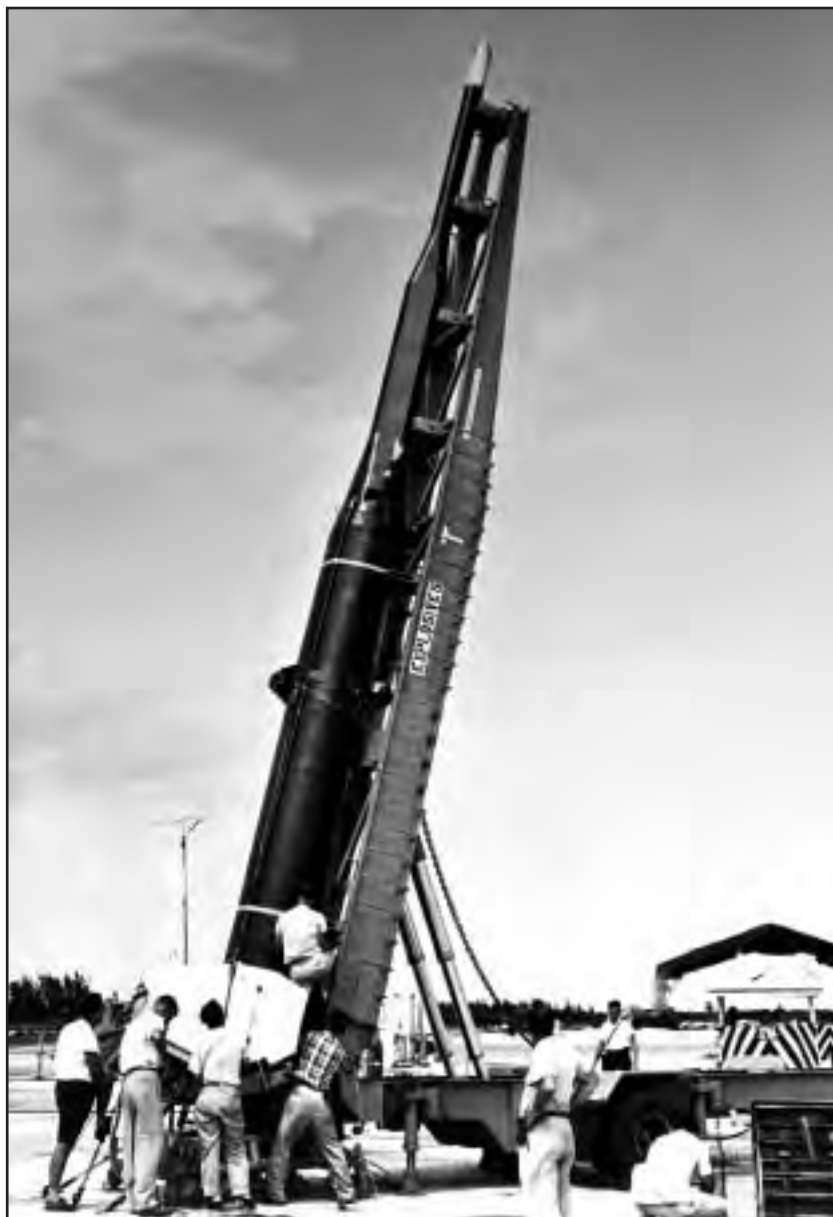
The X-17 used solid rocket motors to carry reentry vehicles to altitude. The original program objectives included reentry speeds of Mach 15 and Reynolds Numbers as high as 24 million. (U.S. Air Force via the Jay Miller Collection)
