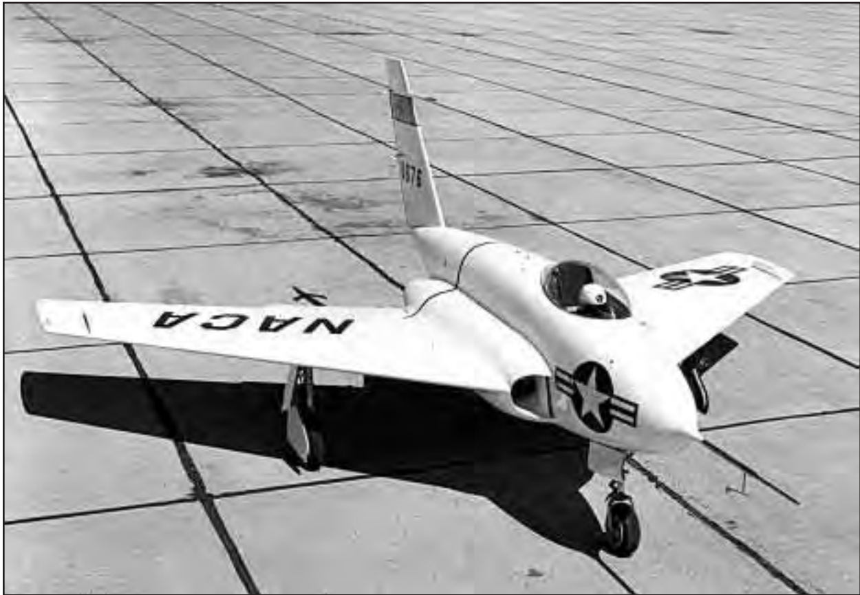
The X-4 was the first U.S. effort to explore the transonic flight characteristics of tailless aircraft. The aircraft exhibited considerable pitch, roll, and yaw instabilities at approximately Mach 0.88. (Gerald Balzer Collection)
