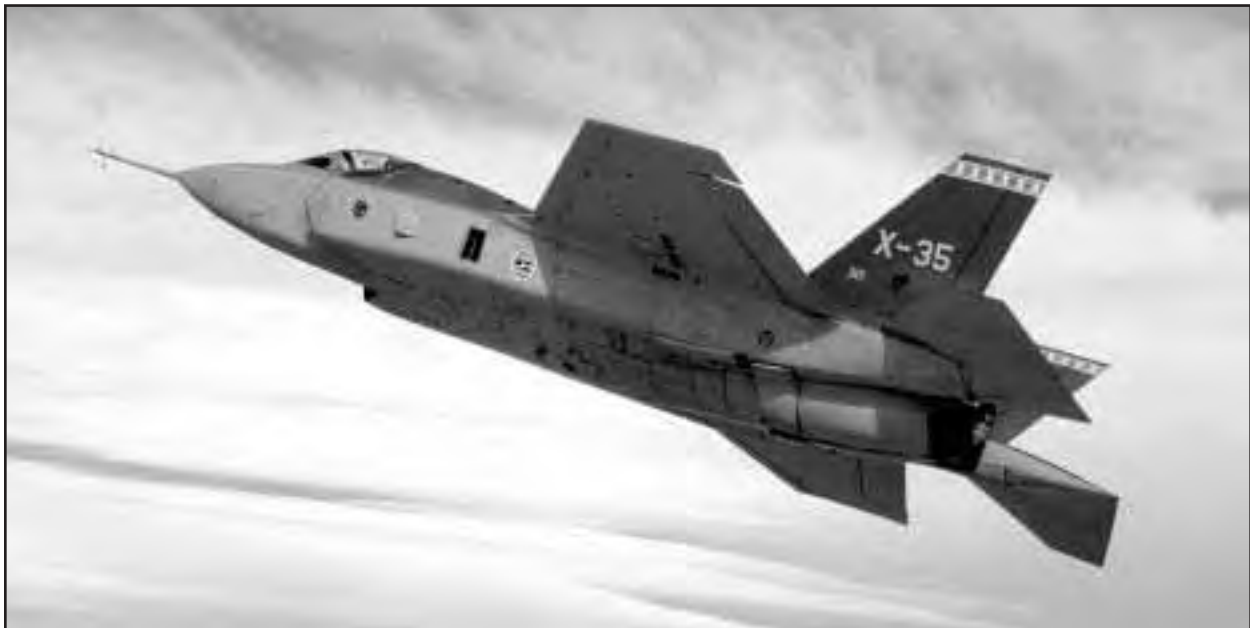
The first of the X-35 demonstrators. Despite being completely different, there is a strong family resemblance to the Lockheed F/A-22 Raptor. (Lockheed Martin via the Tony Landis Collection)
