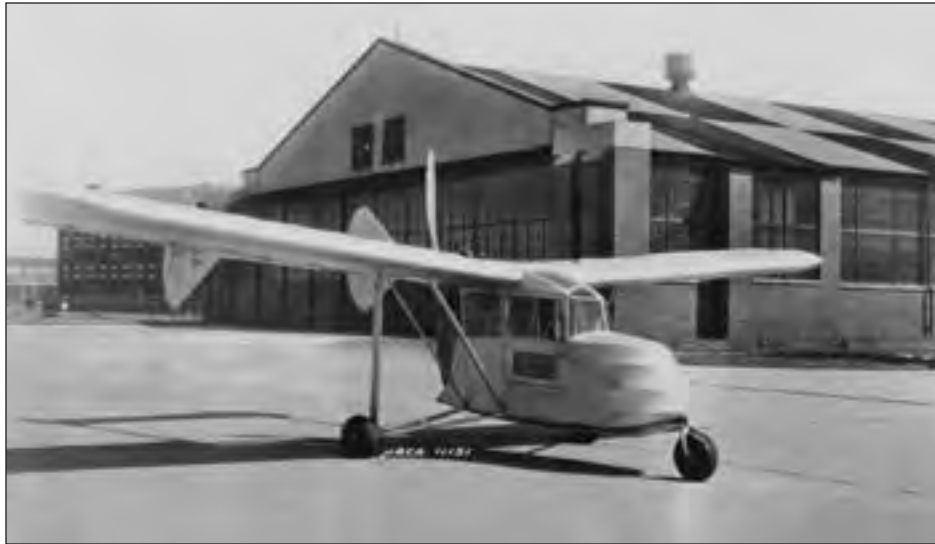
Fred E. Weick's W-1 home-built experimental airplane with steerable, tricycle gear precipitated a major change in how engineers designed modern aircraft. (NASA Image No. L-11151)
