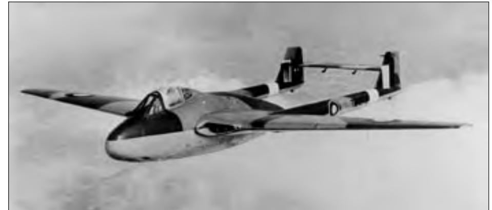
In the early 1950s the British conducted a wide-ranging program of laminar-flow control (LFC) research using three De Havilland Vampire jet fighters. The De Havilland Vampire was Great Britain's second jet fighter of World War II, first flown in 1943. Powered by Rolls Royce engines, it could fly at 540 miles per hour, about 100 mph faster than the Spitfire. National Air and Space Museum, Smithsonian Institution (SI 2001-1109)
