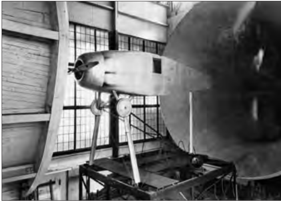
The inclusion of NACA Cowling No. 10, seen here undergoing tests in the 20-foot tunnel in September 1928, into the design of the Martin B-10 bomber increased the airplane's maximum speed by 30 mph to 225 mph and reduced its landing speed significantly. (NASA Image No. 1974-L-02730)
