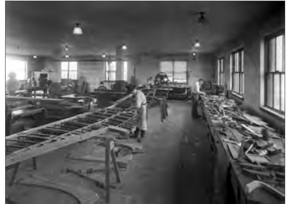
Workmen in the patternmakers' shop at NACA Langley manufacture a wing skeleton for a Thomas-Morse MB-3 airplane for pressure distribution studies in flight, June 1922. The MB-3's wing employed a Royal Air Force 15 airfoil. NASA Image #L-00184 (LaRC)
