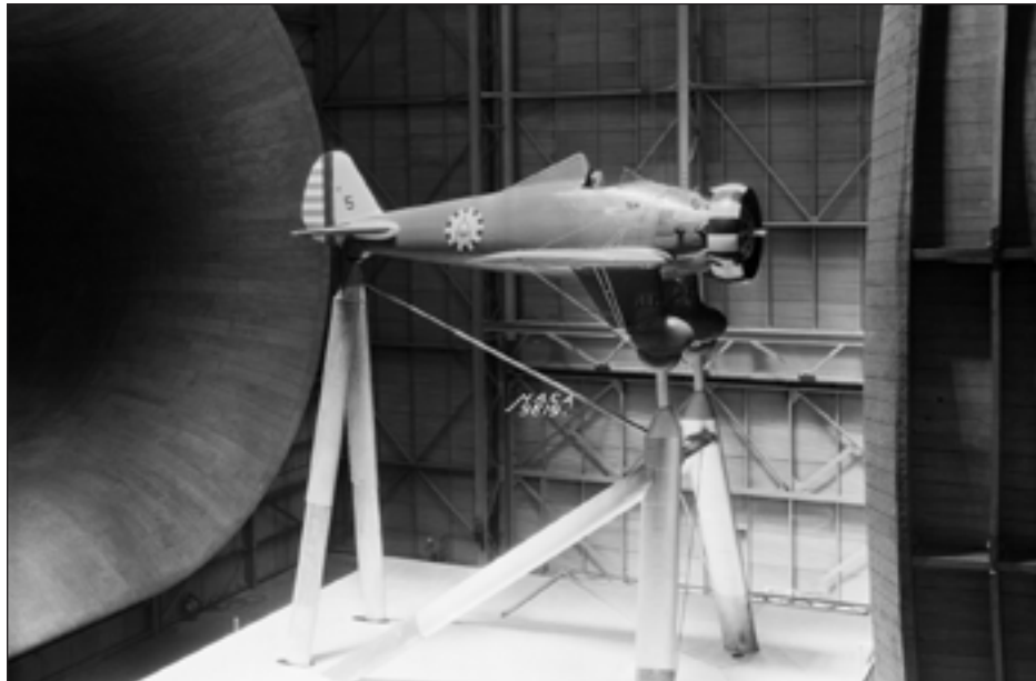
The alternative to the NACA cowling was the Townend ring, seen here mounted on a Boeing P-26 Peashooter perched in the Langley Full-Scale Tunnel for aerodynamic testing. (NASA Image No. L-09819)
