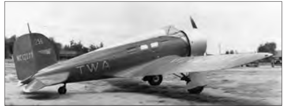
The highly successful Lockheed Orion utilized retractable landing gear and an aerodynamically refined shape to generate unprecedented overall performance. Nevertheless, its wooden construction and lack of a high-lift flap system and a variable-pitch propeller kept it from being a truly revolutionary airplane. (SI Negative No. 1996-0012; Videodisc No. 1B-14112)
