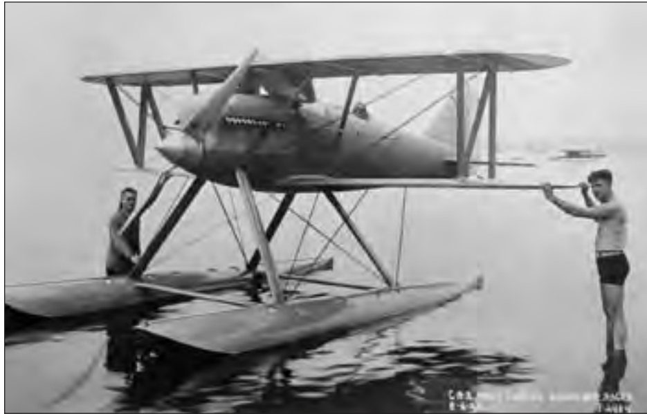
The streamlined fuselage, flush wing radiators, and solid aluminum alloy Reed propeller of the navy Curtiss CR-3 racer highlighted the role of aerodynamics in high-speed aircraft design. Lt. David Rittenhouse (in cockpit) flew the CR-3 to victory in the 1923 Schneider Cup international seaplane race in Cowes, England. (SI Negative No. A-47217)
