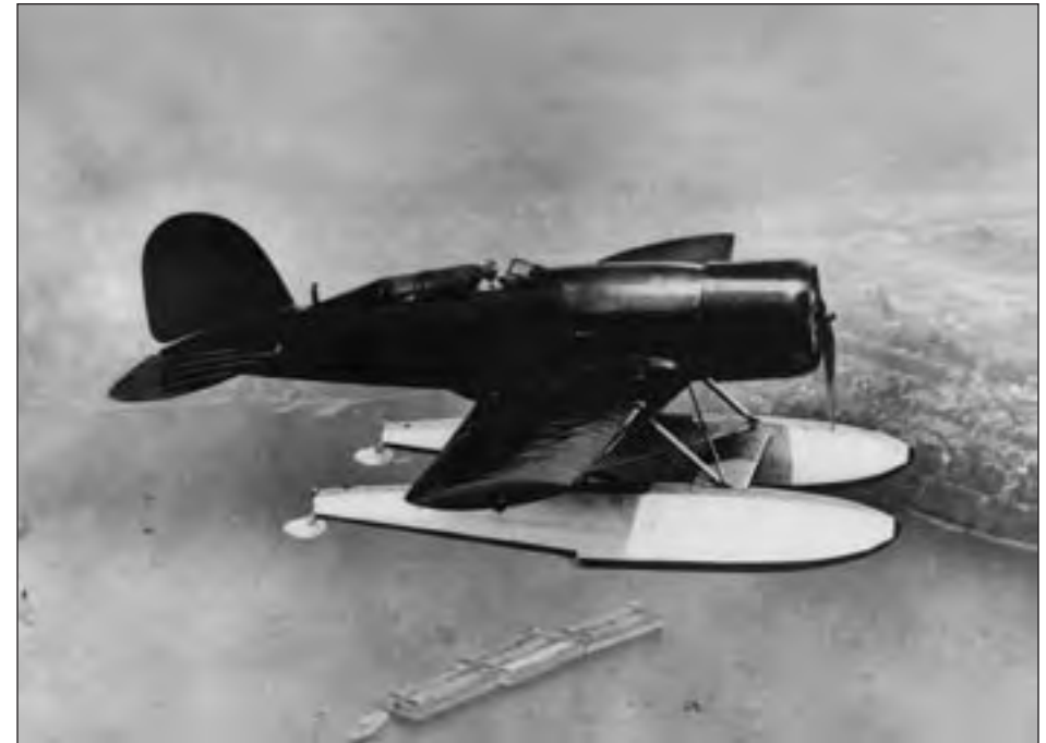
Aircraft such as the Lockheed Sirius “Tingmissartok” flown by Charles and Anne Lindbergh represented the transitional nature of aerodynamic design with its advanced streamline shape combined with an open cockpit, ground-adjustable pitch propeller, and large floats. (SI Negative No. A-5172)
