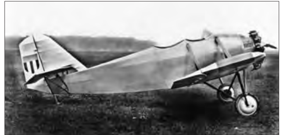
NACA engineers found that with the later addition of wing fillets and a NACA cowling, the diminutive McDonnell Doodlebug experienced greatly reduced buffeting and aerodynamic interference. (SI Negative No. A43437-C)
