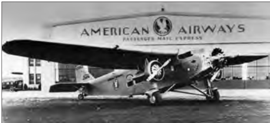
The Ford Trimotor 5-AT-B was a “mainstay design” for America’s growing commercial airline industry, but its improperly placed engine nacelles below the wing, angular windscreen, exposed engines, ground-adjustable pitch propellers, fixed landing gear, and corrugated aluminum construction did not reflect the rapid advances in aerodynamic streamline design. (SI Negative No. 47937-J)
