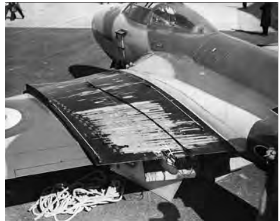
On the wing of the Vampire, researchers experimented with various porous surfaces in hopes of achieving prolonged laminar flow. The British tried a rolled metallic cloth on the wing surface, a technique that did not work, as roughness picked up in the mesh caused a premature transition to turbulent flow. They later used a perforated sheet metal. Eventually, they succeeded in providing a very smooth surfaces back to 25 percent of the chord. National Air and Space Museum (NASM 1A35429), Smithsonian Institution
