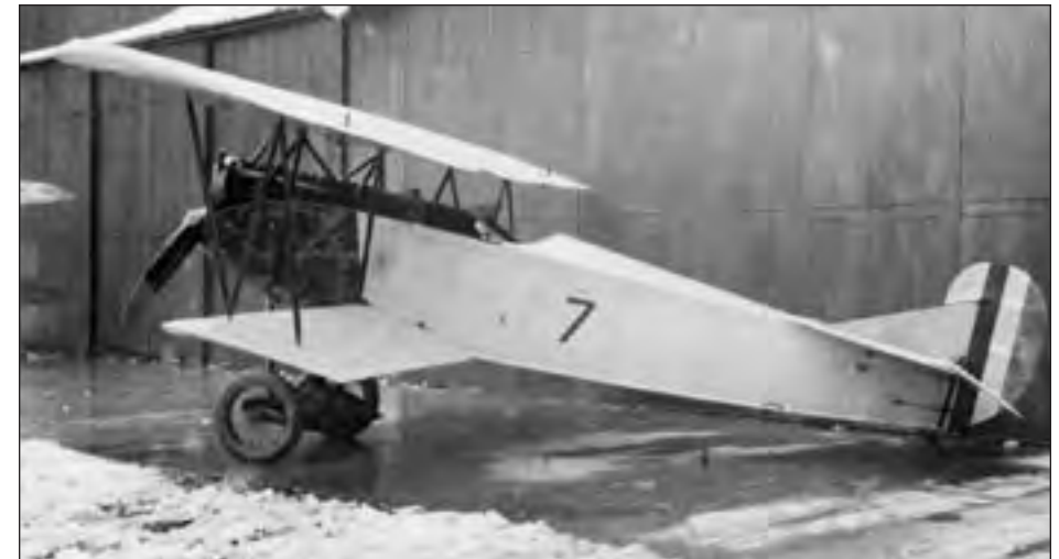
The most advanced feature of the Fokker D-VII airplane of World War I was its internally braced cantilever wings involving very thick airfoil sections. Many of the fine characteristics of this biplane, one of the most renowned of Germany's fighters, were due to its wing thickness, which was unusual for its day. Fokker built the D-VII wing around a Göttingen 418 airfoil. Laurence K. Loftin, Jr, Quest for Performance , p. 34. http://www.hq.nasa.gov/office/pao/History/SP-468/ch2-2.htm
