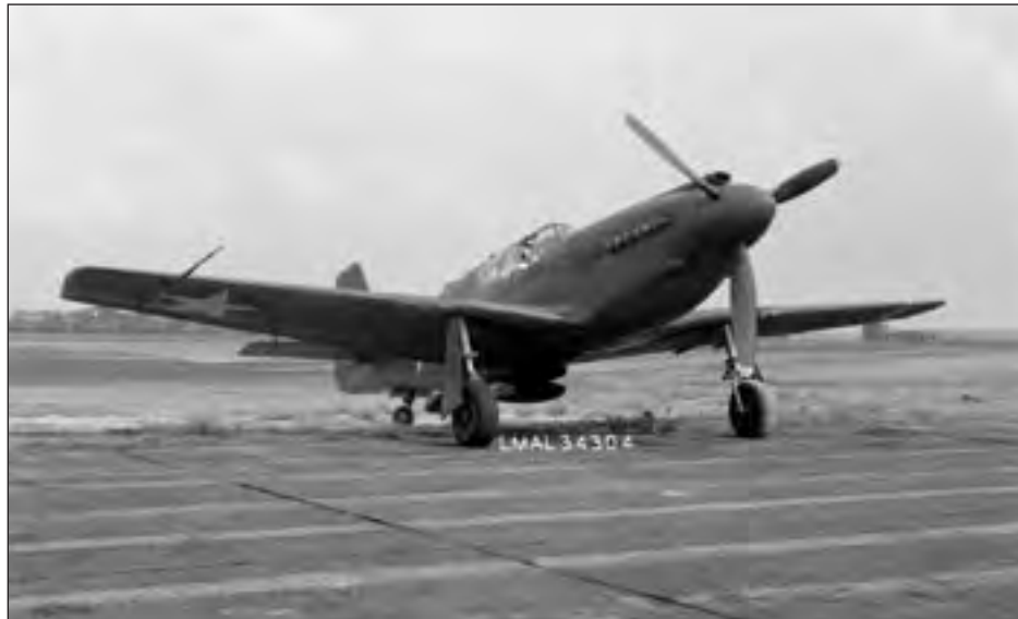
One of the reasons why many experts feel the North American P-51 Mustang represents the highest level of technical achievement ever accomplished in a propeller-driven fighter aircraft is its highly effective low-drag wing. The XP-51 was the first aircraft to incorporate an NACA laminar-flow airfoil. This is the second XP-51, which arrived at Langley in March 1943. NASA Image #L-34304 (LaRC)
