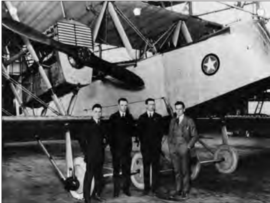
Aircraft such as the biplane, strut-and-wire braced Martin MB-1 Bomber represented the state of the art in aerodynamic design circa 1917. The designers of the aircraft, Laurence D. Bell (left), Glenn A. Martin (second from right), Donald W. Douglas (right), and James Kindleberger (not pictured), would use the advances of the design revolution to create vastly different aircraft. (Martin test pilot, Thomas E. Springer, is second from left.) (SI Negative No. 43067)
