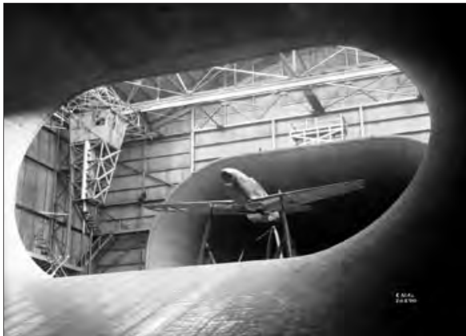
The NACA put the Mustang through systematic drag reduction tests in Langley's Full Scale Tunnel. NASA Image #L-34590 (LaRC)
