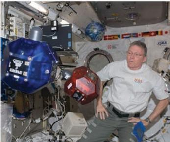
Smart SPHERES intelligent satellites floating free during tests aboard the International Space Station, September 2011.
