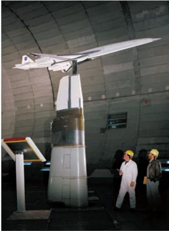
Civil transport model installed in the 40 by 80 foot wind tunnel.
