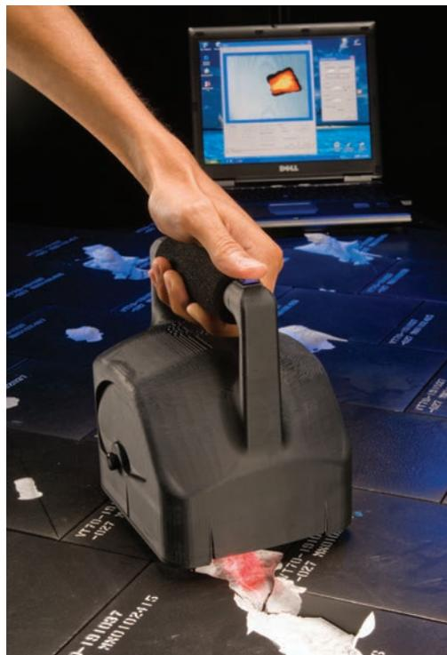
*A wireless scanner for Shuttle orbiter tiles, developed by Joe Lavelle.*
