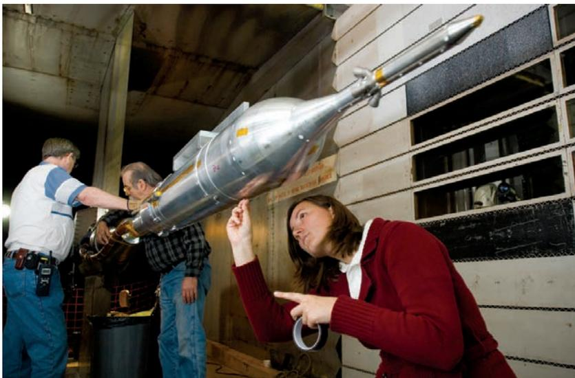
*Crew Lift Vehicle ascent model installed in the 9 by 7 foot wind tunnel*
