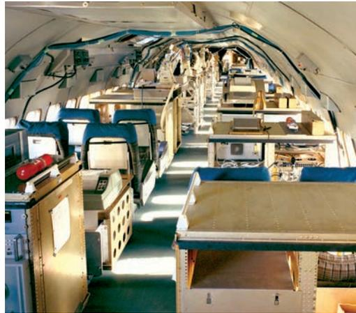
*The interior of the Galileo II in 1972. Ames scientists used this converted Convair 990 as an airborne science platform.*
