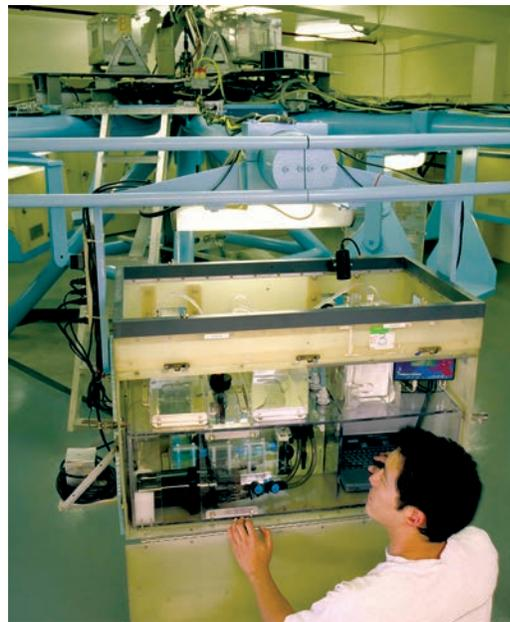
*An experiment package to study zebrafish in microgravity is tested in the Ames aquatic centrifuge.*
