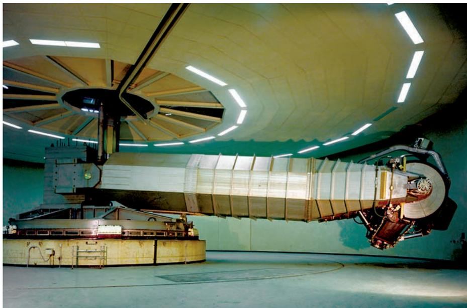
*Flight and guidance centrifuge in 1971 was used for spacecraft mission simulations and research on human response to motion stress.*
