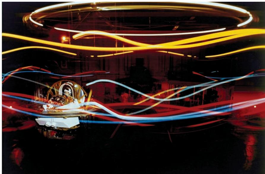
*The 5-degree-of-freedom piloted flight simulator in 1962, also shown in time lapsed exposure to display its wide range of motion.*
