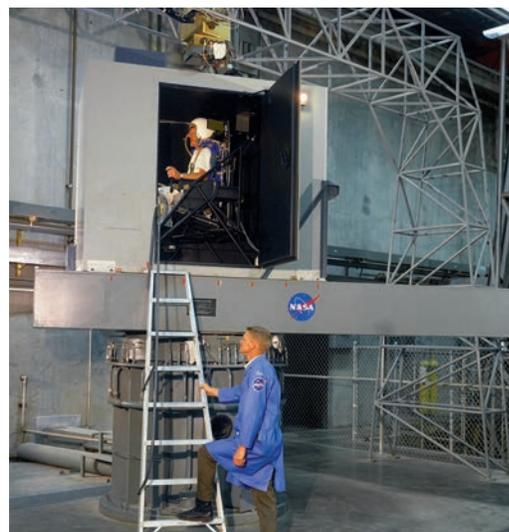
*A human-carrying rotation device opened in 1966 for studies of motion sickness and pilot response to micro-gravity.*
