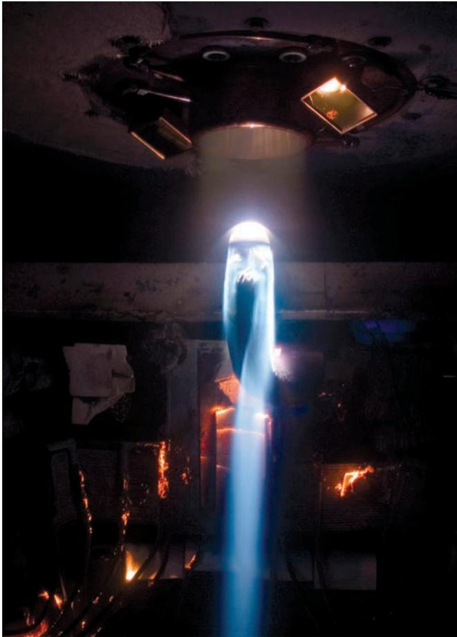
*Arc jet tests of the CEV thermal protection system.*
