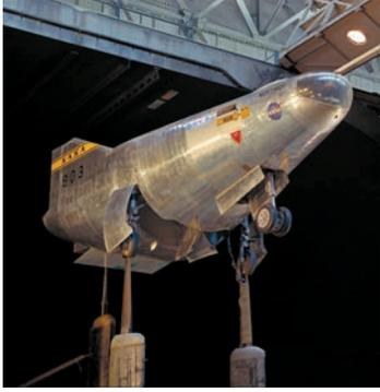
M2-F2 lifting body mounted in the 40 by 80 foot wind tunnel in July 1965 prior to flight tests.
