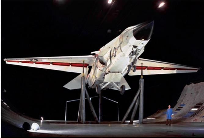
*General Dynamics F-111B aircraft, with its wings fully extended, undergoing tests in the 40 by 80 foot wind tunnel in 1969.*
