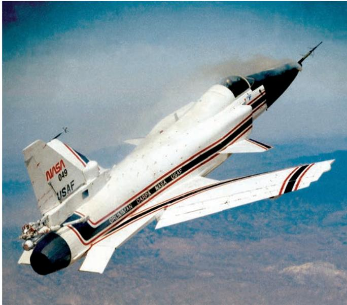
*The X-29 HiMAT in a September 1991 test flight, with smoke blown to demonstrate vortex flow at high angle of attack.*
