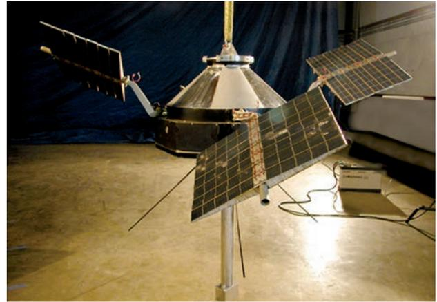
*Explorer 12, a spin-stabilized, solar-cell-powered spacecraft.*
