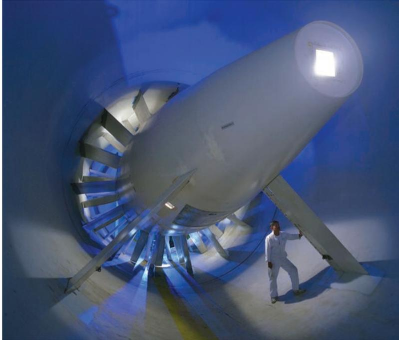
*The 20-blade axial flow fan of the renovated 12 foot pressure tunnel.*
