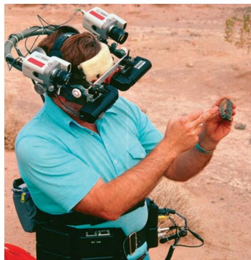
*A 1992 field test of goggles designed for telepresence on Mars.*
