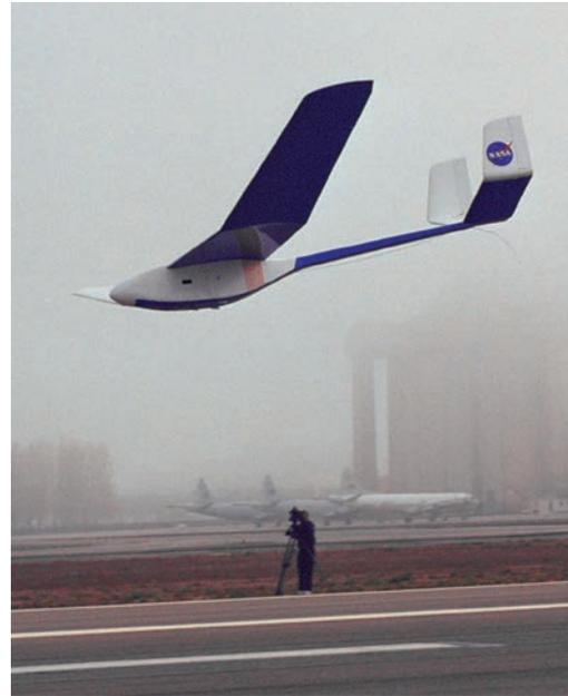
*Another innovative Mars exploration concept, the AME-2, designed to be unfolded and flown through the atmosphere of Mars, in flight tests at Moffett Field.*
