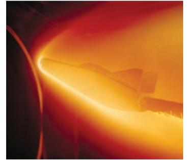
Model of the M2 lifting body, in 1962, in the Ames atmospheric entry simulator, to determine the areas of most intense heating.
