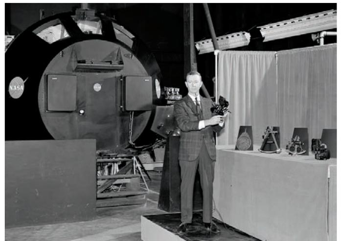
*Ablation test of a Mercury capsule model in an Ames arc jet.*
