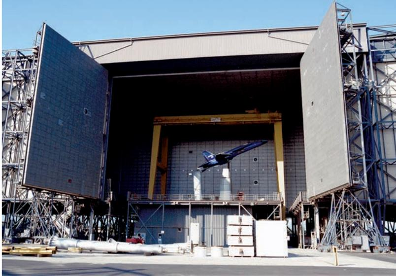
*F-18 installed in the 80 by 120 foot test section for tests at high angles of attack, in September 1993.*
