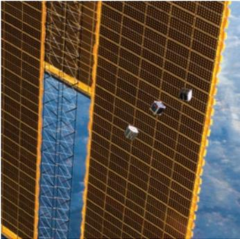
TechEdSat, the left-most object, after being launched from the International Space Station in October 2012. This CubeSat was designed by students at San Jose State University, working in partnership with NASA Ames, to test communications technologies.
