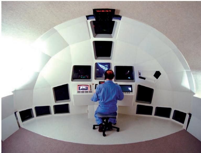
*Space station simulator during research on how best to dock a Shuttle orbiter.*
