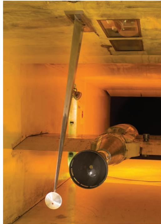
*Test of MSL parachute in the 9 by 7 foot supersonic wind tunnel.*
