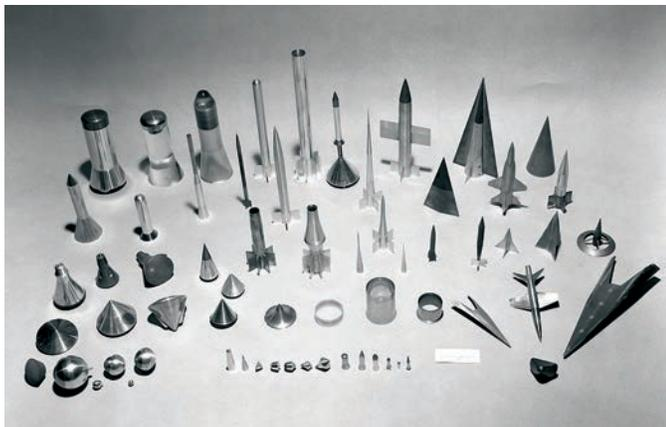
*Models tested in the Ames hypervelocity free flight tunnel.*
