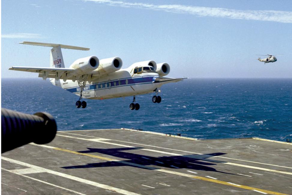
*The quiet short-haul aircraft (QSRA), a highly modified C-8A, undergoing carrier trials on board the USS Kitty Hawk.*
