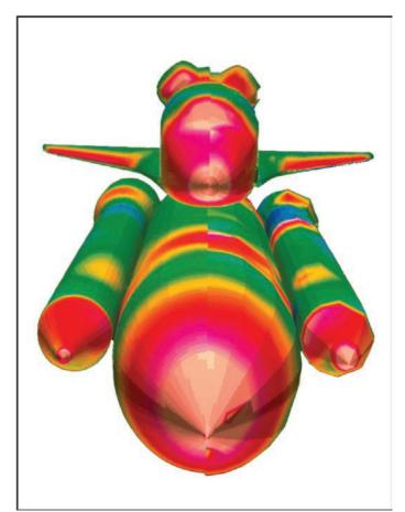
Shuttle in launch configuration showing surface pressure comparisons, 1995. Cetin Kiris created a program called INS3D (an incompressible Navier-Stokes solver in general three-dimensional coordinates). Because it was useful in modelling low-speed, friction-dominated flows, in 1993 the group also applied the code to model air flow over transport aircraft at take-off and to improve a mechanical heart developed at Pennsylvania State University.
