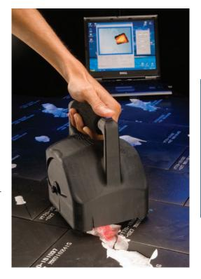
A wireless scanner for Shuttle orbiter tiles, developed by Joe Lavelle.
