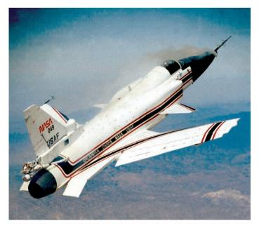
The X-29 HiMAT in a September 1991 test flight, with smoke blown to demonstrate vortex flow at high angle of attack. to the optimum camber and angle, whether at cruise speeds or undergoing heavy loading during maneuvers. Tests of aeroelastic tailoring on the HiMAT provided valuable data on the use of composite materials in all modern aircraft.
