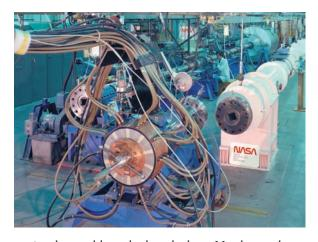
Electric arc shock-tube facility, opened in 1966, was used to study the effects of radiation and ionization during entry into the atmospheres of the outer planets.
