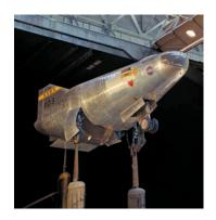
M2-F2 lifting body mounted in the 40 by 80 foot wind tunnel in July 1965 prior to flight tests.
