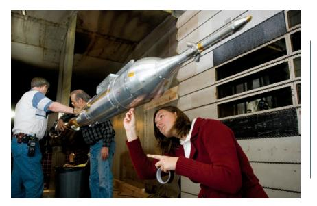
Crew Lift Vehicle ascent model installed in the 9 by 7 foot wind tunnel
