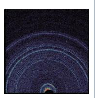
The first X-ray view of Martian soil, taken in October 2012 by the CheMin experiment aboard the Curiosity Rover. Each mineral has a unique pattern of rings.
