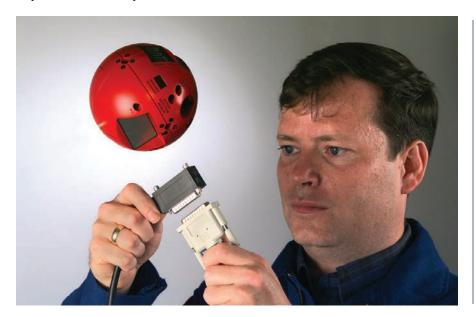
Yuri Gawdiak displays a personal satellite assistant prototyped at Ames in 1999. The PSA hovers behind an astronaut, collects data from onboard experiments, provides video conferencing, and otherwise serves as a wireless link between the astronauts and ground crews.
