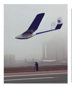
Another innovative Mars exploration concept, the AME-2, designed to be unfolded and flown through the atmosphere of Mars, in flight tests at Moffett Field.
