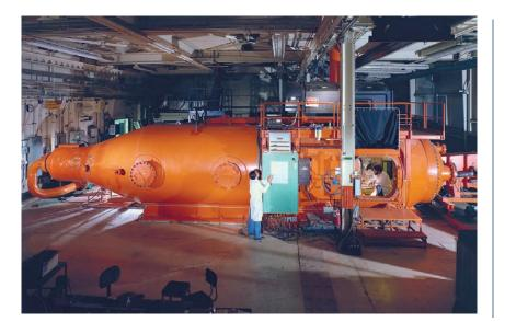
This high Reynolds number channel was opened in 1980 to complement a channel opened in 1973. Aerodynamicists used it for experimental support to verify computational fluid dynamics codes and for very precise studies of two-dimensional airflows.
