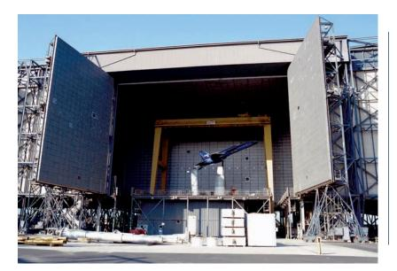
F-18 installed in the 80 by 120 foot test section for tests at high angles of attack, in September 1993.
