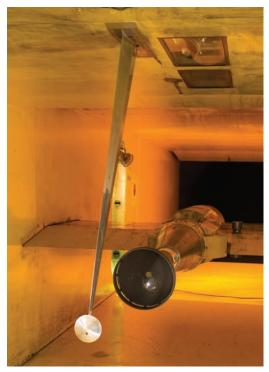
Test of MSL parachute in the 9 by 7 foot supersonic wind tunnel.
