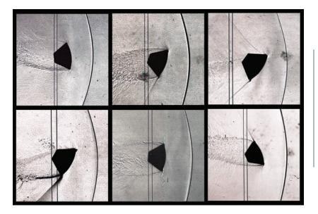
Images of the CEV in aerodynamic stability tests.
