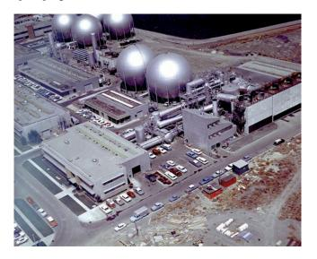
While the HFF generated an enthalpy of 30,000 Btu per pound, the peak heating lasted mere milliseconds. These tunnels worked well for studying reentry aerodynamics, but the heating time was of little use for testing ablative materials. Ablative materials include ceramics, quartz, teflon, or graphite composites that slowly melted The test section of the 60 megawatt aerodynamic heating facility from the outside, and from within.
