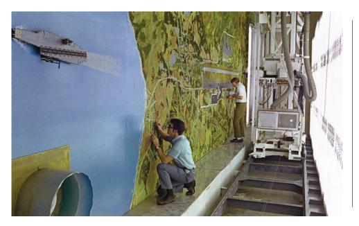
A terrain model, installed at Ames in 1971. A video camera overflew it to generate visual clues for pilots in a remote cockpit simulator.
