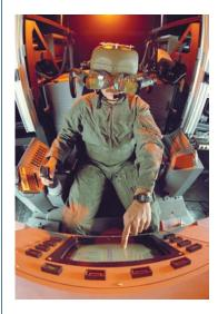
Early tests of a helmet mounted display for a helicopter pilot, 1988.
