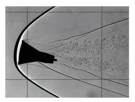
Shadowgraph of the Mercury capsule in a free flight study of aerodynamic stability.
