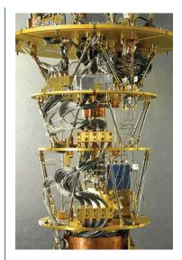
The support structure for the D-Wave Vesuvius processor, the heart of the revolutionary quantum computer installed at the NASA Ames quantum artificial intelligence laboratory, 2013.
