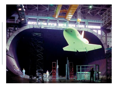
Shuttle Orbiter model in the 40 by 80 foot wind tunnel.
