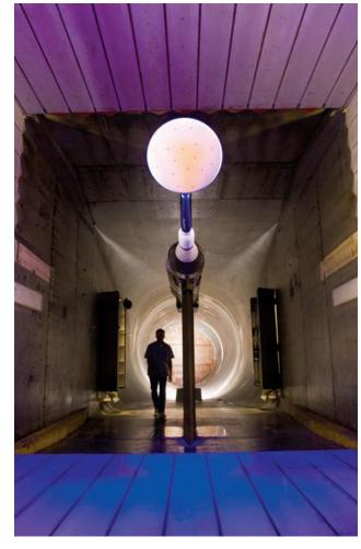
CEV with launch abort system being tested in the Ames 9 by 7 foot supersonic wind tunnel.
