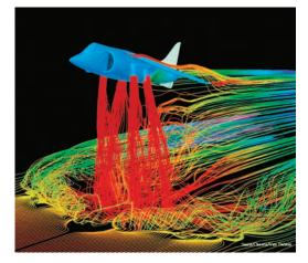
Computed airflow beneath an AV-8B Harrier, 1991.
