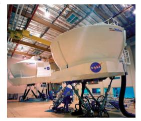
The high bay of the crew vehicle systems research facility: to the front is the Boeing 747-400 cab and to the rear is the advanced cab flight simulator for basic human factors research on pilot workload.
