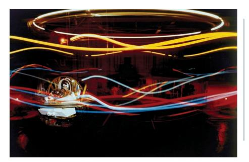
The 5-degreeof-freedom piloted flight simulator in 1962, also shown in time lapsed exposure to display its wide range of motion. window scenes to make the simulation seem even more realistic for the pilot. These began with wooden models of airfields, over which a television camera would fly in response to how the pilot flew the simulator. They evolved into digital images generated by increasingly more powerful computer visualization methods.
