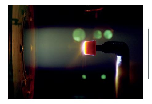
Space shuttle TPS materials in an arc jet test.
