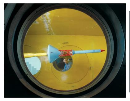
A model of the Apollo command module and launch escape rocket installed in the 9 by 7 foot supersonic wind tunnel in November 1963.
