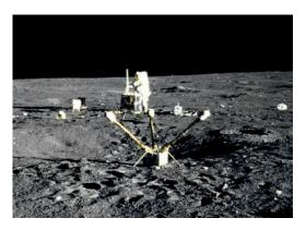
The tri-axis magnetometer used to measure magnetic fields on the Moon.
