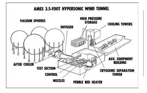
Schematic of the Ames 3.5 foot hypersonic wind tunnel, the site of a quarter of all wind tunnel testing of the Space Shuttle.
