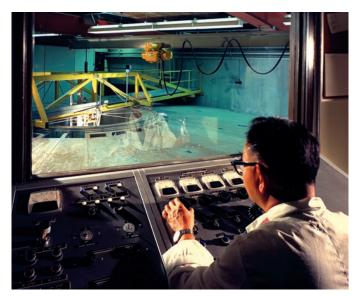
Jiro Oyama in 1968 controlling a life sciences experiment in the Ames 50 foot centrifuge. all this life sciences research, Ames asked its instrumentation group to use the expertise it had earned in building sensors for aircraft to build bioinstrumentation. Under the guidance of John Dimeff, the Ames instrumentation branch built sophisticated sensors and clever telemetry devices to measure and record physiological data with minimal impact on the subjects.
