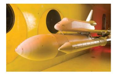
3 percent model of the ascent stack of the Shuttle in supersonic wind tunnel studies for its return to flight. of insulating foam striking the wing during launch would cause a fissure able to produce the sequence deduced by Arnold's team. Once all these pieces were in place, the reconstruction of the tragedy unfolded self-evidently.
