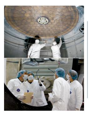
SOFIA primary mirror, in 2008, before and after being coated in the NASA Ames vacuum chamber.
