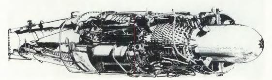
Schematic view of General Electric's TG-180 shows the axial compressor influenced by the NACA eight-stage compressor.
