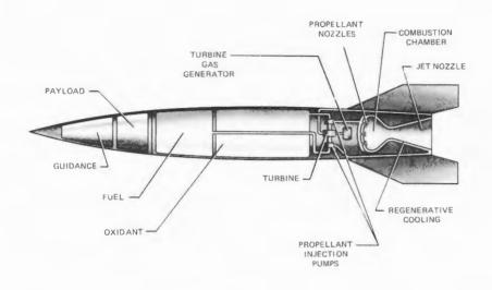
Diagram of a Liquid Propellant Rocket, 1953.
