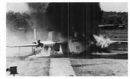
In the crash fire program at the Ravenna Arsenal, a service-weary cargo plane (C-82) was run down a launching track into a crash barrier. Engineers studied the crash fire to determine ignition sources.
