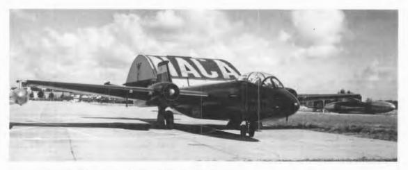
A B-57 aircraft had one engine fueled with liquid hydrogen.
