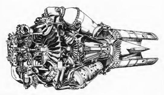
Cutaway view of the Nene engine.
