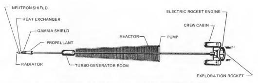
Diagram of electric space vehicle with nuclear power source for a round trip to Mars.
