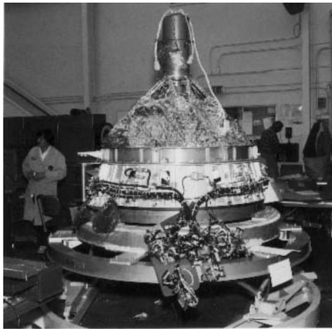
Figure 5.2. Galileo’s despun section receives its cabling.
