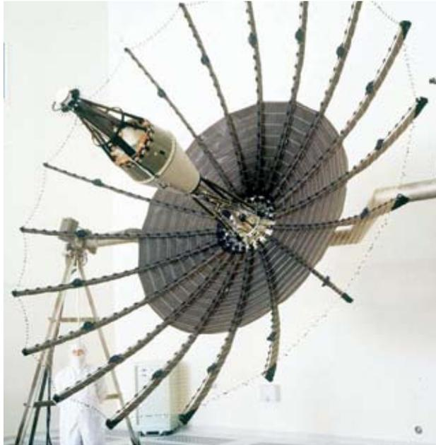
Figure 7.1. The unfurled high-gain antenna. (Adapted from JPL image number 230-893B)
