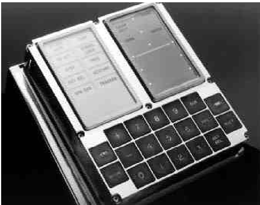
The DSKY eventually used on the F-8 in Phase I of the fly-by-wire program. Warning lights are in the upper left section, displays in the upper right, and the keyboard is in the lower section. (NASA photo EC96-43408-1 by Dennis Taylor).
