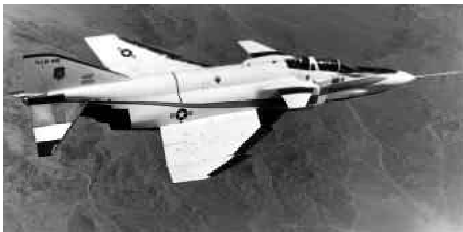
The F-4 that the Air Force converted to an analog fly-by-wire system was considered for Phase II of NASA's project. More funding for the Air Force appeared, however, and the canards were added to make the airplane longitudinally unstable. (U.S. Air Force photo).
