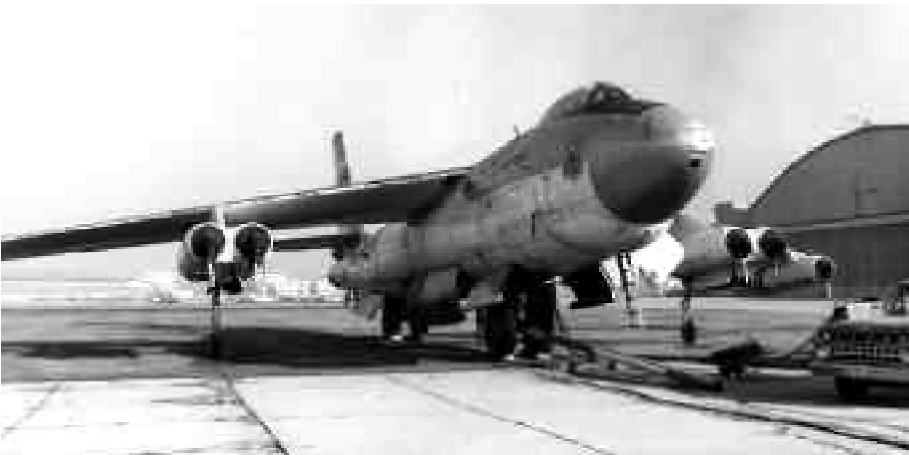
This B-47 was modified by the U.S. Air Force as a fly-by-wire testbed using analog computers. (U.S. Air Force photo).
