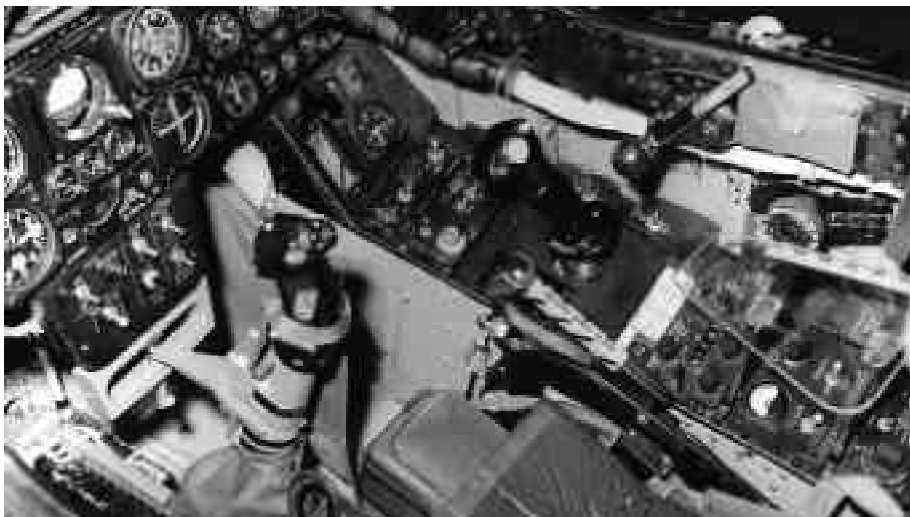
The side-stick was mounted on the right instrument panel. Note the clear plexiglass armrest that could be folded up for stowage. The pilot could still read the instruments under it by lifting his arm a little and looking through the transparent material. (NASA photo E-26466).
