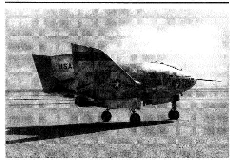
Martin Marietta's X-24A, built for subsonic flight, duplicated the shape of PRIME, which flew at near-orbital velocity. (NASA)(E-18769)
