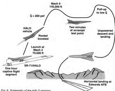
Fig. 6. Schematic of the HALO mission.
