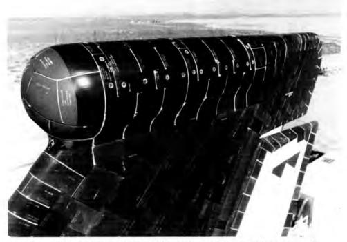
Fig. 7. The SILTS pod on top of the tail of Space Shuttle Columbia. (EC86 33311-33)
