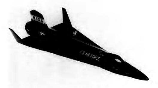
Fig. 2. One of many proposed follow-on X-15 designs with a delta wing modification. (E-13857)
