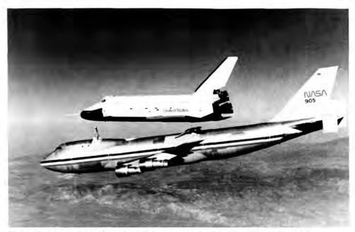
Fig. 2. The Enterprise without the tailcone, separating from the SCA. (E77 8923)
