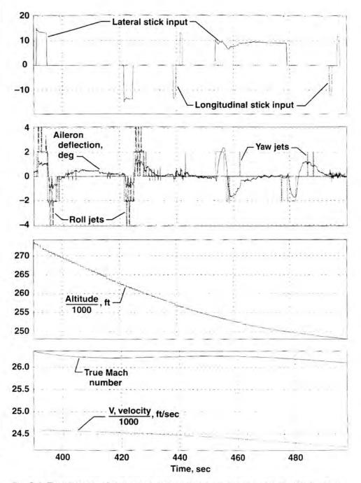
Fig. G-2. Time histories of high speed, high altitude manual maneuvers on STS-2 with a more sensitive time scale.
