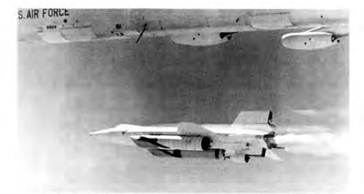
Fig. 4. X-15A-2 with the tanks and full ablative coating a few minutes before reaching its record setting Mach 6.7 speed on October 3, 1967. Pete Knight's flight resulted in shock impingement damage and the loss of the dummy ramjet experiment. (EC68-1889)
