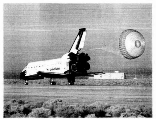
Fig. 10. Columbia and its fully inflated drag chute on flight STS-58. (EC93 42263-2)
