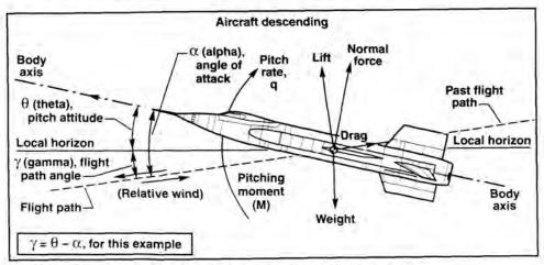
Fig. D-2. Diagram showing longitudinal terms with aircraft descending.
