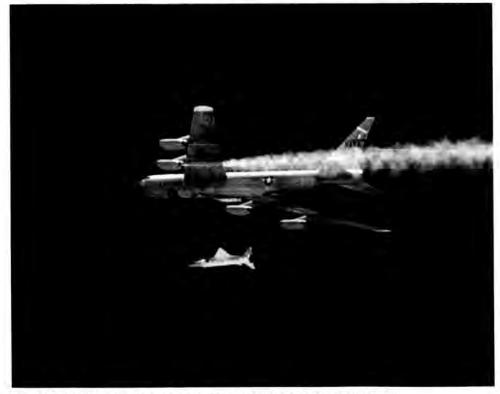
Fig. 6. The X-43 immediately after launch from the B-52 on June 2, 2001. (EC01 182-20)
