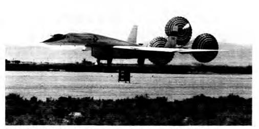
Fig. 6. XB-70A number one with the landing chutes deployed. (ED97 44244-3)
