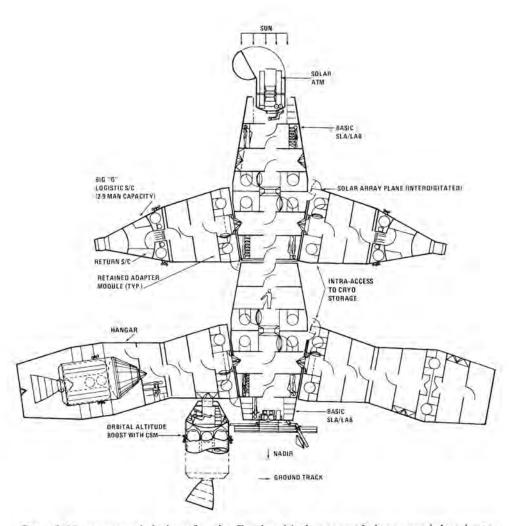
One of 18 conceptual designs for the Earth-orbital spacecraft lunar module adapter laboratory prepared by spacecraft design experts of the MSC Advanced Spacecraft Technology Division. This configuration was developed to illustrate the extent to which the building block philosophy could be carried. It would utilize both Gemini and Apollo spacecraft and would require 2 unmanned launches and 10 manned logistic launches. The report was published 25 April 1968.
