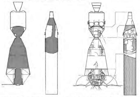
The figures above present two comparisons of the total amount of space available for crewmen to work in the Apollo/SLA Workshop (to the left in each illustration) and the Air Force Manned Orbiting Laboratory. The MOL space could be expanded downward, using more of the empty propellant tank space in the launch vehicle.
