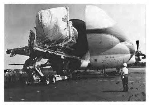
The Skylab airlock module/multiple docking adapter is shown during offloading procedures at Cape Kennedy's Skid Strip, after arrival on the Super Guppy aircraft.
