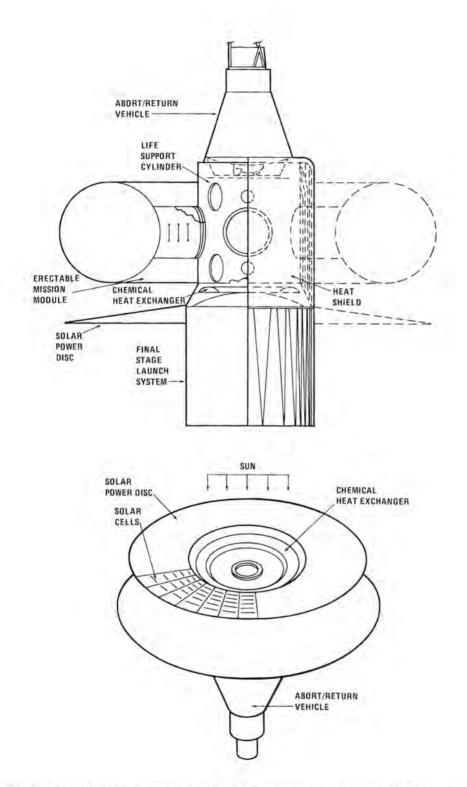
In October 1960 Rene A. Berglund of Langley Research Center's Space Station Office prepared the spacecraft design concept of an inflatable space laboratory based on the Mercury spacecraft.
