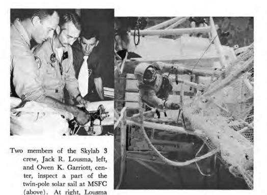
practices erecting the solar sail over a portion of the Orbital Workshop mockup in the MSFC Neutral Buoyancy Tank. Nylon netting was used for this underwater training instead of the aluminized fabric the actual sail was made of.
