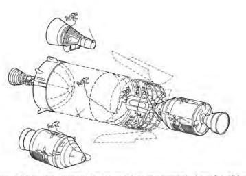
This concept, indicating extravehicular activity accommodations for either the Gemini spacecraft or Apollo command and service modules, was submitted to NASA in January 1966 by Douglas Aircraft Company, Inc. It was part of a report on the orbital S-IVB spent-stage experiment support module feasibility study.
