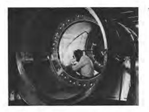
The airlock tunnel assembly was fabricated at the McDonnell Douglas facility in St. Louis. This photo shows the hatch still being tackwelded.
