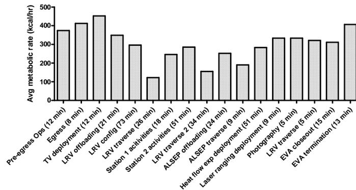
Figure 17. Metabolic expenditures of the first Apollo 15 lunar EVA in chronological order (durations of each activity are noted in parentheses). The average total energy expenditure during the EVA was 1800 kcal. ALSEP = Apollo Lunar Surface Experiments Package, EVA = extravehicular activity, LRV = Lunar Roving Vehicle, TV = television. Data are from Waligora and Horrigan [712].
