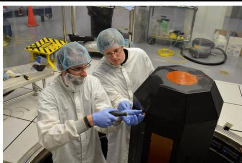
**Archinaut project manager and fellow Made In Space engineer fine-tune the Extended Structure Additive Manufacturing Machine -- the core of this In Space Manufacturing project's innovative, in-space 3-D printing capability -- during thermal vacuum testing at NASA's Ames Research Center in Moffett Field, California.**
