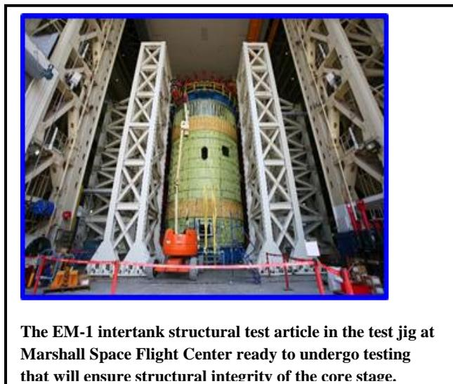
**The EM-1 intertank structural test article in the test jig at Marshall Space Flight Center ready to undergo testing that will ensure structural integrity of the core stage.**
