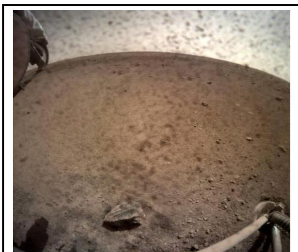
**NASA InSight spacecraft flipped open the lens cover on its Instrument Context Camera (ICC) on Nov. 30, 2018, and captured this view of Mars. Located below the deck of the InSight lander, the ICC has a fisheye view, creating a curved horizon. Some clumps of dust are still visible on the camera's lens. One of the spacecraft's footpads can be seen in the lower right corner. The seismometer's tether box is in the upper left corner.**
