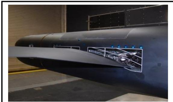
**Shown above is the on-board Laser-Doppler Velocimetry system specifically designed to fit inside a wind tunnel model and accurately measure the turbulent flow in the wing-body juncture region of an aircraft in tests conducted by the Transformational Tools and Technologies (TTT) Project.**
