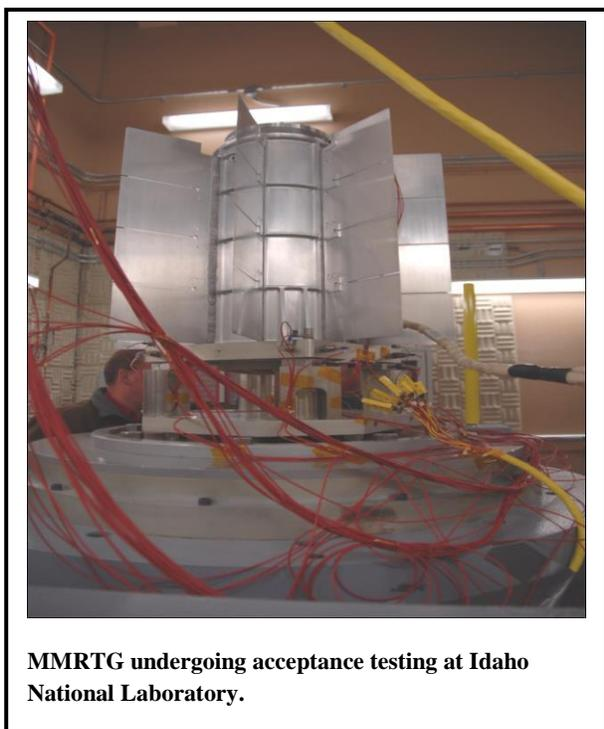
**MMRTG undergoing acceptance testing at Idaho National Laboratory.**
