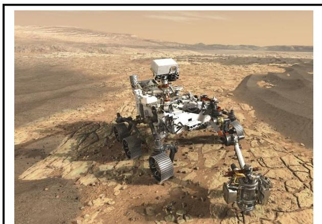
**Mars 2020 will re-use the basic engineering of NASA's Mars Science Laboratory to send a different rover to Mars, with new objectives and instruments, launching in 2020. The rover will carry seven instruments to conduct its science and exploration technology investigations including two contributed by international partners and one to demonstrate a critical technology for future human exploration.**
