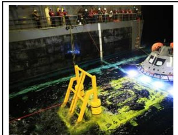
**At night, on November 1, 2018, a test version of the Orion capsule is pulled into the well deck of the USS John P. Murtha during Underway Recovery Test-7 (URT) in the Pacific Ocean. URT-7 is one in a series of tests conducted by the Exploration Ground Systems Recovery Team to verify and validate procedures and hardware that will be used to recover the Orion spacecraft and its crew after it splashes down in the Pacific Ocean following deep space exploration missions.**
