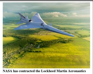
Company to build the X-59 Quiet Supersonic Technology (QueSST) research aircraft, which will generate quiet sonic "thumps."
