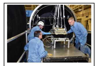
Laser Communications Relay Demonstration engineers place Flight Modem 2 in the thermal vacuum chamber for testing. LCRD's flight modems are a critical part of the LCRD payload. They encode data into laser light to be transmitted to the ground. Laser Communications Relay Demonstration seeks to prove the utility of bidirectional optical communications relay services between geosynchronous orbit and Earth.
