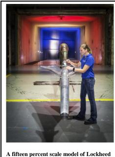
A meter percent scare model of Lockneed Martin's Quiet Supersonic Technology (QueSST) X-plane preliminary design is prepared for testing in in the NASA Langley 14-by-22-Foot Subsonic Tunnel.
