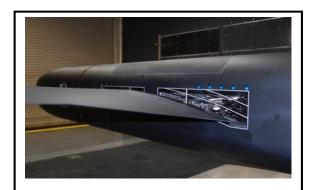
Shown above is the on-board Laser-Doppler Velocimetry system specifically designed to fit inside a wind tunnel model and accurately measure the turbulent flow in the wing-body juncture region of an aircraft in tests conducted by the Transformational Tools and Technologies (TTT) Project.
