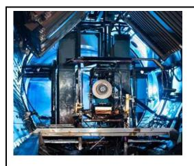
Electric Propulsion thruster in testing. The project will be conducting a spaceflight demonstration of a 30-50kW class solar electric propulsion system on the Lunar Gateway Power and Propulsion Element.
