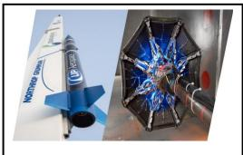
Flight Opportunities conducted a sounding rocket test of Game Changing Development's Adaptable, Deployable, Entry and Placement Technology (ADEPT) aeroshell. Launched on UP Aerospace's SL-12 Launch, the umbrellalike aeroshell achieved full deployment and configuration lock prior to reaching 80 kilometers altitude on descent.
