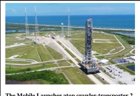
The Mobile Launcher atop crawler-transporter 2 traveling 4.4 miles to Launch Complex 39B to undergo a fit check, followed by several days of systems testing.
