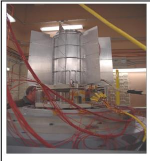
MMRTG undergoing acceptance testing at Idaho National Laboratory.
