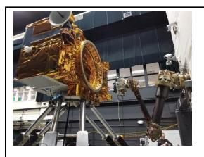
Grapple of Landsat-7 mock up by Robot arm. NASA engineers use mock-ups to evaluate and refine concepts.
