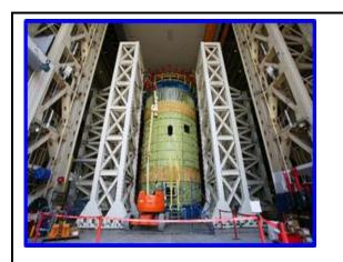
The EM-1 intertank structural test article in the test jig at Marshall Space Flight Center ready to undergo testing that will ensure structural integrity of the core stage.
