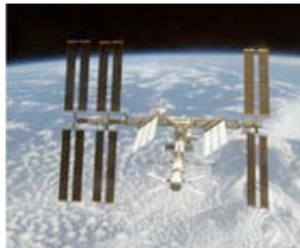
The ISS shows off its new International Partners elements—the European Space Agency's Columbus module, Japan's Kibo Pressurized Module and Logistics Module (all three located where the main body of the ISS meets the truss in the photo), and Canada's Dextre robotic arm—as Space Shuttle Discovery pulls away at the end of STS-124 in June 2008. (Credit: NASA)
