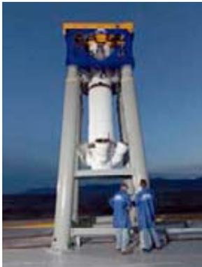
Technicians at Alliant Techsystems (ATK) in Utah inspect the facility's new test stand, which contains the inverted, full-scale inert abort motor for the Orion crew capsule's launch abort system. The abort motor, which anchors atop the capsule, is designed to pull Orion and its crew safely away from the Ares I rocket in the event of a mishap on the launch pad or during the first 300,000 feet of the launch. (Credit: ATK)
