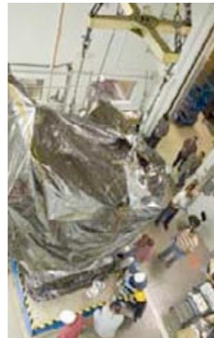
Technicians move LRO into the vibration chamber at the Goddard Space Flight Center for testing in summer 2008 to make sure the spacecraft would be ready to withstand the harsh space environment. Later in the year, NASA transported LRO to the Kennedy Space Center, where it is being prepared for launch. (Credit: NASA/D. McCallum)
