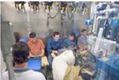
Volunteers work inside a test chamber to help NASA scientists at Johnson Space Center test the Carbon-dioxide and Moisture Removal Amine Swing-bed. For three weeks in spring 2008, the volunteers worked, slept, ate, and exercised in the chamber to simulate activities a crew would perform during a space mission. They reported that while the air smelled "a little artificial," the chamber remained comfortable, indicating that the hardware worked as anticipated. (Credit: NASA)
