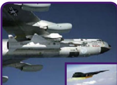
NASA's B-52B mothership carries the X-43A, attached to the nose of a Pegasus rocket booster, under its wing on November 16, 2004. The body of the small, slim X-43A (inset artist's concept) forms critical elements of the vehicle's design. The forebody acts as part of the intake for airflow and the aft section serves as the nozzle. (Photo: C. Thomas/NASA; drawing S. Lighthill)
