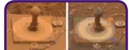
What a difference ten days make: The photo on the left shows a part of *Spirit* covered in a thick layer of red, Martian dust on March 5, 2005. Ten days later, dust-lifting winds had blown the part clean. The solar arrays, which also were blown clean, began collecting more power. (Photos: Cornell/NASA)
