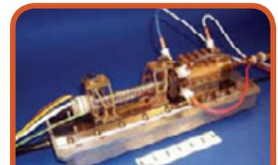
This photo shows a 100-Watt Ka-band traveling wave tube amplifier designed for NASA's 2009 Mars Telecommunication Orbiter mission. (Photo: NASA)
