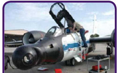
The WAVE project swiveling video recording system sits on the front of NASA's two WB-57 jets like a bulbous nose. The primary optic lens, a 4,150-millimeter reflector telescope, is visible on the right of the spherical turret. NASA partnered with Southern Research Institute, who design gimbal systems for the U.S. Army, to design a large, rotating gimbal to house the cameras that was stable and would remain focused on the speeding Shuttle. (Photo: NASA)
