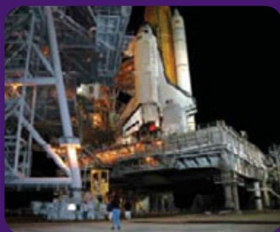
Top far left: In May, NASA rolled the Shuttle from the launch pad back to the Vehicle Assembly Building at Kennedy to take care of liquid hydrogen cut-off sensors that malfunctioned during a tanking test (left). *Discovery* was given a new external tank and a new heater to minimize potential ice and frost buildup on the main engines' feedline bellows. (Photo: NASA)
