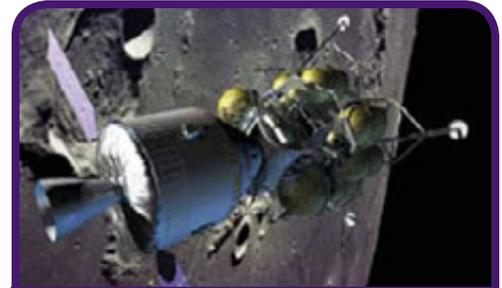
NASA's new exploration vehicle, shown in this artist's concept orbiting the Moon, will have solar panels to provide power. The capsule and the lunar lander will use liquid methane in their engines. NASA chose liquid methane as a fuel in anticipation of future Mars missions, where astronauts can convert Martian atmospheric resources into methane fuel. (Image: NASA/John Frassanito and Associates)
