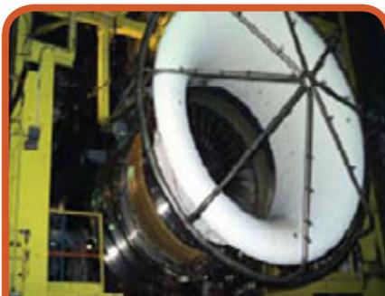
The engine shown above demonstrated a 50 percent reduction in NO<sub>x</sub> emissions during past tests conducted by NASA's program partner, Pratt & Whitney. (Photo: NASA)
