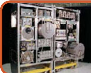
This photo shows the water recovery system for the International Space Station's Environmental Control and Life Support System in 2000. NASA engineers are developing smaller, lighter, and more efficient technologies to reduce the mass of all life support systems for the Station and future space exploration spacecraft and surface habitats. (Photo: NASA)
