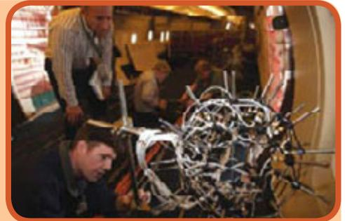
A NASA research team installs a sphere containing 50 sensitive microphones in the cabin of a 757 jet to isolate the sources of noise that are irritating to aircraft crew and passengers. This testing helps engineers develop planes that are quieter and more comfortable. (Photo: NASA)
