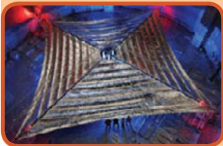
NASA engineers, visible near the bottom of the photo, look at a 20-meter solar sail and boom system after it is fully deployed during testing at NASA's Space Power Facility. Red and blue lights help illuminate the four triangular sail quadrants as they lie outstretched. The sail material is supported by a series of inflatable booms that become rigid in the space environment. The system extends via remote control from a central stowage container about the size of a suitcase. (Photo: NASA)
