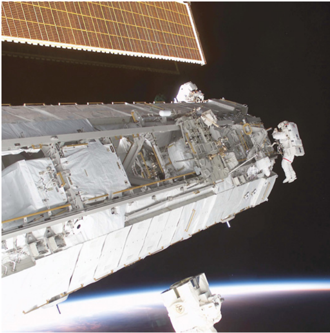
Astronauts Michael E. Lopez-Alegria and John B. Herrington work on the newly installed Port One (P1) truss on the International Space Station (ISS) during the STS-113 mission. The spacewalk lasted 6 hours, 10 minutes. The end effector of the Canadarm2 / Space Station Remote Manipulator System (SSRMS) and Earth's horizon are visible in bottom of frame.
