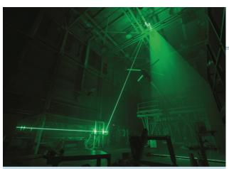
Partnering with NASA, Innovative Scientific Solutions Inc. (ISSI) developed pressure-sensitive paint technology for gathering data from high-speed, unstable surfaces such as rotorcraft blades. The innovation gives NASA new capabilities in aeronautics, and ISSI now sells the product worldwide. Pictured here is a wind tunnel test using a helicopter model equipped with ISSI's paint.
