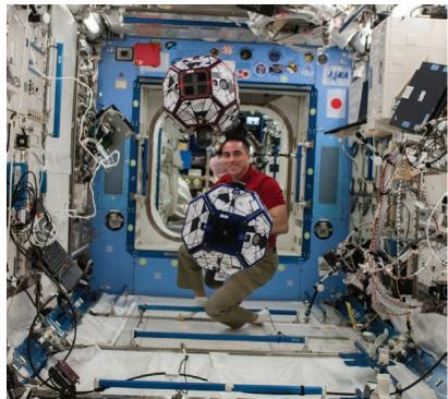
In the ISS's Kibo laboratory, NASA astronaut Chris Cassidy, Expedition 36 flight engineer, conducts a session with a pair of bowling-ball-sized free-flying satellites known as Synchronized Position Hold, Engage, Reorient, Experimental Satellites, or SPHERES. Each satellite is self-contained with power, propulsion, computers, and navigation equipment. The results are important for satellite servicing, vehicle assembly and formation flying spacecraft configurations.
