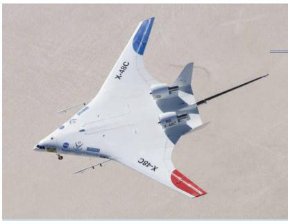
The sub-scale experimental X-48C Hybrid Wing Body flies over Rogers Dry Lake in California. The X-48C is a modification of NASA's X-48B blended wing body aircraft modified to evaluate the low-speed stability and control of a low-noise version of a hybrid-wing-body design. The concepts and technologies being demonstrated through these test aircraft could find their way into all types of new aircraft over the next 20 years, enabling more sustainable, environmentally friendly aviation.
