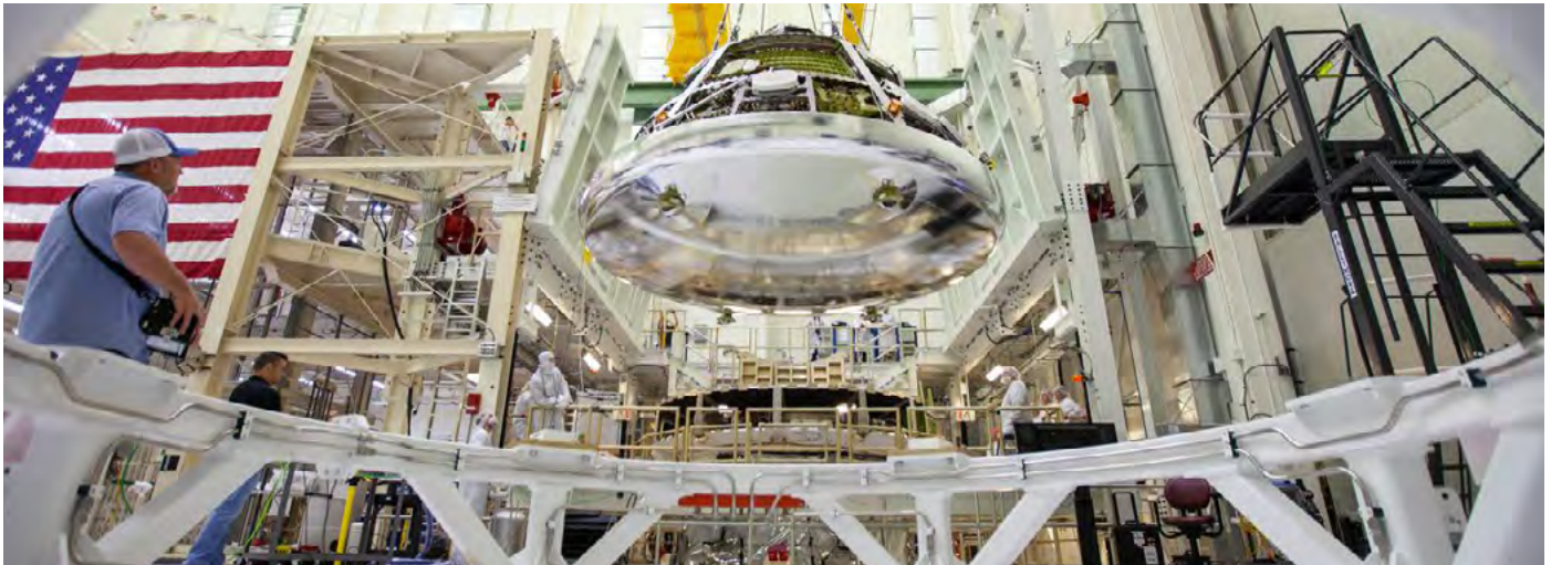
The Orion crew module for Artemis 1 is lifted by crane on July 16, 2019, in the high bay inside the Neil Armstrong Operations and Checkout Building high bay at NASA's Kennedy Space Center in Florida. The crew module will be moved to the final assembly and test cell and work will begin to secure it atop the service module. The Orion spacecraft is being prepared for its uncrewed test flight atop NASA's Space Launch System (SLS) rocket. Artemis 1 is the first test flight of the SLS and Orion spacecraft as an integrated system. Orion will travel thousands of miles beyond the Moon during a mission that will test its systems in space. The spacecraft will return to Earth and splashdown in the Pacific Ocean where it will be retrieved and transported back to Kennedy. Photo Credit: NASA/Ben Smegelsky
