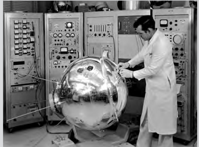
A GSFC scientist examines the atmospheric satellite Explorer XVII prior to launch. (NASA image G-63-4001)
