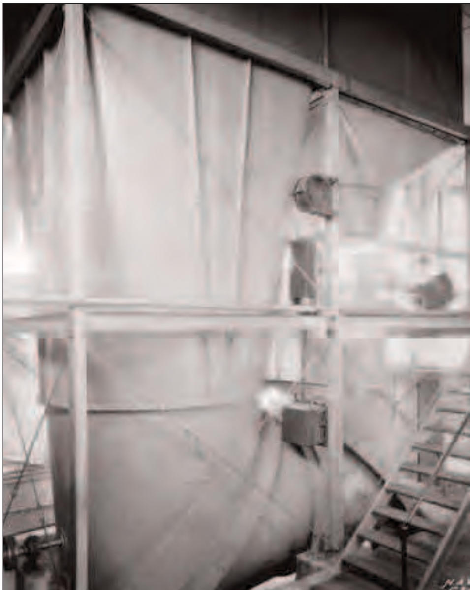
Housed in the same building as the seven- by ten-foot AWT, Langley researchers used the five-foot Vertical Wind Tunnel mainly for spin tests. An engineer kneels on a platform next to the test chamber. In the foreground is the device's (closed) return passage. Like the AWT, the tunnel had an open throat. The vertical tunnel stood thirty-one feet tall and was twenty feet long and ten feet wide. It was not ready for operation until early 1931. NASA Image #EL-1999-00410 (LaRC)
