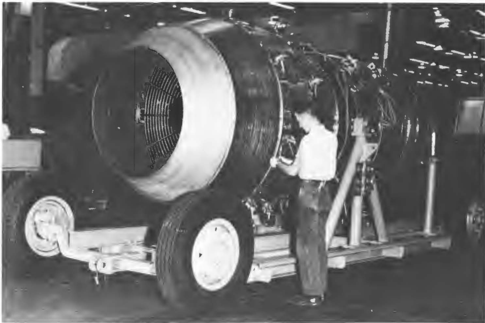
Fig. 44. Pratt & Whitney's model 304 engine using liquid hydrogen as fuel. Visible inside the nozzle is the afterburner fuel injector. The engine was first tested in September 1957. The numerous wires on the engine led to sensors for measuring performance. (Courtesy of Pratt & Whitney.)
