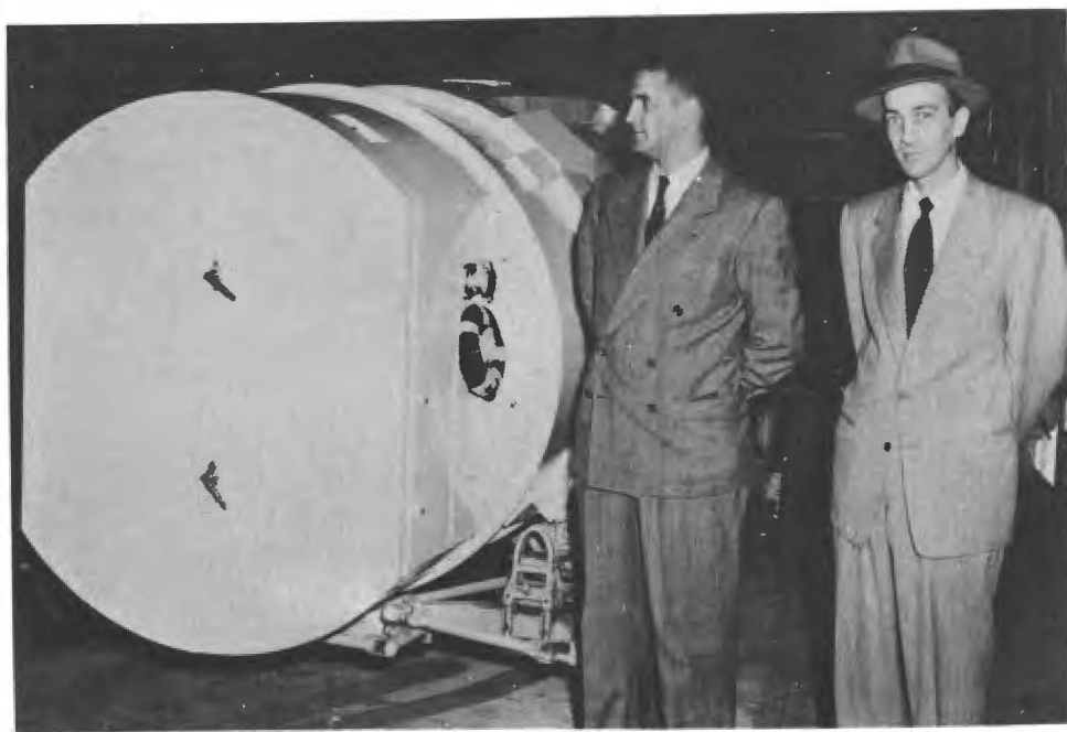
Fig. 13. Air-transportable dewar for 750 liters of liquid hydrogen developed by H. L. Johnston, ca. 1952. Howard Altman is on the left. (Courtesy of H. A. Altman.)
