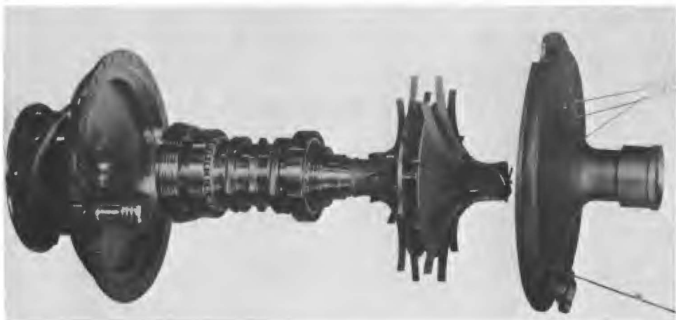
Fig. 41. Pratt & Whitney's liquid-hydrogen pump for the model 304 jet engine. The seal between the rotor and bearings operated dry; the bearing lubrication was conventional. (Courtesy of Pratt & Whitney.)
