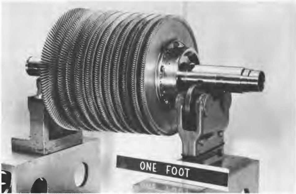
Fig. 43. High-pressure group of the 12 stages of hydrogen turbine expansion used by Pratt & Whitney's model 304 engine. The early stages operated near 1000 K. (Courtesy of Pratt & Whitney.)
