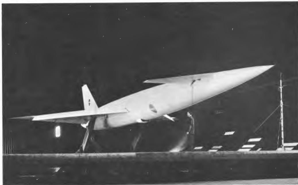
Above: A North American XB-70 in flight. Below: The canard configuration in 40- by 80-foot tunnel.
