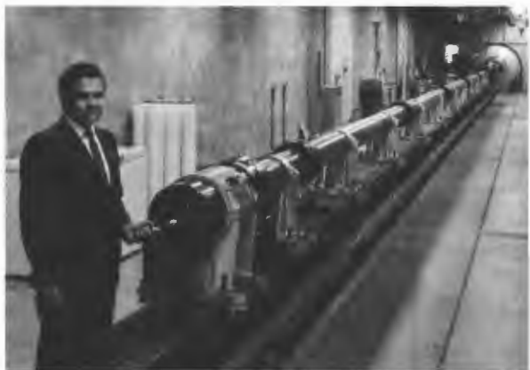
Light-gas gun. Thomas N. Canning holds model that is fired down range. Plastic pistons are seen stacked against wall at left.
