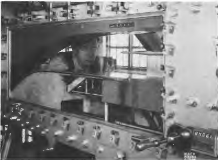
Sliding-block throat of 8- by 8-inch tunnel, prototype of 6- by 6-foot tunnel, which was built to test the sliding-block throat.
