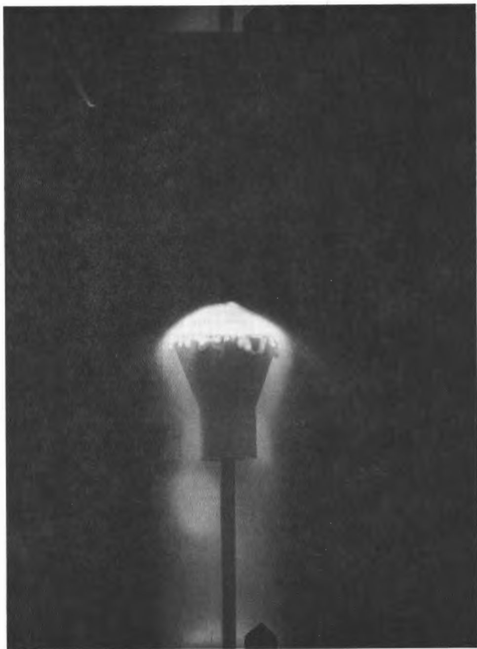
Ablation of Mercury capsule model.
