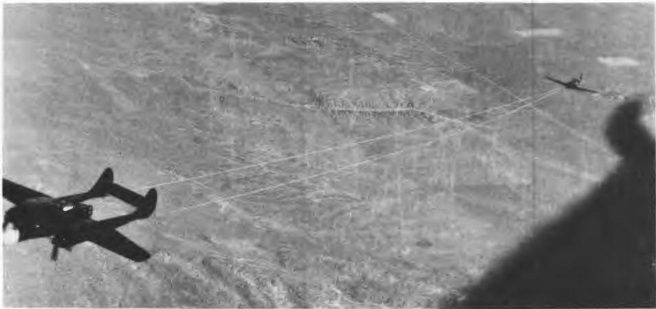
Northrop P-61A towing propellerless P-51B.
