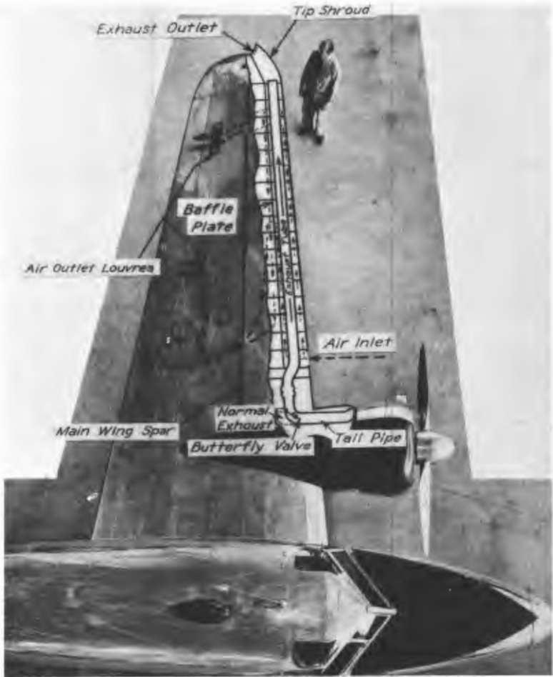
Diagram of the system using exhaust-heated air to prevent icing on the Lockheed 12A wings.
