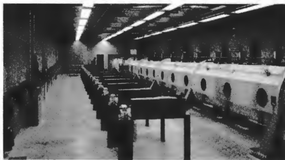
Above: Shock tunnel (air gun) composed of driver and shock tubes. At left: Test section of aerodynamic facility; this is the "counterflow" region where the test model and the air jet, traveling in opposite directions, meet.
