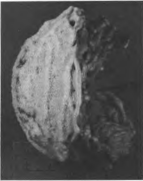
Artificial fluffy meteorite ablated in arc-jet.
