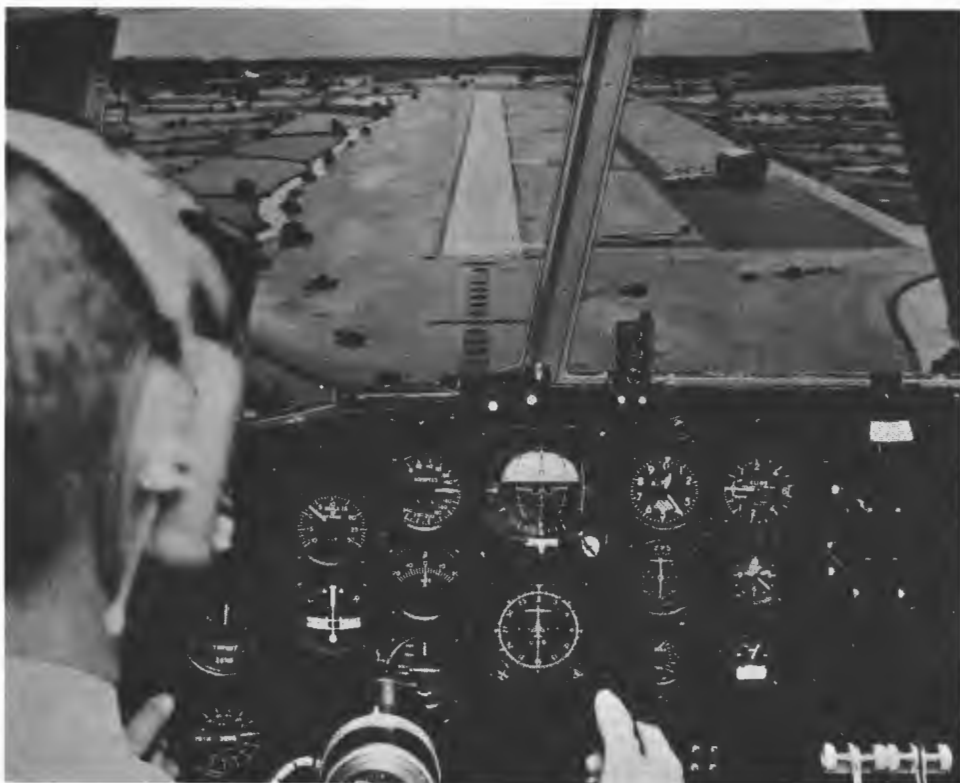
Upper left: Schematic drawing of flight simulator for advanced aircraft. Upper right: The redifon visual cue generator. Below: View of simulated runway and landscape from simulator cockpit.
