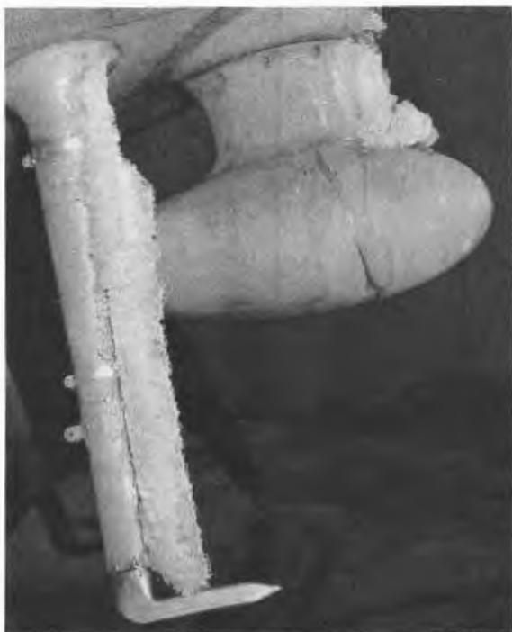
Ice formation on radio antenna and airspeed mast of C-46 airplane.
