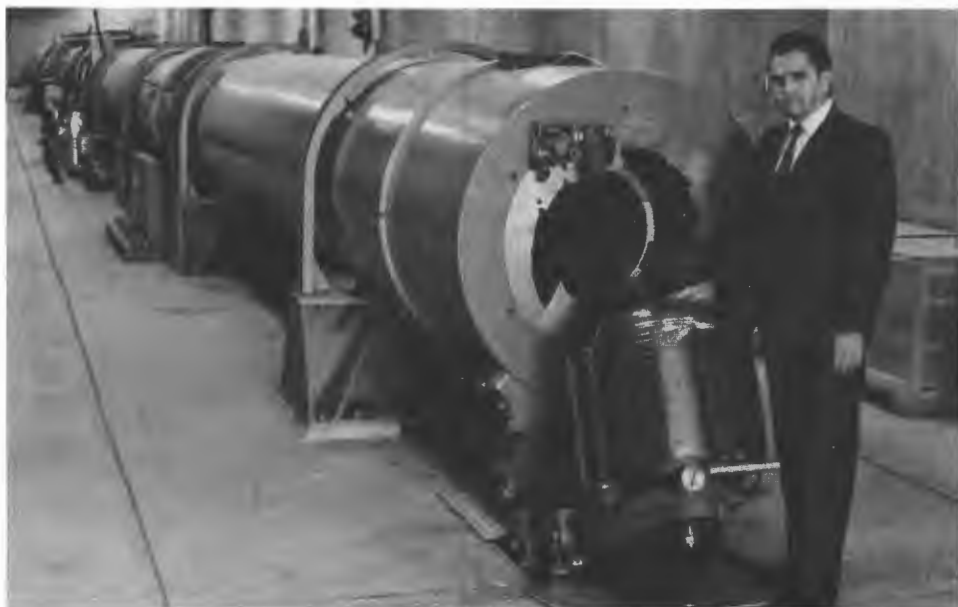
Above: Shock tunnel (air gun) composed of driver and shock tubes. At left: Test section of aerodynamic facility; this is the "counterflow" region where the test model and the air jet, traveling in opposite directions, meet.
