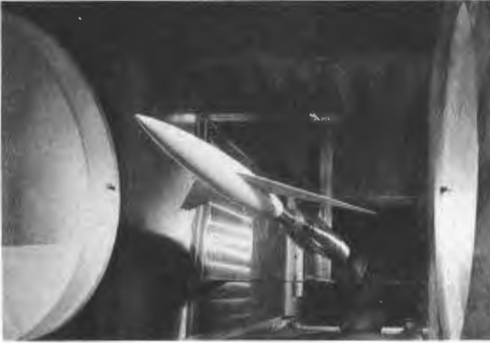
Throat of 6 × 6-foot supersonic tunnel showing schlieren windows.
