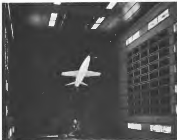
Below: A model of the 14-foot transonic tunnel. At right: A model in the test section of the 14-foot tunnel.
