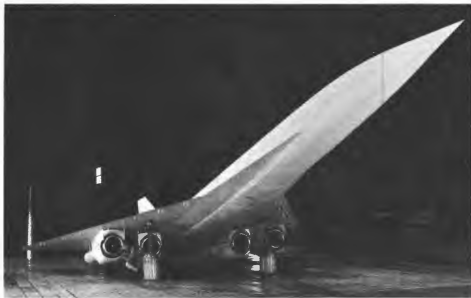
Above: OGEE wing model in transonic tunnel. Below: Double-delta supersonic transport model in 40- by 80-foot tunnel.
