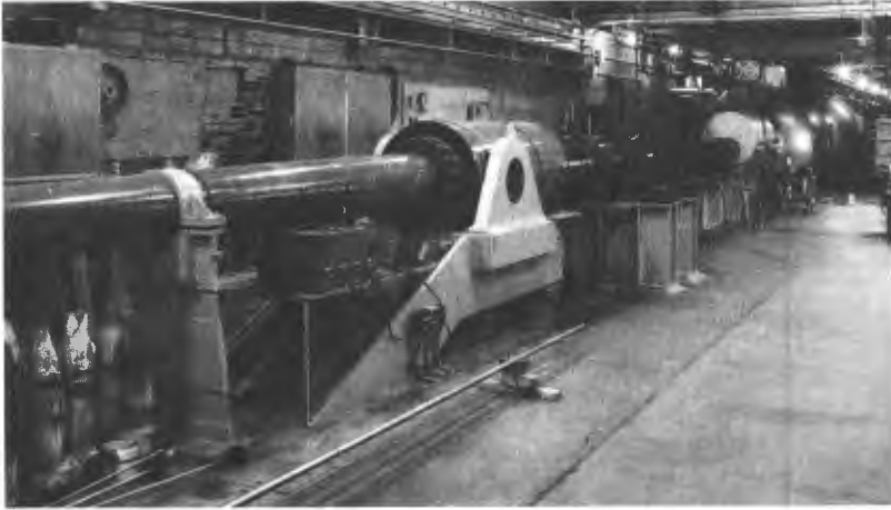
June 25, 1965, deformable-piston gun applied to main range. Used plastic pistons are under gun at left.
