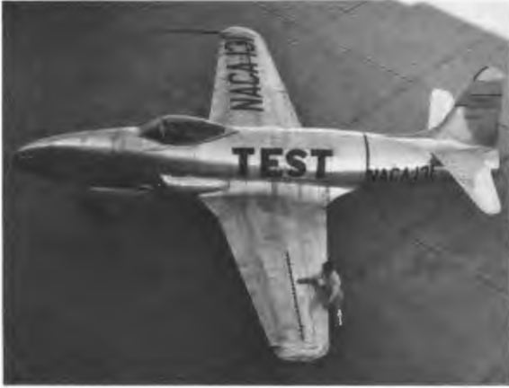
Lockheed P-80 with vortex generators installed ahead of ailerons to combat aileron buzz.
