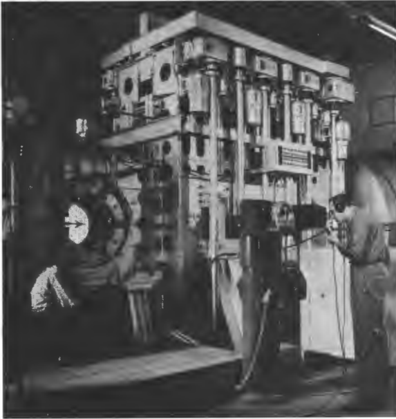
1- by 3-foot blowdown tunnel with variable-geometry-throat mechanism.
