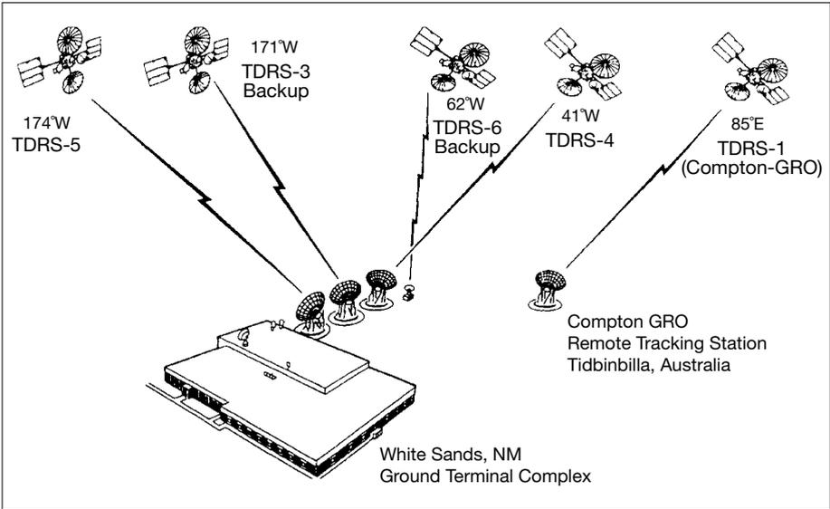
The first generation Tracking and Data Relay Satellite System (TDRSS) constellation as it appeared in 1994, with five orbiting satellites—two operational and three backups—in communication with the White Sands Ground Terminal (WSGT) and the GRO Remote Terminal System. (Space Shuttle Mission STS-54 Press Kit, January 1993, NASA Headquarters)
