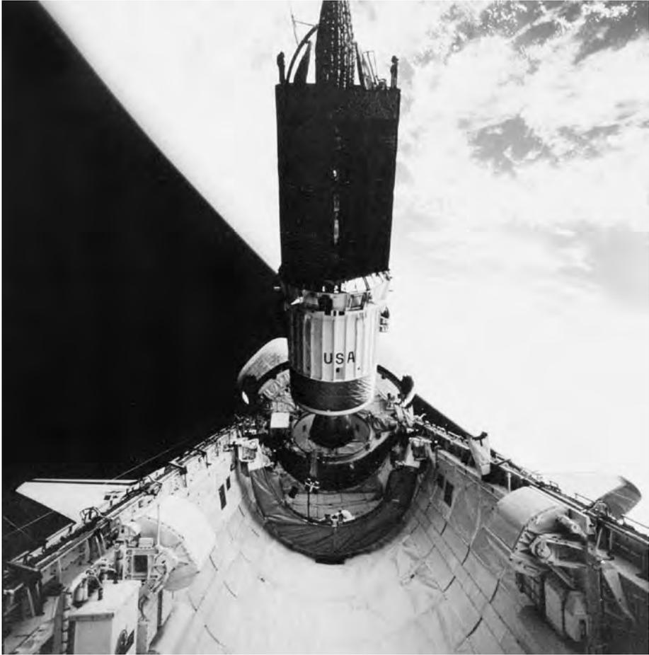
The Tracking and Data Relay Satellite (TDRS) stowed in the Shuttle payload bay is raised to a vertical attitude in preparation for deployment from low-Earth orbit. Shown here is TDRS-6 being deployed from the Shuttle *Endeavour* on STS-54 on 13 January 1993. Clearly visible is one of the Single Access (SA) parasol antennas seen folded at the top. The solar arrays are also in the stowed position. The Inertial Upper Stage (IUS) is visible below the satellite. (NASA Image Number STS054-71-025)
