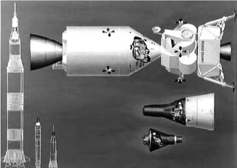
This vintage 1964 drawing shows the relative sizes of the Mercury, Gemini and Apollo spacecraft, as well as the Atlas, Titan and Saturn V used to launch them. The combined weight of the Apollo Command Module, Service Module and Lunar Module at launch was 47,630 kilograms (105,000 pounds). By comparison, typical weight of the Mercury capsule was only 1,950 kilograms (4,300 pounds) and the Gemini 3,760 kilograms (8,300 pounds). (NASA Image Number S64-22331)
