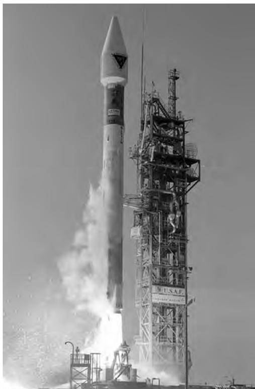
Unlike the first generation of Tracking and Data Relay Satellites, TDRS-H, I and J were launched using expendable launch vehicles. Here, TDRS-H rises from PAD36A, Cape Canaveral Air Force Station at 8:56 a.m. EDT on 30 June 2000 atop an Atlas IIA/Centaur launch vehicle. The new satellites augmented TDRSS's existing S- and Ku-band capabilities by adding a Ka-band capability. (NASA Image Number KSC-00PP-0825)
