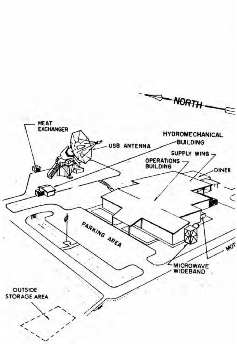
The Guam Apollo Station had as its centerpiece a 9-meter USB antenna used to communicate with the Apollo spacecraft during the near-Earth and trans-lunar portions of the mission. The station was one of the longest lived in the network, operating for over
