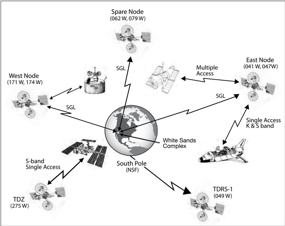
The Tracking and Data Relay Satellite System, TDRSS. The first generation Space Network used S and Ku-band to relay communications from up to 20 satellites at the same time. Ka-band capability was added beginning with three second generation satellites in the early 2000s. (Adapted from Roger Flaherty, Satellite Communications, Goddard Space Flight Center, May 2002)
