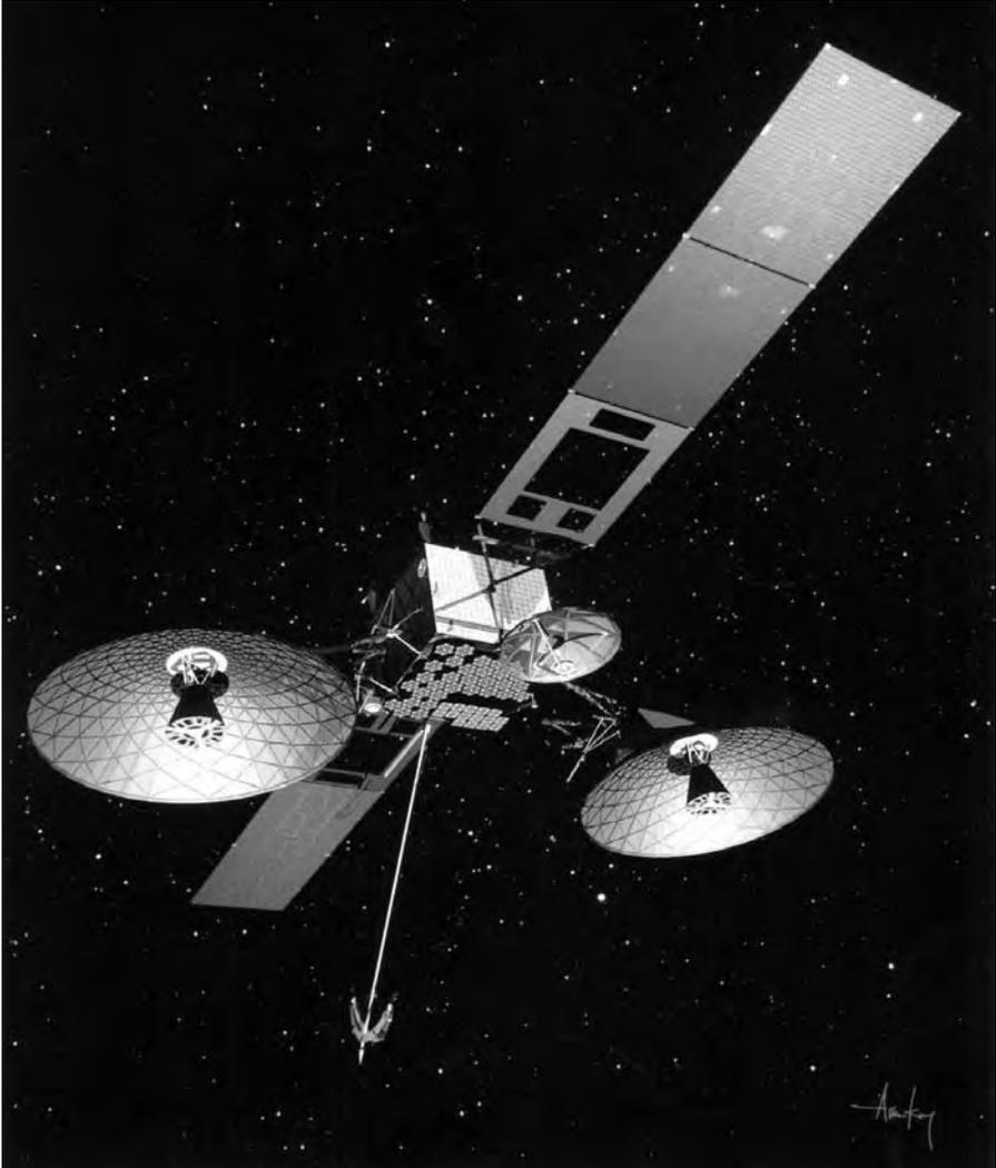
TDRS-H, I, and J could provide over two and a half times the data relay capability of its predecessors by using Ka-band and other new features. (Photograph courtesy of NASA, [www.gsfc.nasa.gov/topstory/20021127tdrs\\_j.html](http://www.gsfc.nasa.gov/topstory/20021127tdrs_j.html), accessed October 2, 2005)
