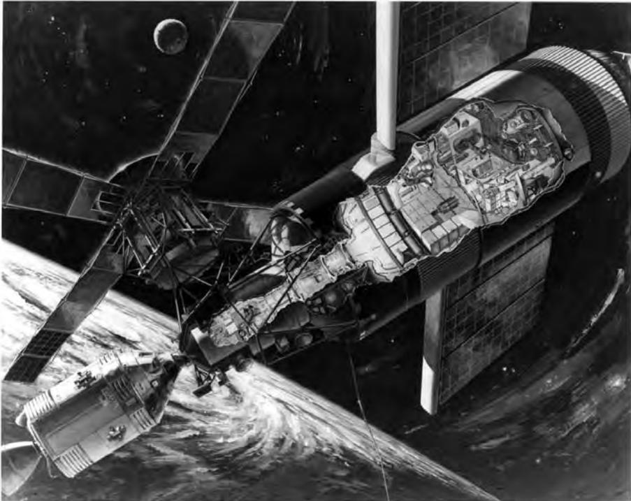
Skylab consisted of four major modules: the Orbital Workshop, Airlock Module, Multiple Docking Adaptor and Apollo Telescope Mount (ATM). The Orbital Workshop was a converted S-IVB third stage of a Saturn V. The ATM could not be accessed from the rest of the space station and a spacewalk was required to reach it. Launched in 1973, three crews visited the station between May 1973 and February 1974. Skylab remained in orbit until 1979. (NASA Image Number MSFC-72-SL-7200-110)
