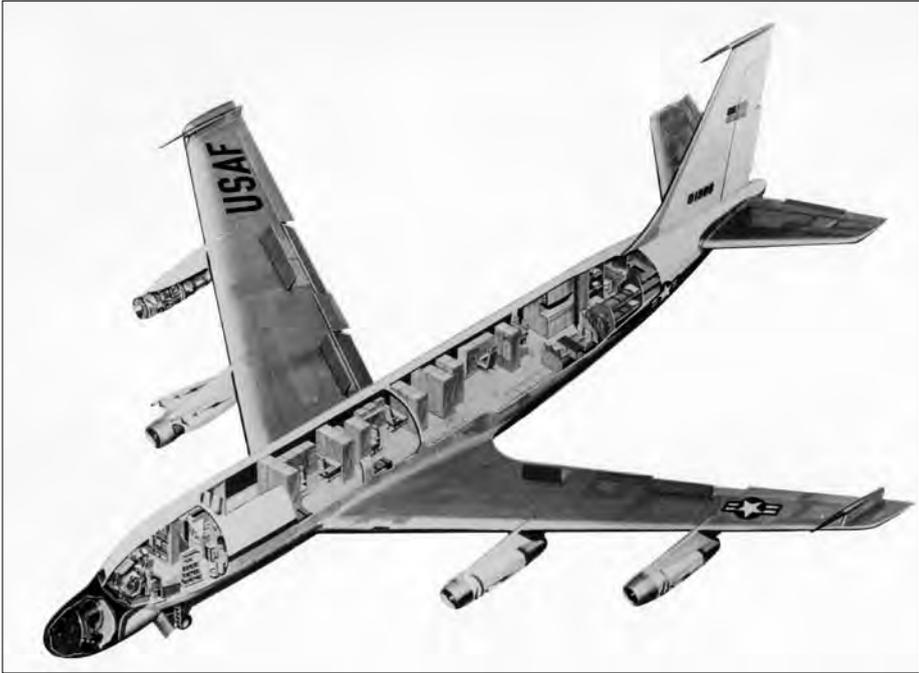
The Apollo Range Instrumentation Aircraft (ARIA) served as airborne relay points between the Apollo spacecraft and the rest of the network. About the size of a 707 jetliner, NASA borrowed these converted Air Force C-135A cargo airplanes to support launch and reentry communications during the Apollo years. (Folder 8788, NASA Historical Reference Collection, NASA History Division, NASA Headquarters, Washington DC)
