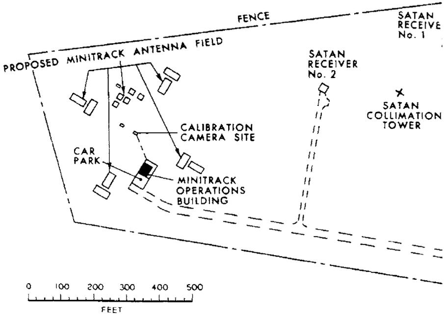
Layout of the Orroral Valley STADAN Station. Note that the Minitrack array transferred from Woomera was eventually placed further west of the SATAN receivers than shown
