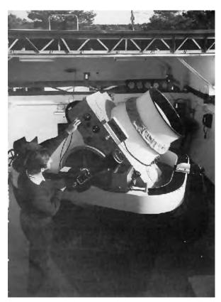
An optical satellite tracking network using Baker-Nunn cameras established by the Smithsonian Astrophysical Observatory was in place by the late 1950s. The camera would alternately track a satellite and the star background to obtain a fix on its location. Baker-Nunn cameras were also used extensively by the Air Force to track military satellites. (http://history.nasa.gov/SP-4202/p9-151.jpg)
