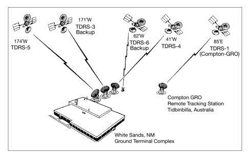
The first generation Tracking and Data Relay Satellite System (TDRSS) constellation as it appeared in 1994, with five orbiting satellites—two operational and three backups—in communication with the White Sands Ground Terminal (WSGT) and the GRO Remote Terminal System. (Space Shuttle Mission STS-54 Press Kit, January 1993, NASA Headquarters)
