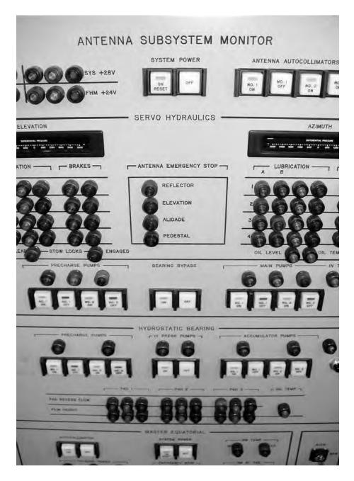
A vintage 1960s Antenna Control Unit (ACU). Graphical computer displays, touch screens and joysticks have, for the most part, replaced the lights and buttons of the old ACUs. Shown is a control unit on display at the Space Museum at the Canberra Deep Space Communication Complex in Tidbinbilla. (Photograph by the author)
