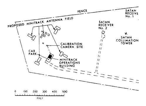
Layout of the Orroral Valley STADAN Station. Note that the Minitrack array transferred from Woomera was eventually placed further west of the SATAN receivers than shown
