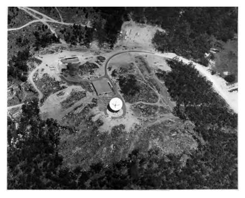
Aerial view of the Apollo Station at Honeysuckle Creek, Australia with its 26-meter (85-foot) Unified S-Band antenna. At the upper left are the diesel fuel tanks for the power generators. Because of its remote location in a national forest, this crucial Apollo Station was run entirely off generator power. (Un-numbered photograph, Box 18, NASA Australian Operations Office, Yarralumla, ACT)
