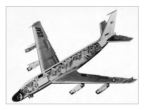
The Apollo Range Instrumentation Aircraft (ARIA) served as airborne relay points between the Apollo spacecraft and the rest of the network. About the size of a 707 jetliner, NASA borrowed these converted Air Force C-135A cargo airplanes to support launch and reentry communications during the Apollo years. (Folder 8788, NASA Historical Reference Collection, NASA History Division, NASA Headquarters, Washington DC)
