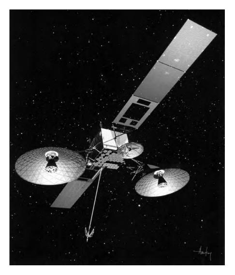
TDRS-H, I, and J could provide over two and a half times the data relay capability of its predecessors by using Ka-band and other new features. (Photograph courtesy of NASA, www.gsfc.nasa.gov/topstory/20021127tdrs\_j.html, accessed October 2, 2005)
