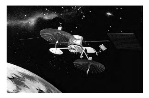
A drawing of the TDRS-3 spacecraft. The Tracking and Data Relay Satellite System (TDRSS) provides nearly uninterrupted communications with the International Space Station (ISS), the Space Shuttle and Earth orbiting satellites, replacing the intermittent coverage provided by the Spaceflight Tracking and Data Network (STDN) ground stations. (NASA Image Number MSFC-8893551)
