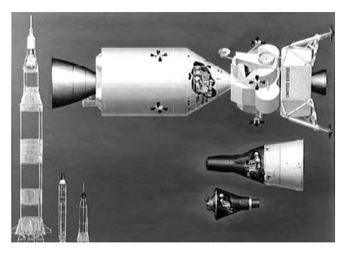
This vintage 1964 drawing shows the relative sizes of the Mercury, Gemini and Apollo spacecraft, as well as the Atlas, Titan and Saturn V used to launch them. The combined weight of the Apollo Command Module, Service Module and Lunar Module at launch was 47,630 kilograms (105,000 pounds). By comparison, typical weight of the Mercury capsule was only 1,950 kilograms (4,300 pounds) and the Gemini 3,760 kilograms (8,300 pounds). (NASA Image Number S64-22331)
