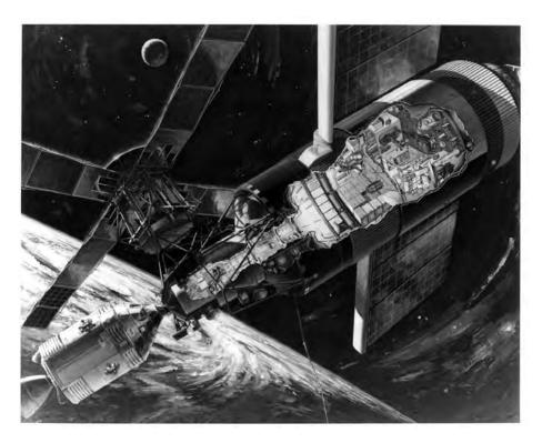
Skylab consisted of four major modules: the Orbital Workshop, Airlock Module, Multiple Docking Adaptor and Apollo Telescope Mount (ATM). The Orbital Workshop was a converted S-IVB third stage of a Saturn V. The ATM could not be accessed from the rest of the space station and a spacewalk was required to reach it. Launched in 1973, three crews visited the station between May 1973 and February 1974. Skylab remained in orbit until 1979. (NASA Image Number MSFC-72-SL-7200-110)
