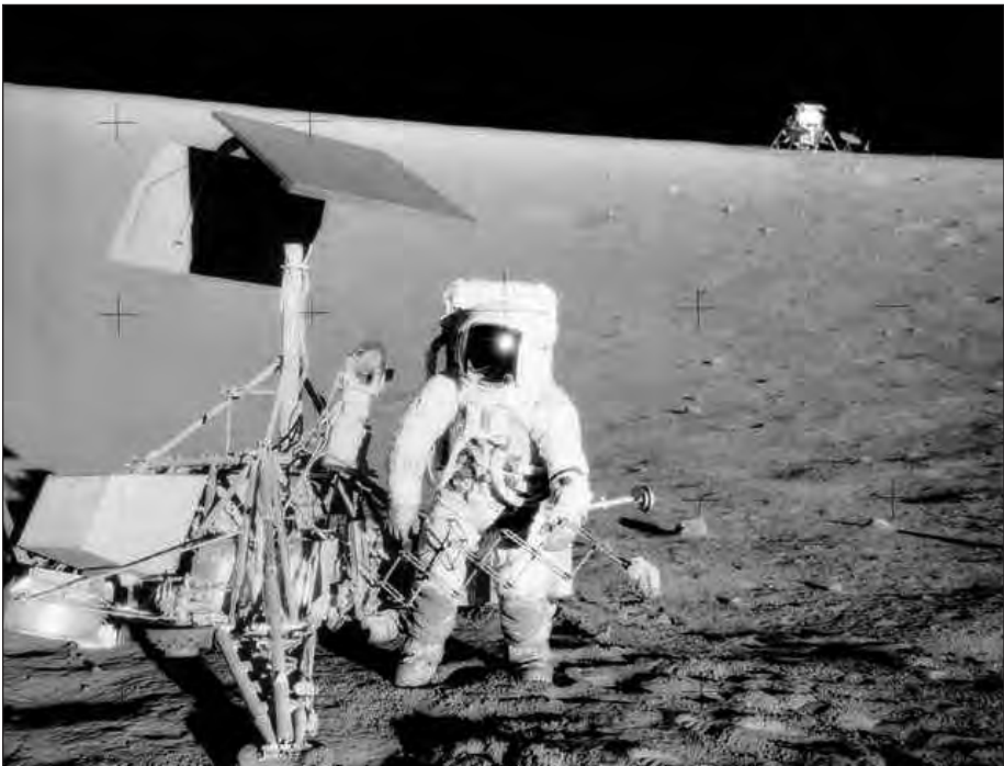
Apollo 12 astronaut Pete Conrad retrieves camera from Surveyor 3 standing in the Moon’s Ocean of Storms. Returned to Earth on Apollo 12 for analysis, the camera was eventually delivered to William Pickering (Photo: NASA/JPL-Caltech Archives, Photo number P10623B).
