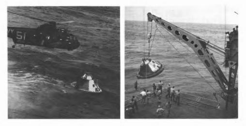
A Navy helicopter hovers over spacecraft 017 awaiting the recovery ship after the *Apollo 4* (AS-501) mission—the first Saturn V flight—on November 9, 1967. Frogmen attached the flotation collar to the command module after splashdown. On arrival of the U.S.S. *Bennington*, CM 017 is hoisted aboard.
