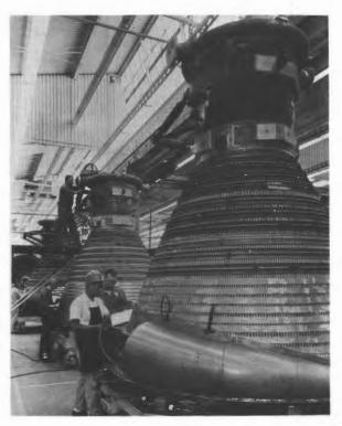
The manufacturing line for thrust chambers of the F-1 rocket engine shows the size of the powerful engine. Five of the engines were used in a cluster to launch each of the Saturn V space vehicles. Rocketdyne photo.
