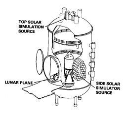
A cutaway view of the large space environment chamber in the Space Environment Simulation Laboratory at Manned Spacecraft Center shows how Apollo spacecraft components were tested at the extreme temperatures they would meet in space.
