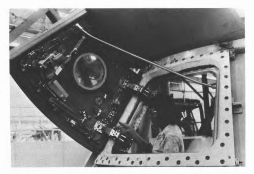
The new unified hatch of the Apollo CM is checked at North American after its development, testing, and manufacture. The Block I hatch on the ill-fated CM 012 had consisted of an outer and an inner hatch.
