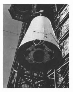
LM-1, fitted inside spacecraftlunar module adapter 7, is raised to position at Kennedy Space Center in preparation for the Apollo 5 mission. 1967
