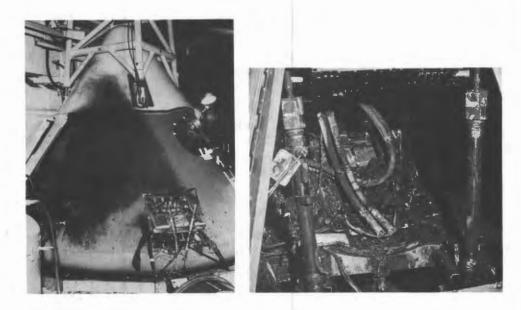
Effects of the flash fire on CM 012, photographed shortly after the fatal January 27, 1967, Apollo 204 accident: exterior of the command module, left, and interior, right.
