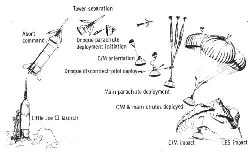
The planned sequence of events for the BP-12 suborbital flight is shown above. At right is the liftoff.
