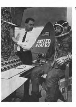
Spacesuits and computers were used in combination with a simplified mockup of NASA's Apollo moonship (background) at the Aeronautical Division of Honeywell in Minneapolis, where the stabilization and control system for the three-man spacecraft was developed. In the photo engineer Bill Summers (left) made final adjustments on one of a number of computers which would feed simulated flight information to engineer-test pilot Jim O'Neil (right) when he was inside the command module mockup.
