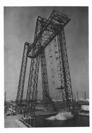
A boilerplate spacecraft is dropped in the impact test facility at NAA's Downey, Calif., plant. The tower was 43.6 meters (143 feet) high, the pendulum pivot was 38.1 meters (125 feet), and maximum impact velocity was 12.2 meters (40 feet) per second vertical and 15.2 meters (50 feet) per second horizontal. —NAA photo.
