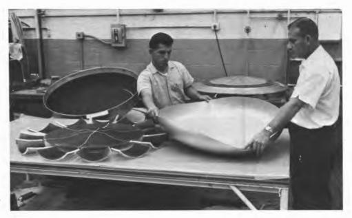
A new design of the LEM landing gear foot pad (Aladdin's lamp) was checked by shopmen before the honeycomb core, left, was placed inside for bonding.
