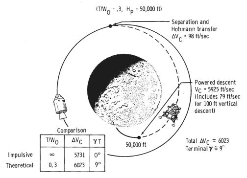
Theoretical optimum lunar model descent with thrust-to-weight ratio (initial value in lunar orbit) at 0.3, height at perilune of the transfer orbit at 15 200 meters (50 000 feet), and using the Hohmann transfer technique. The diagram showed the velocity change ( $\Delta V_e$ , in feet per second) and approach flight-path angle ( $\gamma$ ) close to those for an impulsive orbital change (an instantaneous change, without time value, taken as the ultimate though unachievable ideal for comparison).
