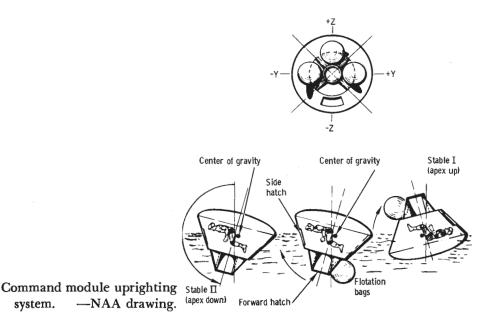
tests with inflatable bags (rather than the rigid foam spheres used previously), while MSC would evaluate the use of an extendable boom with two flotation bags.
