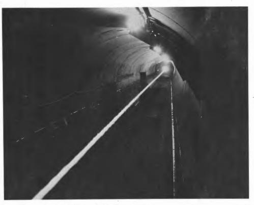
The Hypervelocity Ballistic Missile Range at Ames Research Center launched projectiles at speeds up to 27 360 kilometers (17 000 miles) per hour to simulate micrometeoroids in outer space.
