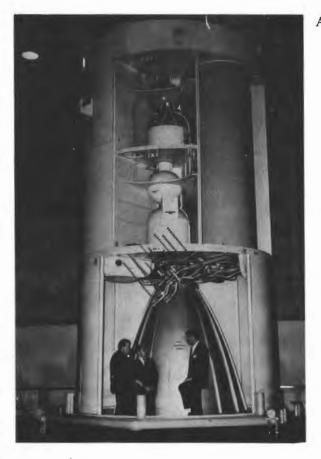
An Apollo service module mockup showing the portion that contained the main rocket engine and propellant supply to be used for maneuvers to and from the moon. Produced by Aerojet-General Corporation under contract to NAA, the engine could provide more than 89 000 newtons (20 000 pounds) of thrust to keep Apollo on course and to perform other missions. Standing by the multiple-start engine's flaring skirt were NAA and Aerojet rocket engineers.
