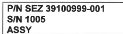
Figure 5: Example of identification markings/engravings on hardware that is part of an assembly.
