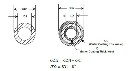
It is recommended that for such applications, both the final dimensions and the "machine to" dimensions should be specified on the engineering drawing.
