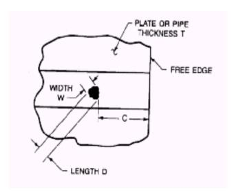
C = Clearance spacing between closest edge of discontinuity and free edge
