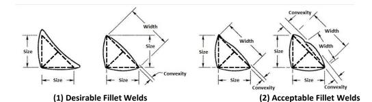
Note: Convexity of a weld or individual surface bead with dimension Width shall not exceed the value of the following table.
