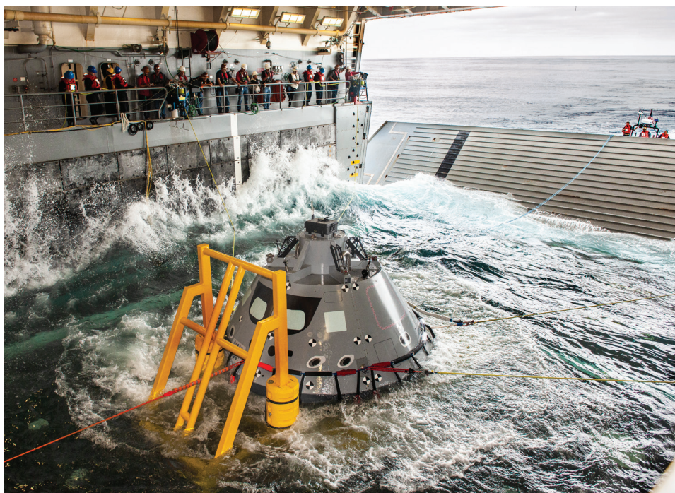
NASA Recovery Team members watch as a test version of the Orion capsule is pulled into the flooded well deck of the USS John P. Murtha, during Underway Recovery Test-7 (URT-7) on Oct. 30, 2018. URT-7 is one in a series of tests that the Exploration Ground Systems Recovery Team, along with the U.S. Navy and Lockheed Martin, are conducting to verify and validate procedures and hardware that will be used to recover the Orion spacecraft after it splashes down in the Pacific Ocean following deep space exploration missions. Orion will have emergency abort capability, sustain the crew during space travel and provide safe re-entry from deep space return velocities. Photo credit: NASA/Tony
