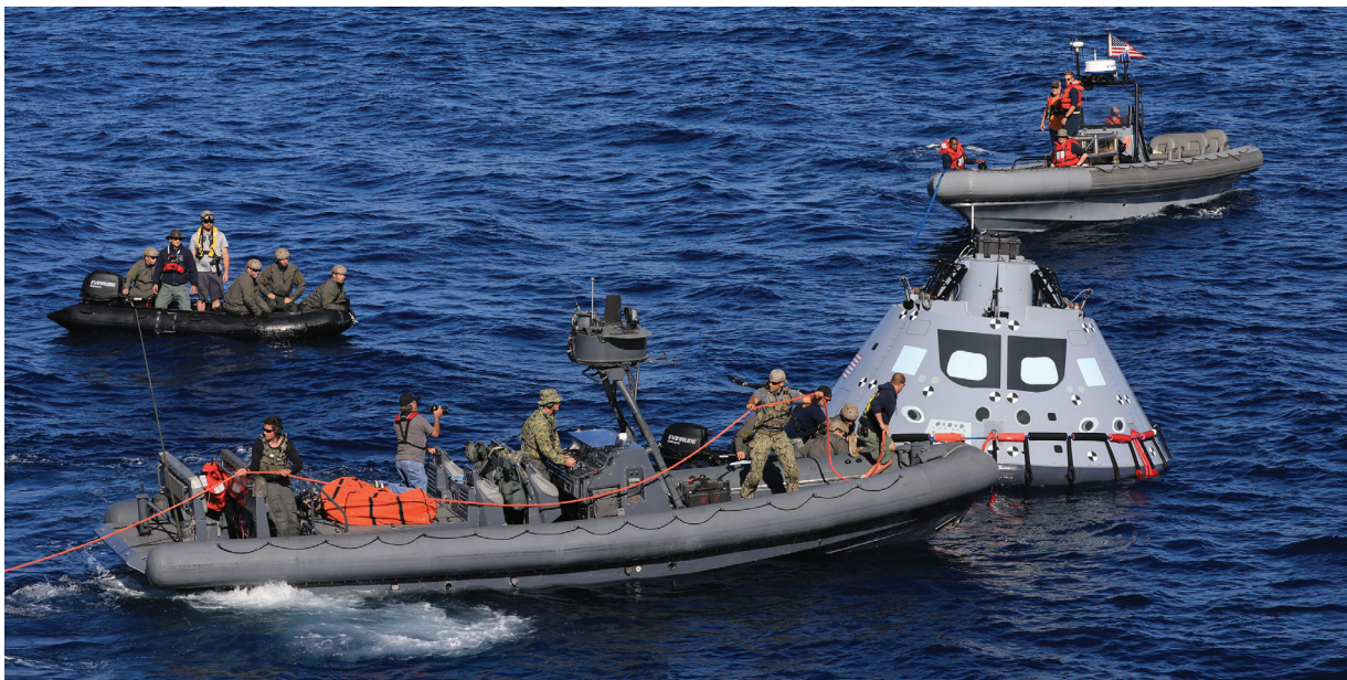
During Underway Recovery Test-7 (URT-7), U.S. Navy divers approach a test version of the Orion capsule to practice securing it for recovery into the well deck of an amphibious assault ship on Oct. 31, 2018 in the Pacific Ocean. Photo credit: NASA/Kim Shiflett
