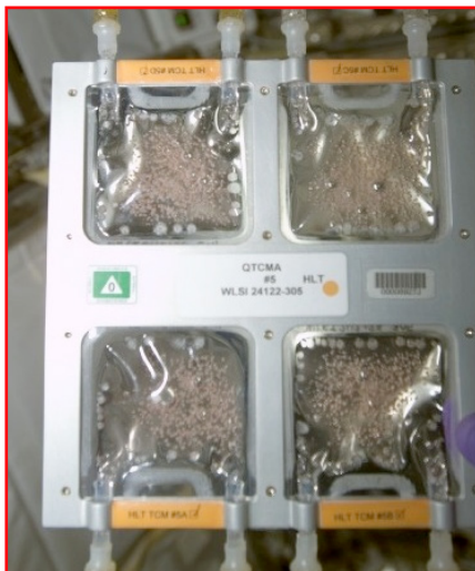
Figure 4: The Biotechnology Specimen Temperature Controller.
