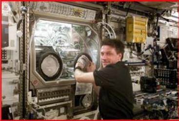
Figure 9. Microgravity Science Glovebox.
