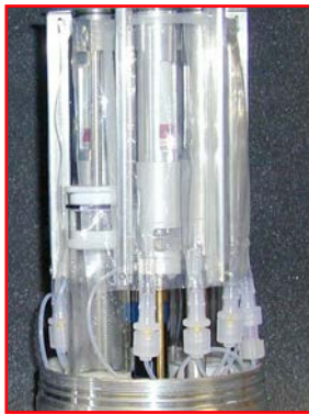
Figure 7. BioServe Culture Apparatus.
