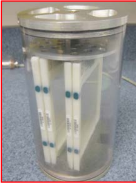
Figure 6. OptiGAP (left) and Gas Exchange - Group Activation Packs (right).
