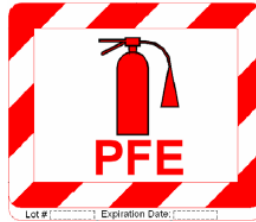
FIGURE 4.13.2.2.2.1-4 ISS PORTABLE FIRE EXTINGUISHER PANEL DOOR LABELS (SDG32107729)
