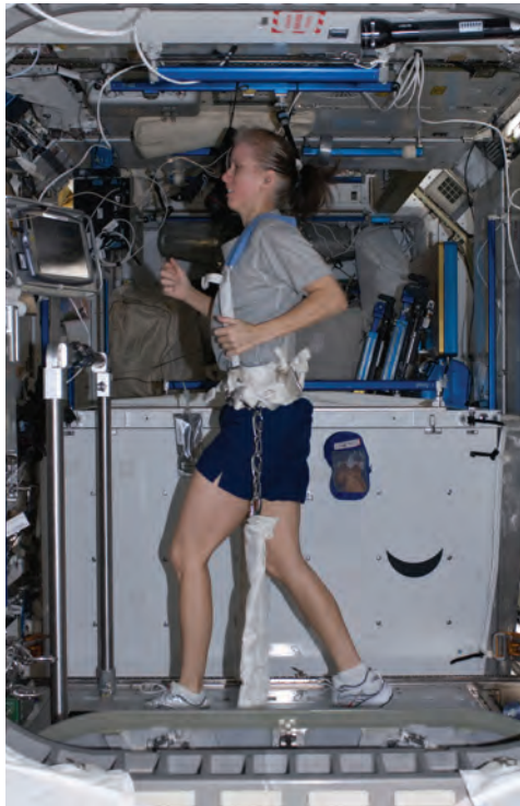
Figure 53. NASA astronaut Shannon Walker, equipped with a bungee harness, exercises on the Combined Operational Load Bearing External Resistance Treadmill (COLBERT) in Node 3 of the ISS. Photo Credit: NASA.
