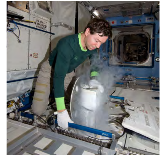
Figure 82. NASA astronaut Mike Barratt puts samples in the MELFI, which is typically maintained at -96°C. Photo Credit: NASA.
