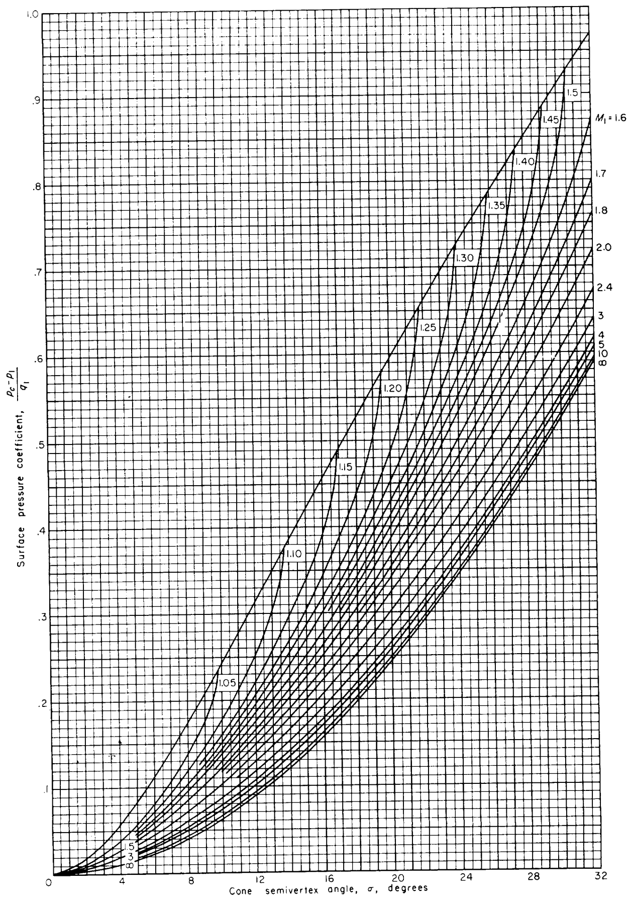
CHART 6.--Variation of surface pressure coefficient with cone semivertex angle for various upstream Mach numbers. Perfect gas, \gamma = 1.405 .
