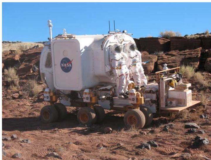
Figure 8. Prototype pressurized lunar rover with exterior-mounted spacesuits.
