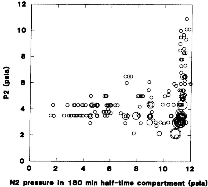
Fig. 1. The circles are 258 tests on a P2 vs. PIN<sub>2</sub> plot. The PIN<sub>2</sub> for each test was calculated using Eq. 1 with t<sub>1/2</sub> = 180 min to account for denitrogenation before ascent to P2. The area of each circle represents the incidence of serious DCS observed during the test. Most of the large circles appear in the lower right corner where limited denitrogenation occurred before ascent and where the test altitudes were between 2.0 and 5.0 psia.
