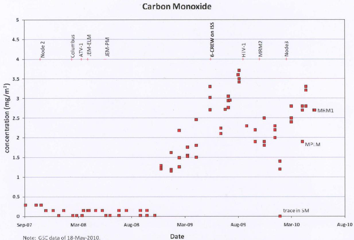
**Carbon Monoxide Accumulation aboard ISS:** From late 2008 the nominal concentrations of CO had been increasing gradually (see figure above). The results from samples returned on this flight indicate that the CO concentrations, after dropping in late 2009, have cycled upward. In any case, these changes are well below the 180-day SMAC for CO, which is 17 mg/m<sup>3</sup>. There is no threat to crew health. The source of the additional CO is unknown.
