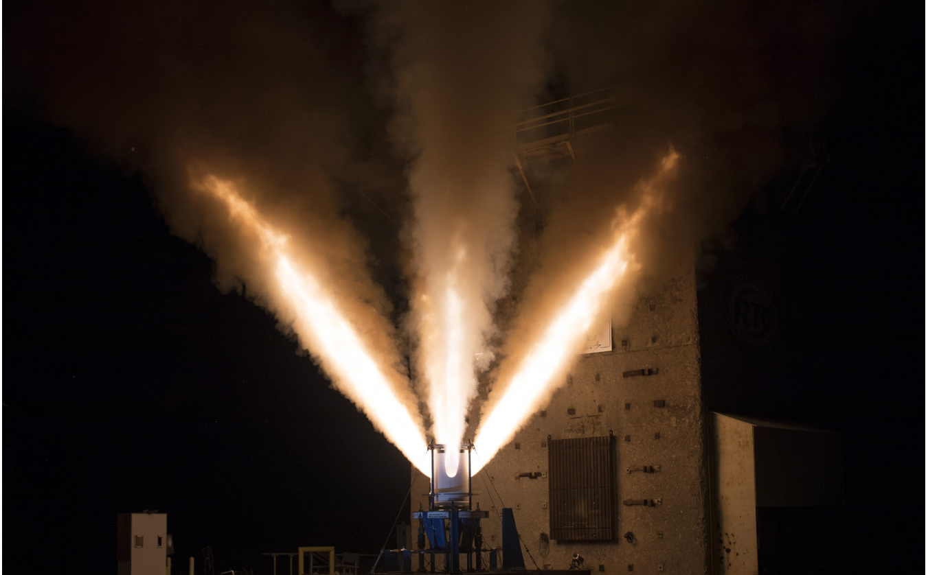
▲ Aerojet Rocketdynes completes a demonstration test on Aug. 28, 2019, with the first jettison motor for the Orion spacecraft’s launch abort system that utilized Aerojet’s Orange, Virginia facility for propellant mixing and loading and motor final assembly.
