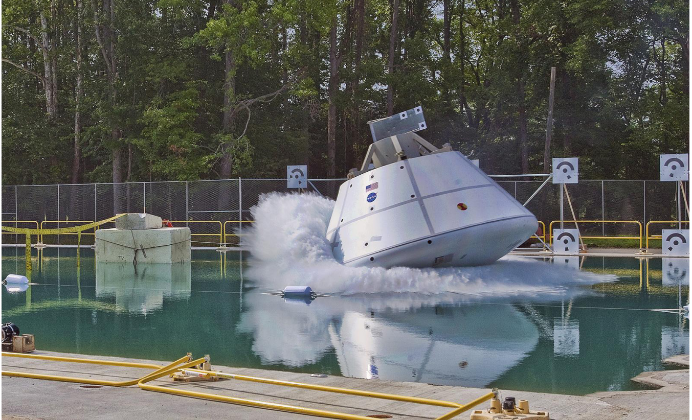
▲ An Orion boilerplate test article (BTA) drop test takes place at the Hydro Impact Basin at the Landing and Impact Research Facility at NASA's Langley Research Center on July 21, 2011.
