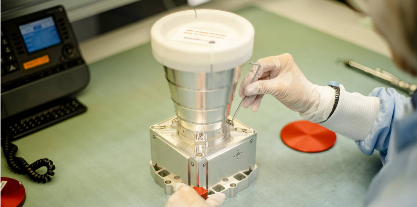
▲ A Jena-Optronik technician in Jena, Germany, works on a star tracker, a sensitive camera that will take pictures of the star field around the Orion spacecraft. By comparing the pictures to its built-in map of stars, the star tracker can determine which way Orion is oriented.
