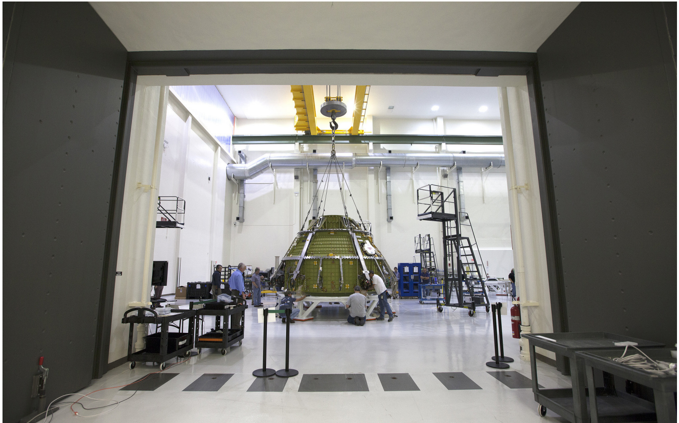
▲ Lockheed Martin engineers and technicians prepare the Orion pressure vessel for a series of tests inside the proof pressure cell in the Neil Armstrong Operations and Checkout Building at NASA's Kennedy Space Center in Florida.
