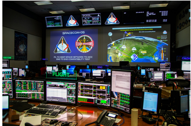
▲ Teams perform communication testing between NASA's Mission Control Center in Houston and a lab at Orion prime contractor Lockheed Martin's facility near Denver that replicates Orion's computer, wiring and avionics systems configurations.
