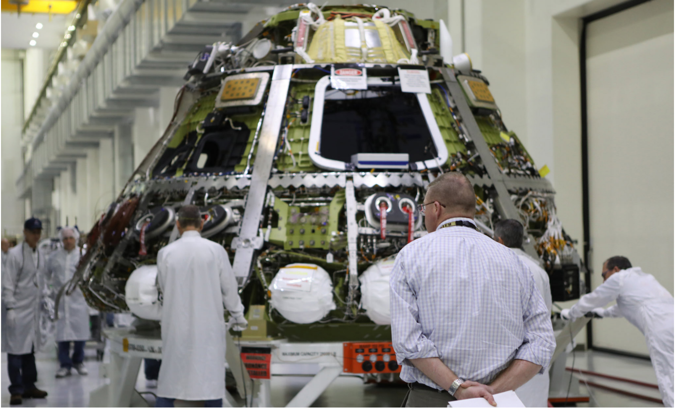
▲ Technicians assist as the Orion crew module for Artemis I is moved toward the thermal chamber in the Neil Armstrong Operations and Checkout Building high bay at NASA's Kennedy Space Center in Florida.
