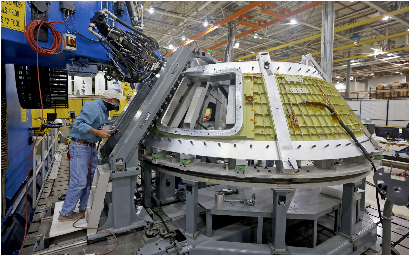
▲ At NASA's Michoud Assembly Facility in New Orleans, technicians from Orion prime contractor Lockheed Martin weld together three cone-shaped panels on Orion's crew module for the Artemis III mission that will land the first woman and next man on the Moon.
