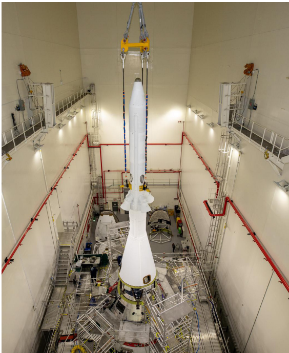
◀ Teams with NASA's Exploration Ground Systems (EGS) and contractor Jacobs integrate the launch abort system (LAS) with the Orion spacecraft inside the Launch Abort System Facility at NASA's Kennedy Space Center in Florida on July 23, 2021.
