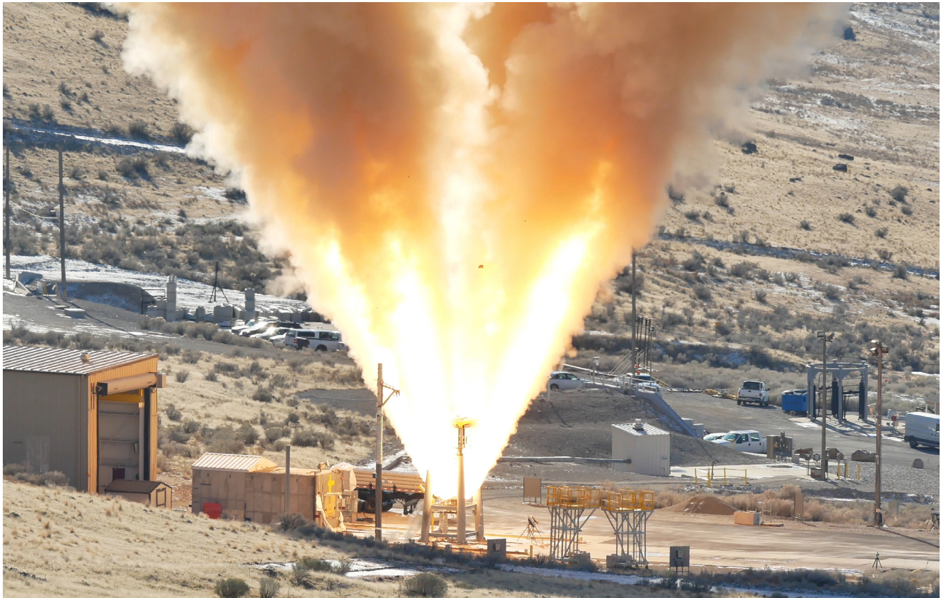
▼ NASA, Northrop Grumman, and Lockheed Martin successfully perform a ground firing static test of the abort motor for the Orion spacecraft launch abort system at Northrop’s facility in Promontory, Utah, on Dec. 13, 2018.
