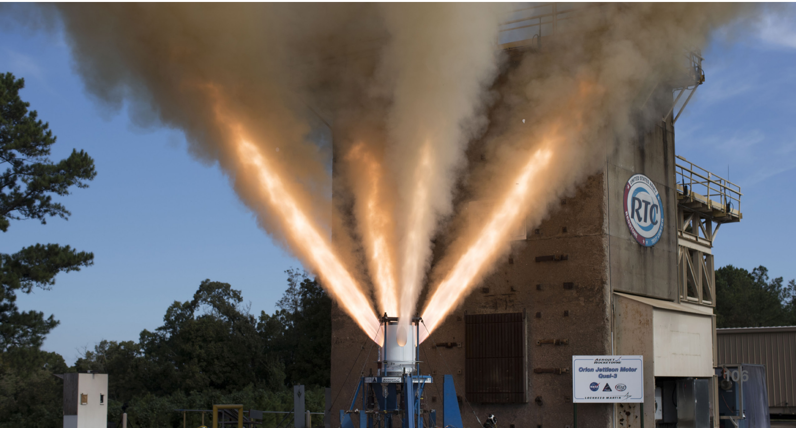
▼ Engineers perform a hot-fire test of the jettison motor for the Orion spacecraft’s launch abort system at the U.S. Army Redstone Test Center on Redstone Arsenal in Huntsville, Alabama on Feb. 25, 2020.
