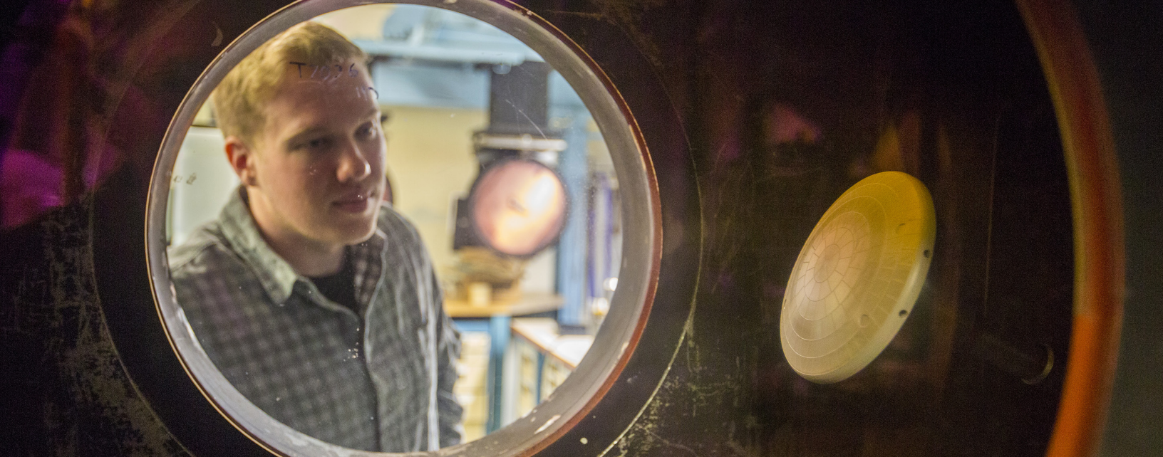
▲ Testing at NASA's Langley Research Center in Hampton, Virginia takes place to investigate the heating of the Orion spacecraft during reentry into Earth's atmosphere with a 6-inch Orion heat shield model in the 20-inch Mach 6 wind tunnel.
