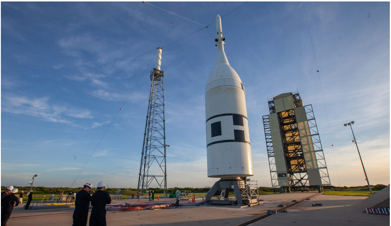
▼ The Ascent Abort-2 test vehicle is secured on the pad at Launch Complex 46 at Cape Canaveral Air Force Station in Florida after rollback of the Vertical Integration Facility on July 1, 2019.
