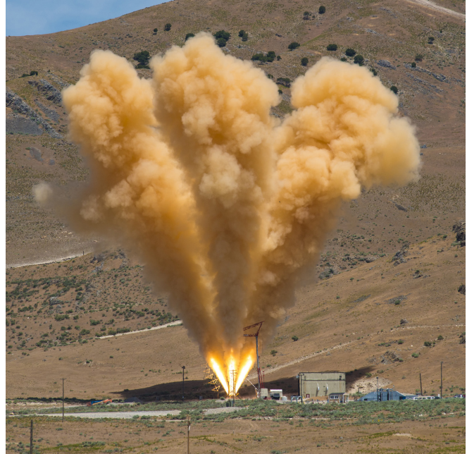
▲ Engineers successfully perform a ground firing static test of the abort motor for the Orion spacecraft launch abort system at Northrop Grumman facility in Promontory, Utah, on June 15, 2017.
