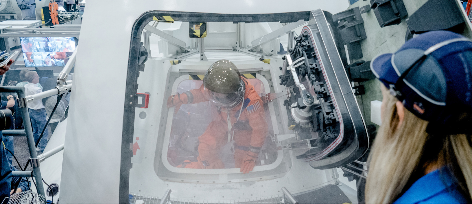
▲ During testing using the Orion mockup in the Space Vehicle Mockup Facility at NASA's Johnson Space Center in Houston, engineers use fake smoke to imitate a scenario in which astronauts must exit the capsule when their vision is obscured.
