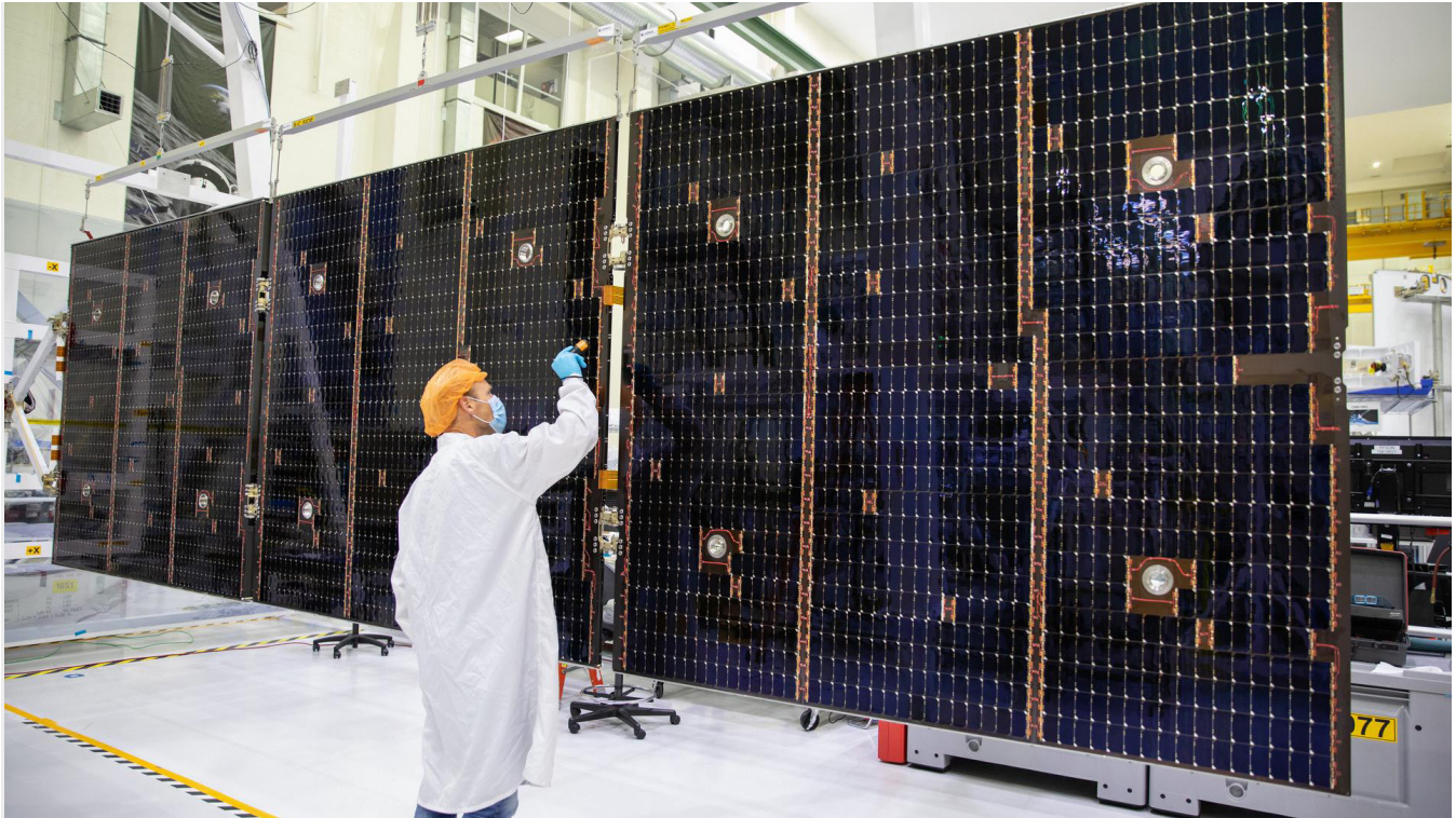
▲ In preparation for installation on the Artemis I spacecraft, technicians extend one of the Artemis I solar array wings for inspection inside the Neil Armstrong Operations and Checkout Building high bay at NASA's Kennedy Space Center in Florida on Sept. 10, 2020, to confirm that it unfurled properly and all of the mechanisms functioned as expected.
