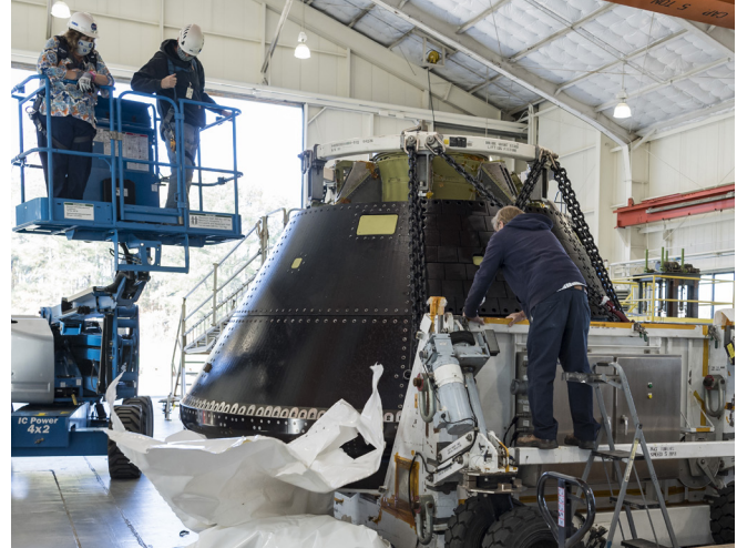
▲ On Dec. 2, 2020, researchers at NASA’s Langley Research Center unwrap Orion’s structural test article to be used in a series of water impact tests that will prepare the final computer modeling for loads and structures prior to Artemis II.
