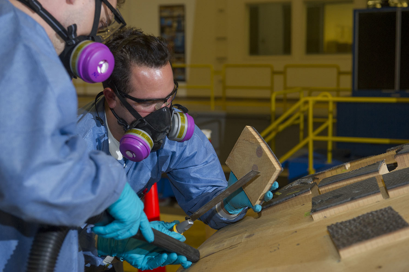
▲ Engineers from Ames Research Center and Marshall Space Flight Center remove samples from the Orion heat shield that flew on Exploration Flight Test-1 in 2014. The heat shield protected the spacecraft from temperatures reaching 4,000 degrees Fahrenheit.
