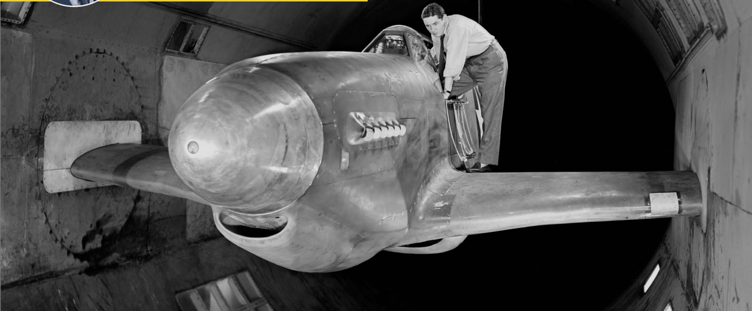
↑ Testing of a North American XP-51B Mustang with cropped wings in the Ames Laboratory's 16-Foot High-Speed Tunnel. Researchers were able to trace the source of a serious rumble to the plane's air scoop below the fuselage. (Photo credit: NACA)
