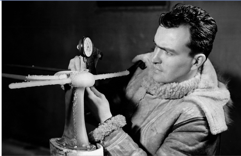
↑ An NACA researcher measures the ice thickness on a landing antenna model in the Icing Research Tunnel at the Aircraft Engine Research Laboratory in Cleveland, Ohio. (Photo credit: NACA)
