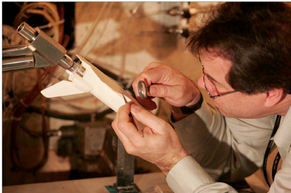
↑ A bit of precisely sized and shaped tape is placed on the surface of a wind tunnel model for studies of aerodynamic heating during Shuttle reentry, simulating the effects of an on-orbit "plug" repair. (Photo credit: NASA/LaRC)
