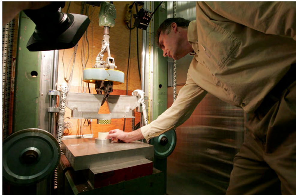
↑ A researcher places a sample of foam like that on the Shuttle External (fuel) Tank into a crushing device to determine how the foam reacts when it strikes something at high speed, as happened during the Columbia mission. (Photo credit: NASA/LaRC)
