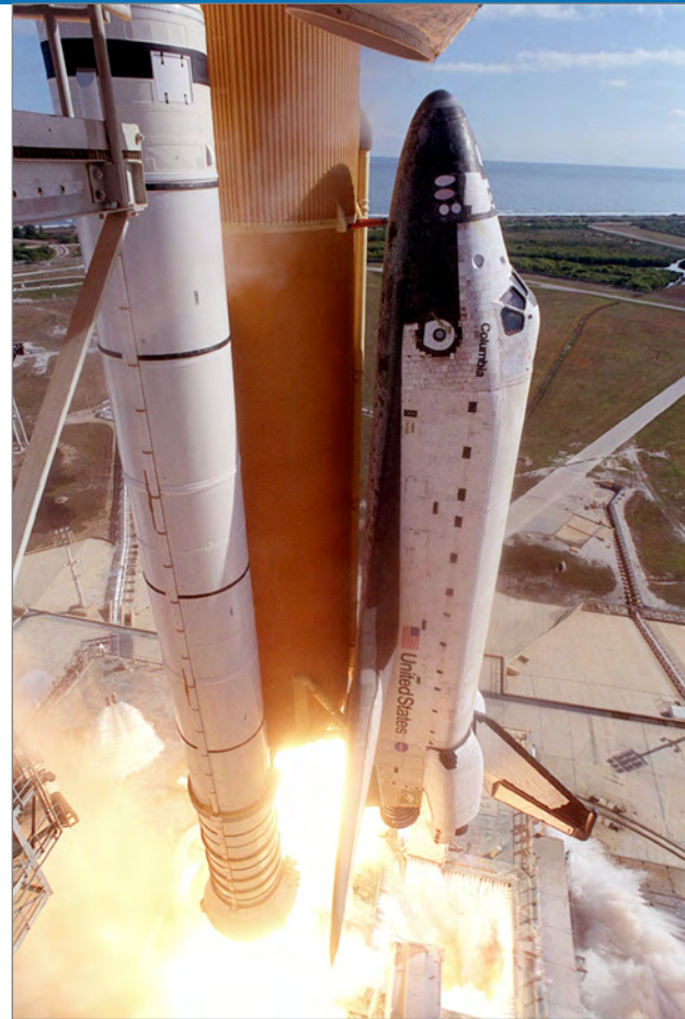
↑ This close-up shows Space Shuttle Columbia as it lifted off from Launch Pad 39A on mission STS-107 on 16 January 2003. A piece of insulative foam from the External Tank struck the leading edge of the left wing (shown here) upon liftoff, leading to the loss of the vehicle and its crew on reentry on 1 February. (Photo credit: NASA)
