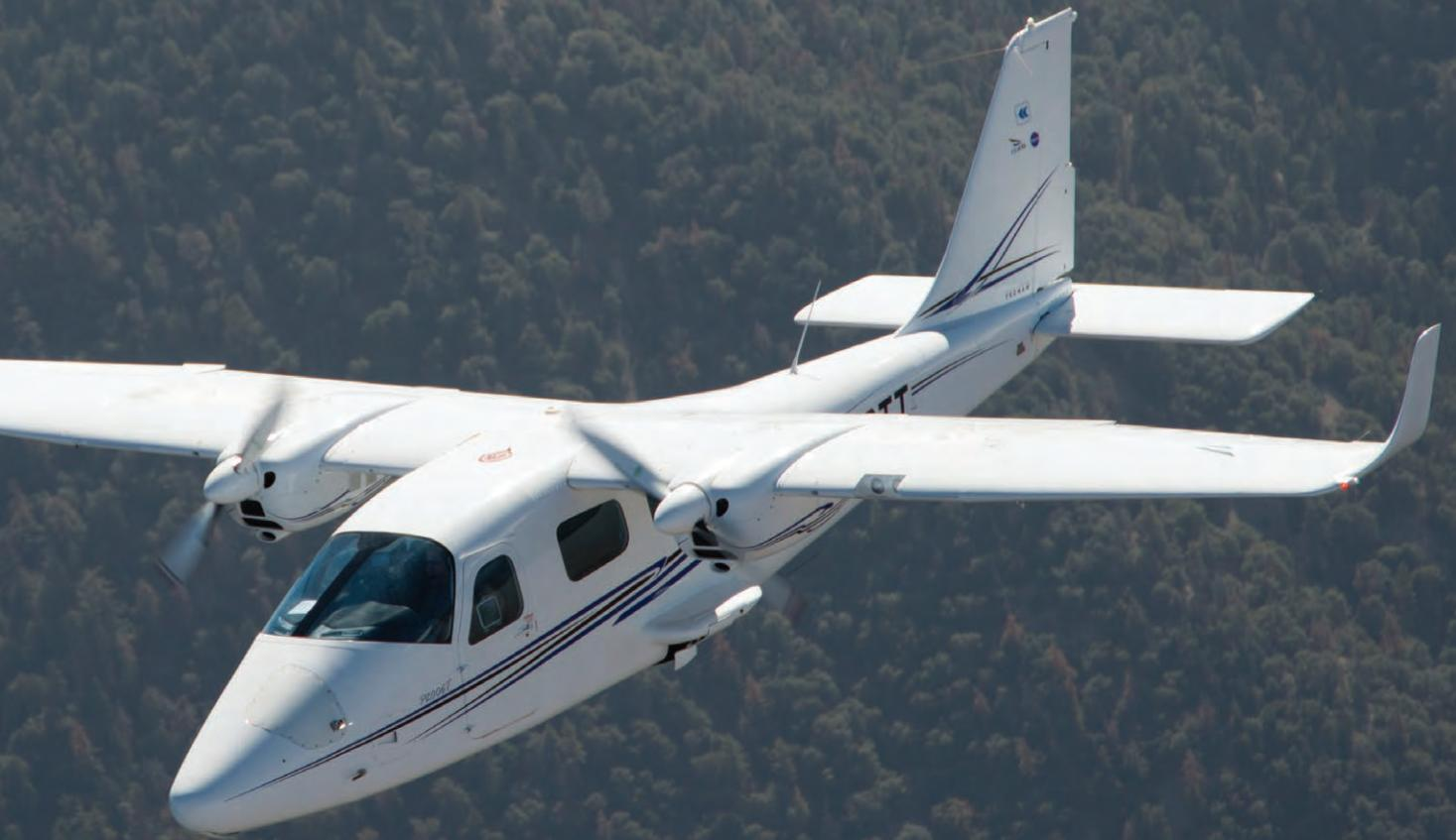
This Tecnam aircraft is part of an X-Plane demonstrator project. It will be modified to evaluate electric propulsion technologies.
