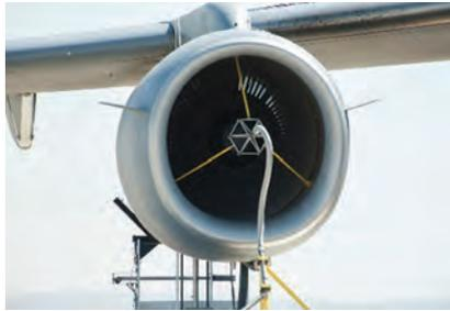
A major aspect of NASA's propulsion health management development work is demonstrating and evaluating emerging technologies on operational engines. Harsh environment conditions within an engine present significant challenges for the integration and application of aircraft health management technologies. VIPR is a program for developing real-world tests to evaluate such emerging technologies.
