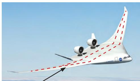
Installed strain sensors
