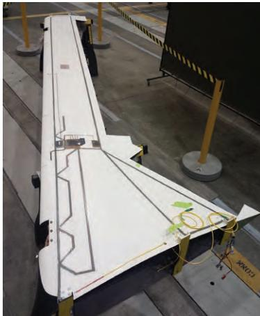
**Work to date:** The team has validated the controller for both flutter suppression and shape control in simulations using X-56A models that contain all six rigid-body degrees of freedom, flexible modes, 10 control surfaces, and actuators. Simulations have shown that the shape controller can affect the global angle of attack and achieve drag changes. The fiber optic sensors have been installed on the flexible wings of the X-56A.
