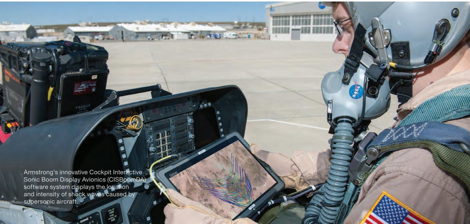
Armstrong's innovative Cockpit Interactive Sonic Boom Display Avionics (CISBooMDA) software system displays the location and intensity of shock waves caused by supersonic aircraft.
