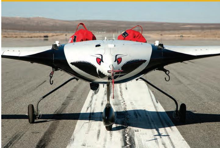
Armstrong engineers continue to pioneer new research in aircraft design and modeling. Researchers are experimenting with revolutionary hyperelastic wing control technologies that can reduce weight, improve aircraft aerodynamic efficiency, and suppress flutter. Other cutting-edge research involves techniques, models, and analysis tools for flutter suppression and gust-load alleviation.
