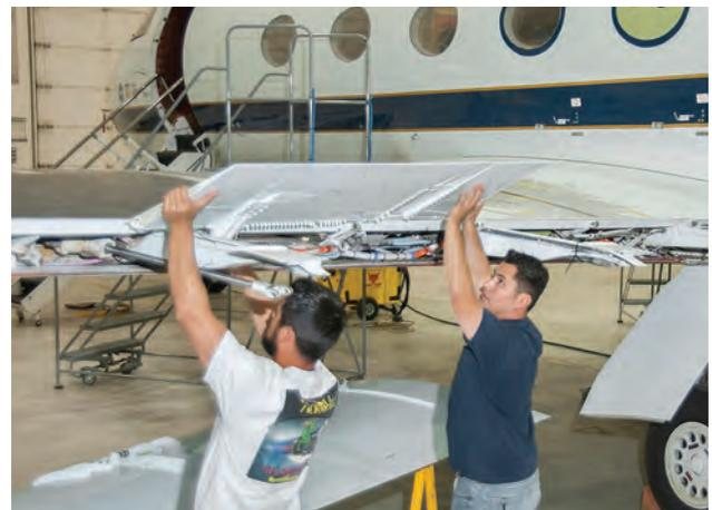
NASA aircraft technicians work on installation of test instrumentation for the ACTE flap on NASA's modified G-III testbed.
