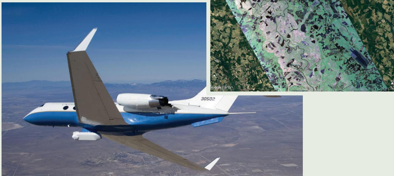
The C-20A is equipped with NASA's Jet Propulsion Laboratory's UAV synthetic aperture radar (UAVSAR) and an Armstrong-developed precision autopilot. In 2022, flights will support study of earthquakes' fault zones, volcanoes, wetlands, and glaciers, and the aircraft will be ready to respond to emergencies related to oil spills, wildfires, floods, and more.
