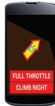
NASA Armstrong's iGCAS can be used for a variety of aircraft, including general aviation, helicopters, and unmanned aircraft. The technology has been incorporated into an application for tablets and other handheld/mobile devices.
