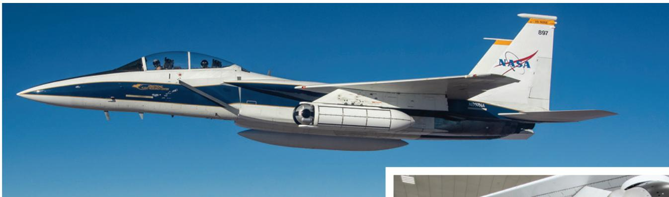
(Above) F-15D TN 897 with new wing store (STA 2) during a compatibility flight profile flight in 2020; (below) GVT and FEM mode shape comparisons of F-15 wing pylon and new wing store; and (right) lateral impact hammer excitation on wing store during GVT
