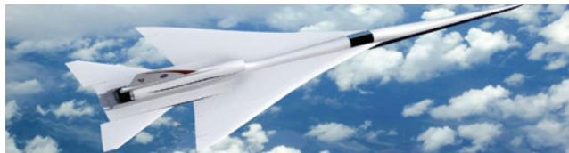
Innovators at NASA Armstrong are developing guidelines and evaluating stability and control characteristics for the planned supersonic Low-Boom Flight Demonstration mission. In addition to stability and control evaluations, Armstrong researchers are developing a supersonic autopilot to control aircraft parameters, such as the flight path and changes in Mach speeds to prevent coalescence of shock waves and minimize perceived sonic boom noise levels on the ground.
