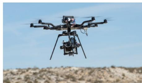
The Resilient Autonomy project team conducted basic functional flight tests of the EVAA-modified HQ-90, a vertical lift and transition remotely piloted aircraft.
