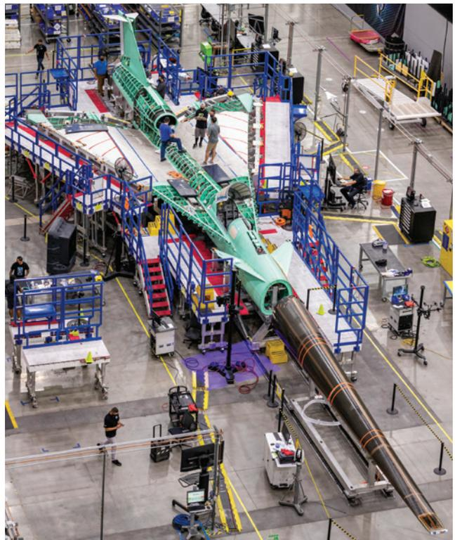
Construction and assembly of the supersonic X-59 QueSST research plane at Lockheed Martin Aeronautics Company's Skunk Works® factory
