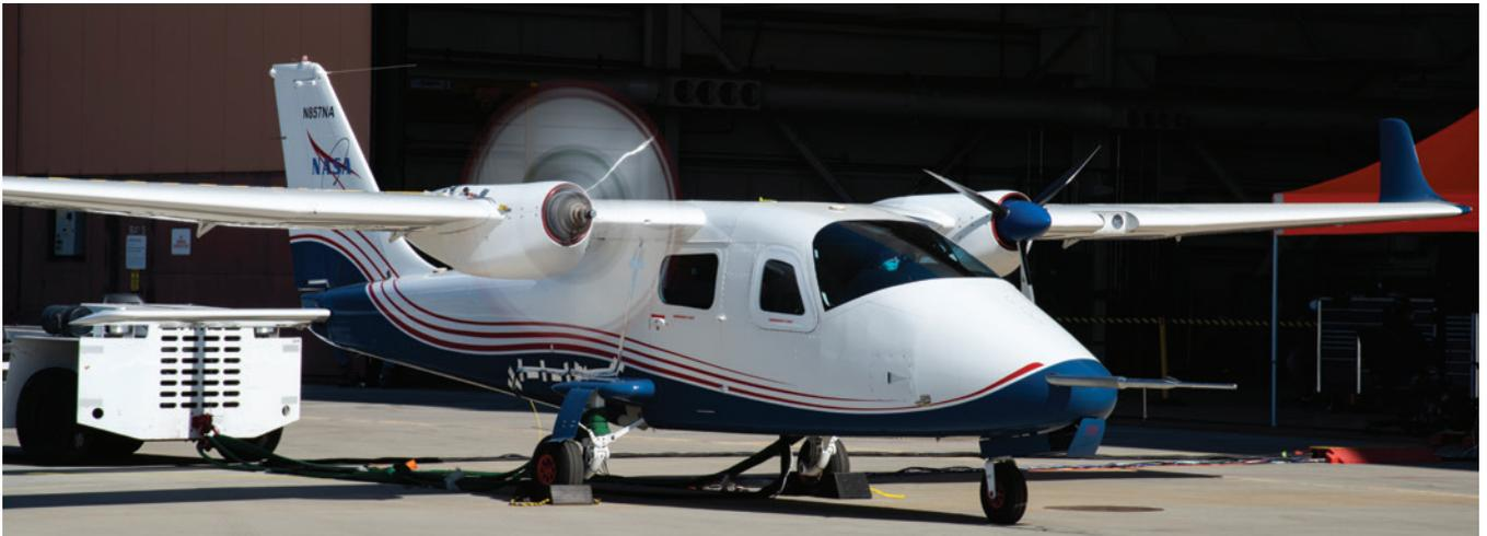
The X-57 aircraft undergoes high-voltage ground testing. Principle goals of the X-57 project are to share the design and airworthiness process with regulatory and standards organizations and establish the aircraft as a reference platform.
