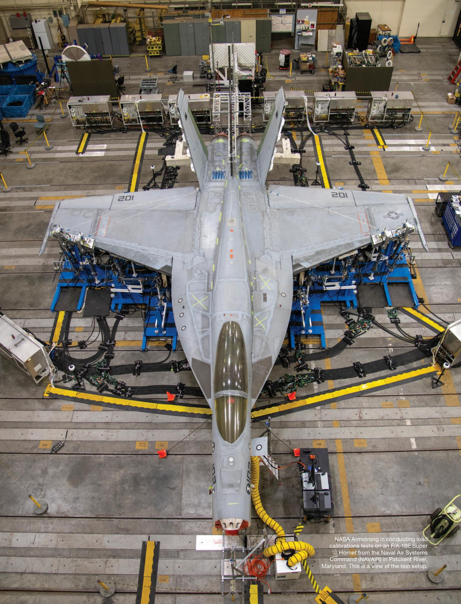
NASA Armstrong is conducting load calibrations tests on an F/A-18E Super Hornet from the Naval Air Systems Command (NAVAIR) in Patuxent River, Maryland. This is a view of the test setup.
