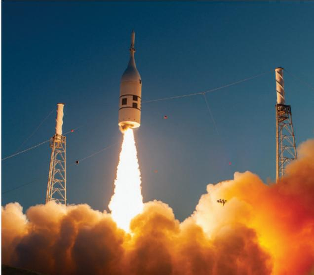
NASA Armstrong researchers developed several systems designed to test the launch abort system (LAS) that will pull astronauts to safety during a launch emergency. The three-minute test, called Ascent Abort-2 (AA-2) occurred in July 2019, and was an important safety milestone in the agency's preparation for crewed flights of the Orion vehicle.
