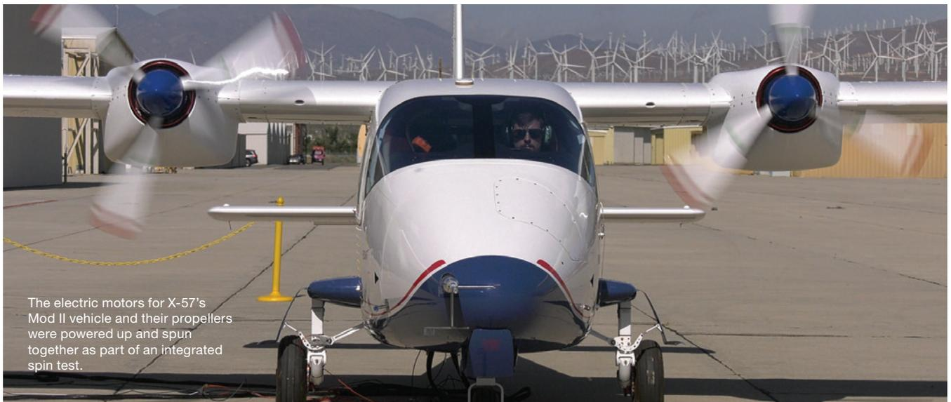
The electric motors for X-57's Mod II vehicle and their propellers were powered up and spun together as part of an integrated spin test.
