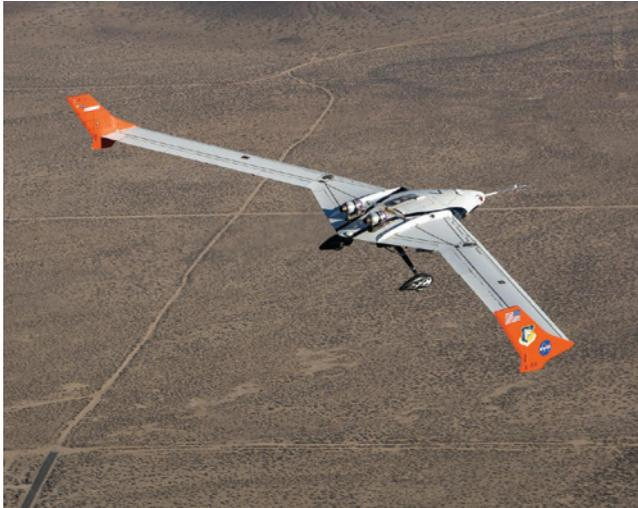
This research effort is developing flight control systems and mathematical models that integrate structural and flight dynamics. As modern aircraft become more flexible and these disciplines converge, conflicts arise between independently developed modeling methodologies. Because the structural and flight dynamics of the X-56A Multi-Utility Technology Testbed (MUTT) aircraft are acutely coupled, resulting models can capture the requirements of both disciplines.
