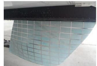
Foam mock-up of the CATNLF test article fabricated by Armstrong's Model Shop
