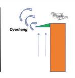
Simplified, preliminary 2D concepts of wind flows near unmodified and modified structures. Potential wind moderators include baffles/wind screens, canvas/mesh scaffold sheeting, and real/artificial vegetation.
