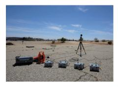
A sonic boom test with THOR and BURST systems, which use data transmitted from supersonic aircraft and satellites to a ground recording system.
