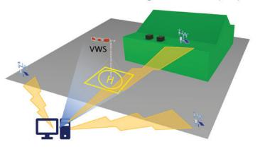
Real-time machine-learning estimations using several networked surrounding weather measurements create a virtual windsock within the TLOF
