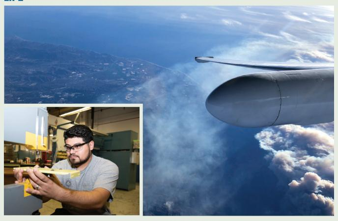
The ER-2 high-altitude aircraft collects data that helps researchers understand the world's ecosystems and provides critical information on natural disasters. Sophisticated imaging technologies enable it to study environmental impacts caused by wildfires.
