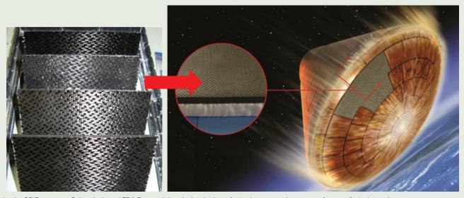
Under the SBIR program, Colorado-based TDA Research Inc., is developing a faster, less expensive process for manufacturing carbon fiber–carbon matrix composites needed for hot structures in a variety of aerospace propulsion systems. Credit: TDA Research Inc.
