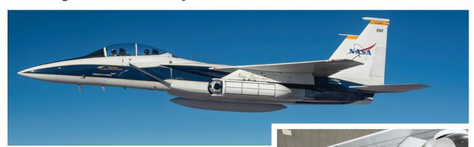
(Above) F-15D TN 897 with new wing store (STA 2) during a compatibility flight profile flight in 2020; (below) GVT and FEM mode shape comparisons of F-15 wing pylon and new wing store; and (right) lateral impact hammer excitation on wing store during GVT
