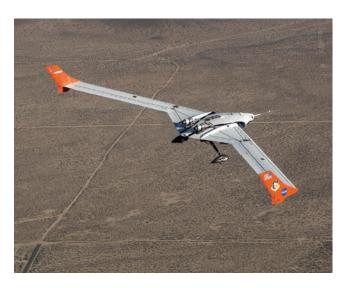
This research effort is developing flight control systems and mathematical models that integrate structural and flight dynamics. As modern aircraft become more flexible and these disciplines converge, conflicts arise between independently developed modeling methodologies. Because the structural and flight dynamics of the X-56A Multi-Utility Technology Testbed (MUTT) aircraft are acutely coupled, resulting models can capture the requirements of both disciplines.
