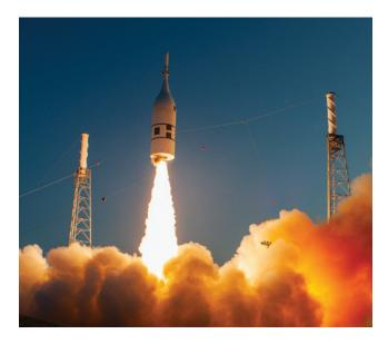
NASA Armstrong researchers developed several systems designed to test the launch abort system (LAS) that will pull astronauts to safety during a launch emergency. The three-minute test, called Ascent Abort-2 (AA-2) occurred in July 2019, and was an important safety milestone in the agency's preparation for crewed flights of the Orion vehicle.
