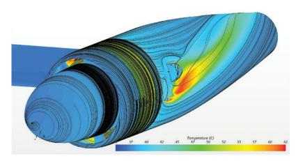
Visualization of the CFD skin temperatures over the X-57 Mod III electric cruise motor nacelle
