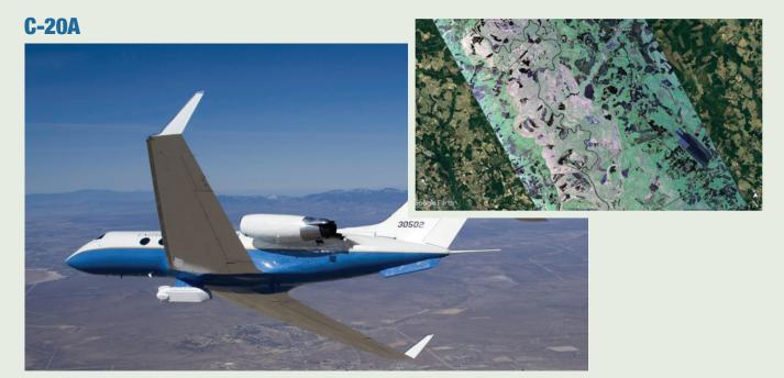
The C-20A is equipped with NASA's Jet Propulsion Laboratory's UAV synthetic aperture radar (UAVSAR) and an Armstrong-developed precision autopilot. In 2022, flights will support study of earthquakes' fault zones, volcanoes, wetlands, and glaciers, and the aircraft will be ready to respond to emergencies related to oil spills, wildfires, floods, and more.
