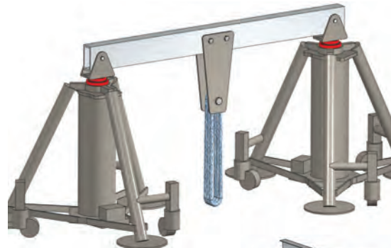
The soft-support system suspended the aircraft by using bungee rings to hold the main landing gear axles.
