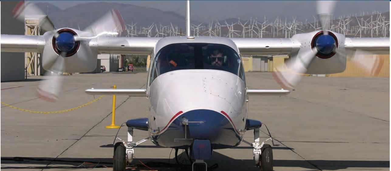
The electric motors for X-57's Mod II vehicle and their propellers were powered up and spun together in an integrated spin test.
