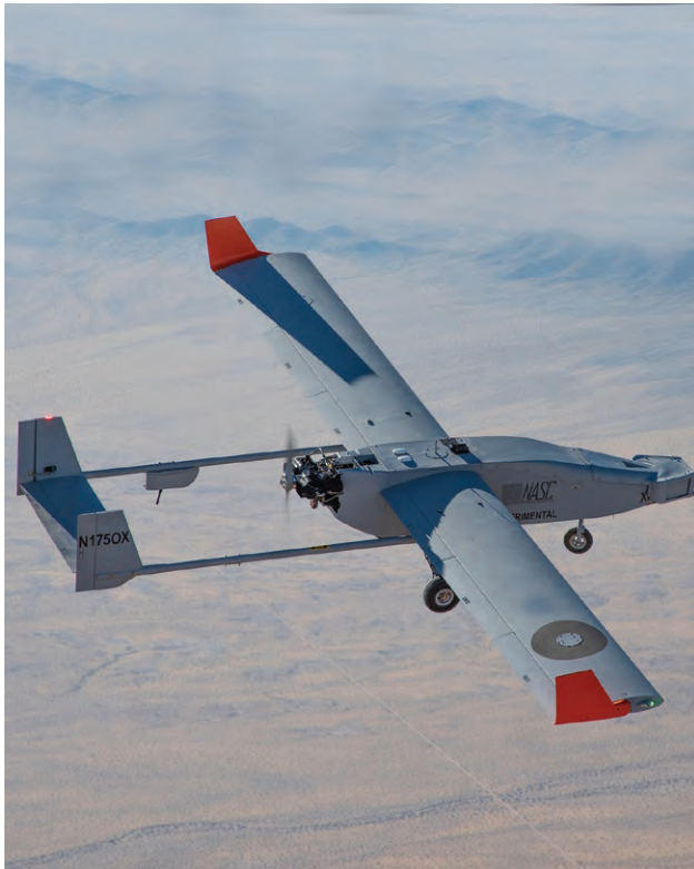
The Navmar Applied Sciences Corporation TigerShark aircraft flew over Edwards Air Force Base in July 2019 during a series of flight tests to support development of DAA standards for medium-sized UAS.
