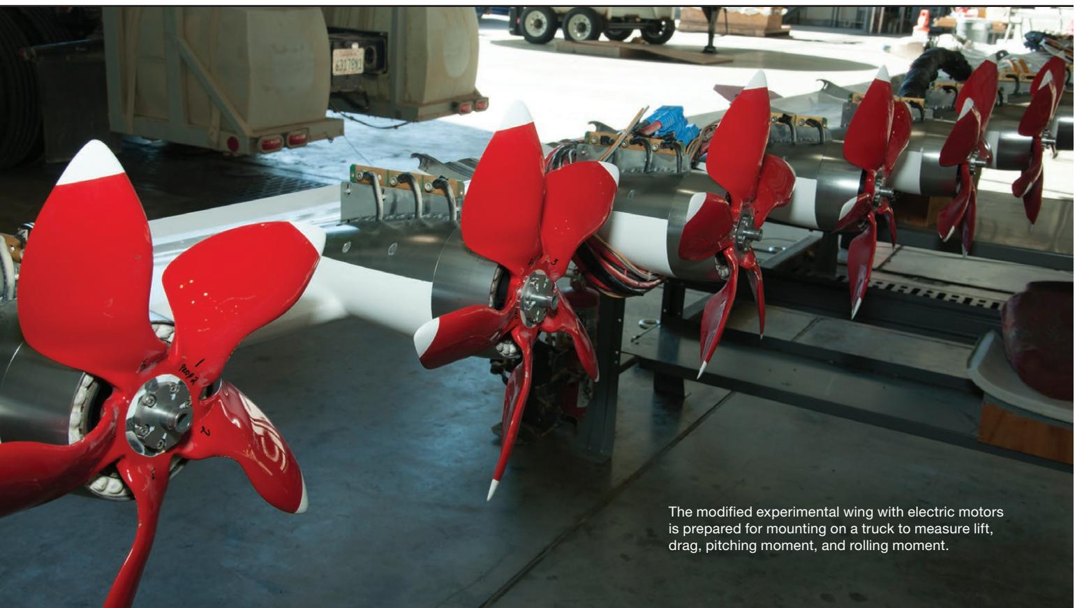
The modified experimental wing with electric motors is prepared for mounting on a truck to measure lift, drag, pitching moment, and rolling moment.
