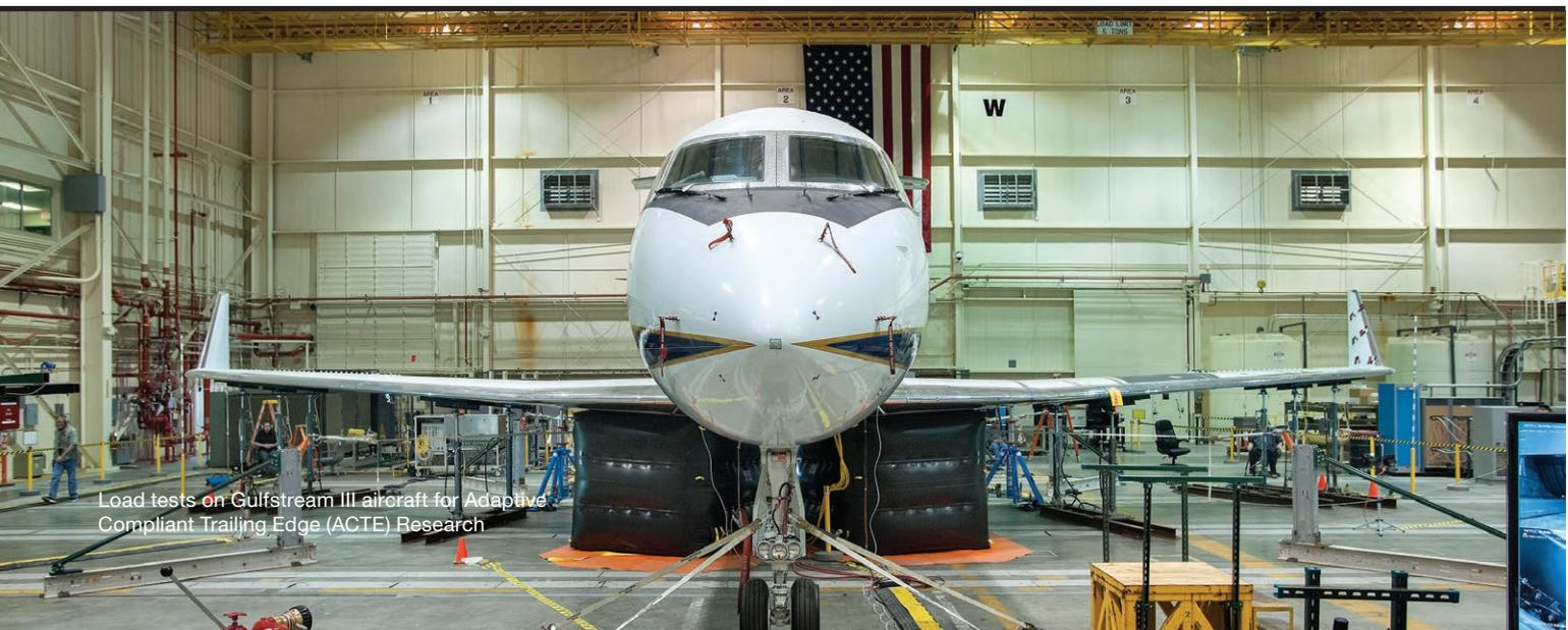
Load tests on Gulfstream III aircraft for Adaptive Compliant Trailing Edge (ACTE) Research
