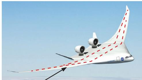
Installed strain sensors
