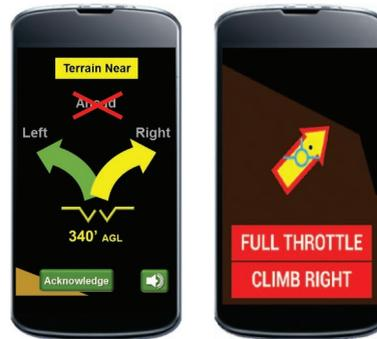
Armstrong's iGCAS can be used for a wide variety of aircraft, including general aviation, helicopters, and UAVs. The technology has been incorporated into an application for tablets and other handheld/mobile devices.
