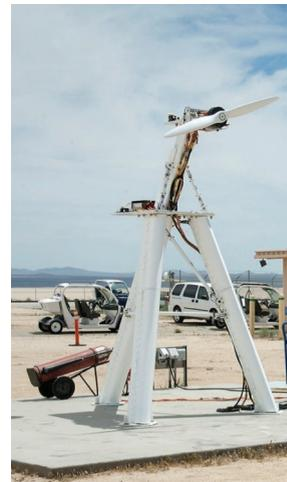
**Work to date:** Researchers have used the Airvolt test stand to gather data from a Joby JM1 motor. Researchers are analyzing the data so that a motor model can be used for a hybrid electric hardware-in-the-loop simulation testbed. Accurate models are required in the simulation to reflect the true hardware configuration and provide an assessment tool for researchers.
