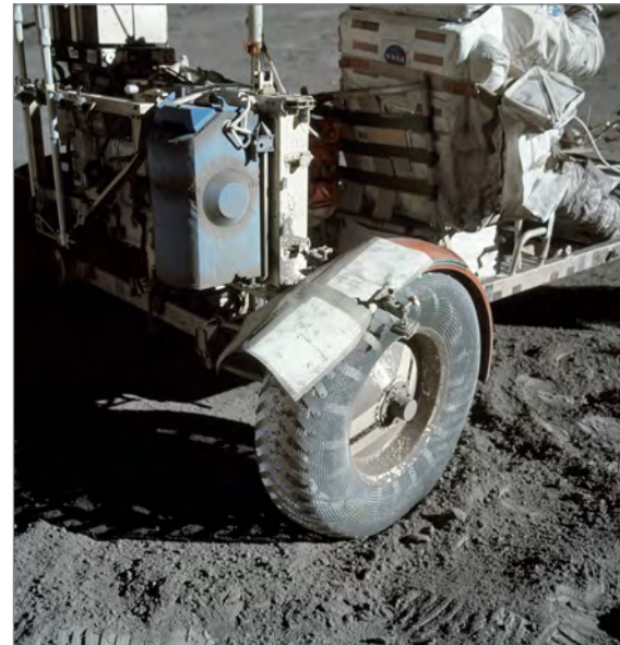
↑ Left: From left to right, John Young, Charlie Duke, Deke Slayton, Rocco Petrone, and Ron Blevins discuss the prototype for the rover replacement fender. Note the lunar maps, tape, and clamps that ultimately held the fender in place for the remainder of the traverses. (Photo credit: NASA) Right: A close-up view of the lunar rover with the final makeshift repair to the right rear fender. Schmitt is seated in the rover. (Photo credit: NASA)
