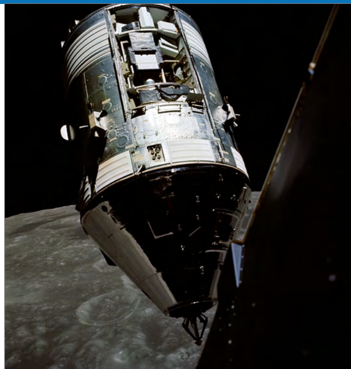
↑ The Apollo 17 Command and Service Modules photographed from the Lunar Module during rendezvous and docking maneuvers in lunar orbit. Note the exposed Scientific Instrument Module Bay, where a lunar sounder, an infrared scanning spectrometer, and a far-ultraviolet spectrometer were housed along with a panoramic camera, mapping camera, and laser altimeter. (Photo credit: NASA)
