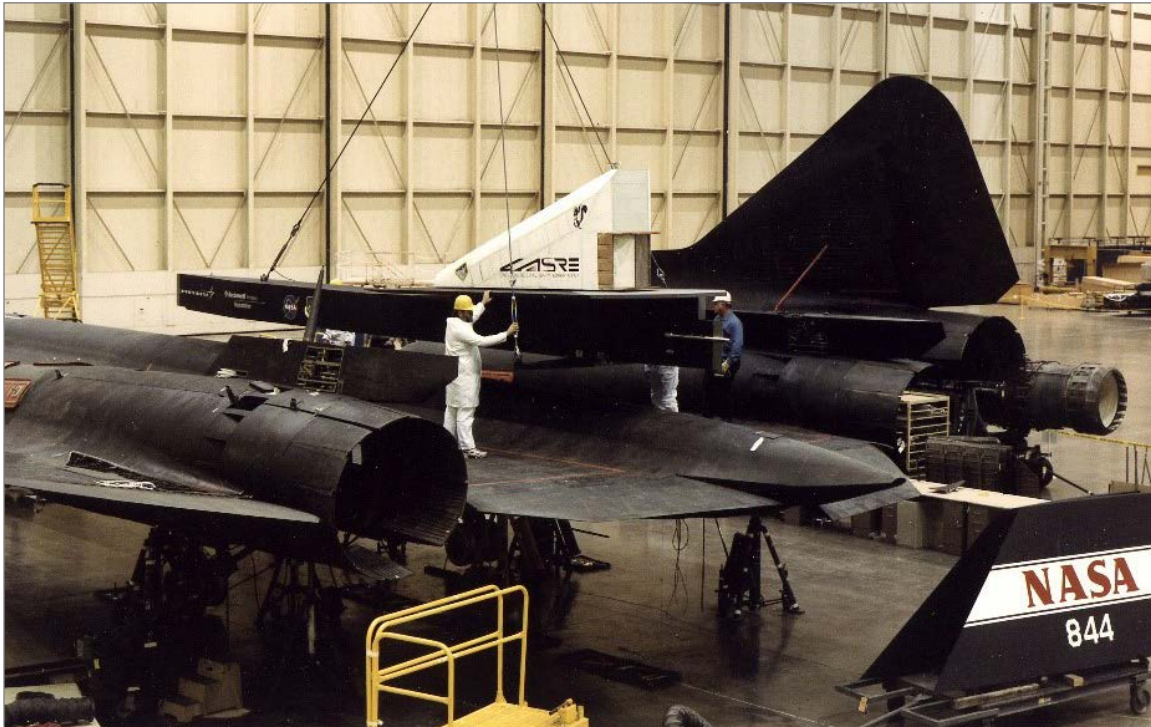
Adding the LASRE pod on the back of the SR-71. (Photo credit: NASA/Tony Landis)
