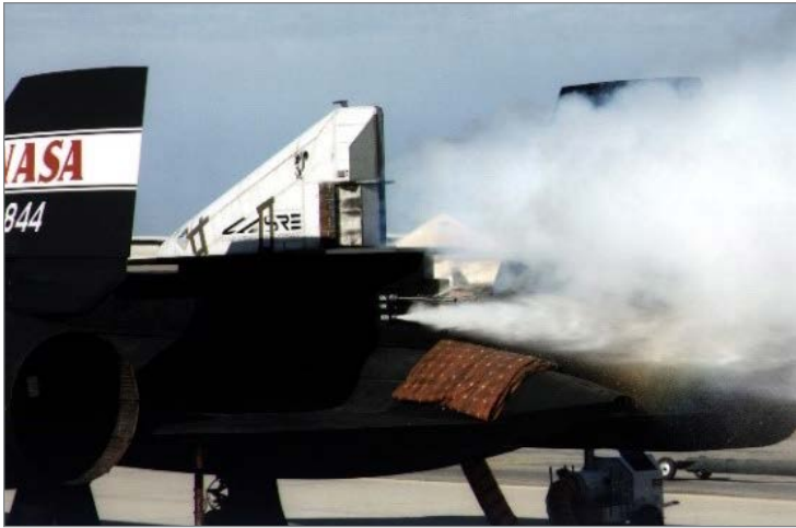
Ground cold flow test of the linear aerospike rocket engine mounted on the rear fuselage of an SR-71. (Photo credit: NASA/Tony Landis)
