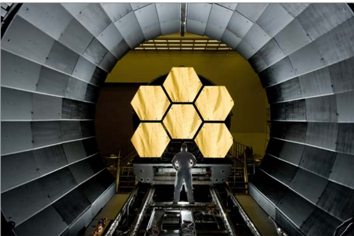
Six gold-coated beryllium primary mirror segments in their test positions in the cryo vacuum chamber at the X-ray and Cryogenic Facility. (Photo credit: NASA/MSFC/David Higginbotham)
