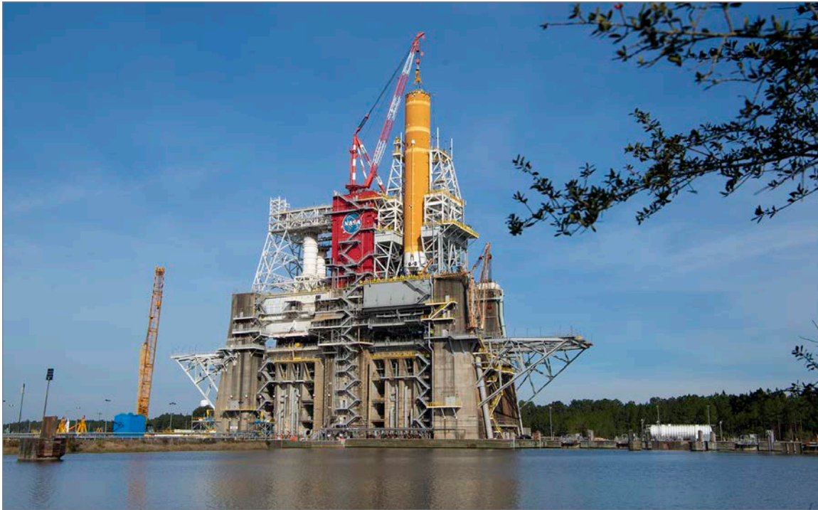
The massive core stage for NASA's Space Launch System (SLS) rocket is in the B-2 Test Stand at NASA's Stennis Space Center near Bay St. Louis, Mississippi, for the core stage Green Run test series. NASA and Boeing, the core stage lead contractor, installed the stage into the test stand in January 2020. The core stage Green Run test series is an important step toward safely launching SLS and NASA's Orion spacecraft beyond Earth's orbit to the Moon for the Agency's Artemis program. The 212-foot-tall rocket stage—the largest stage the Agency has ever produced—contains the cryogenic liquid hydrogen and liquid oxygen tanks that will feed four RS-25 rocket engines, along with the vehicle's avionics and flight computers. The comprehensive test campaign will validate the core stage design and ensure that it is ready for the first and future Artemis missions to the Moon. (Photo credit: NASA)
