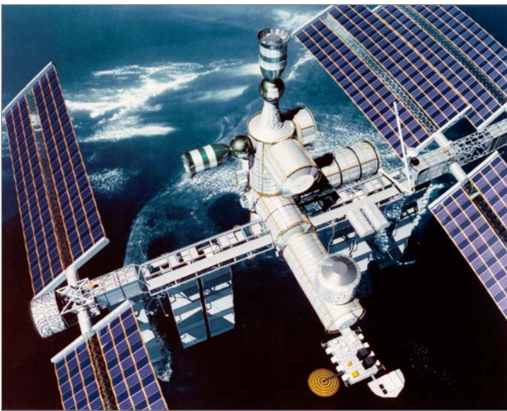
Space Station Freedom option A showing two Soyuz Assured Crew Return Vehicle (ACRV) capsules docked at berthing ports. (Image credit: NASA)
