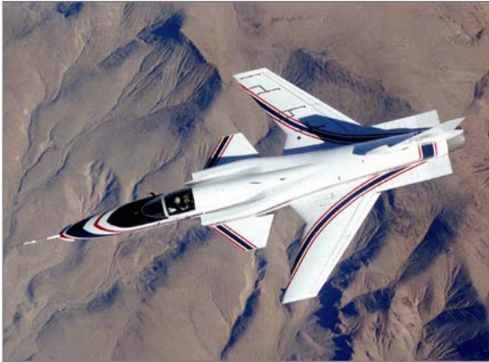
The Grumman X-29 experimental fighter aircraft in flight over California's Mojave Desert in 1985. (Photo credit: NASA)
